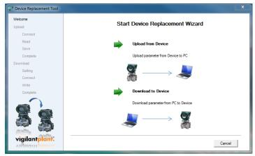
The main menu page for the Device Replacement Tool is displayed. It will step through the upload and download procedure.
