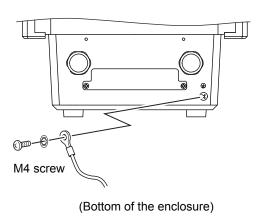
**Wiring Procedure for Grounding Terminals**
