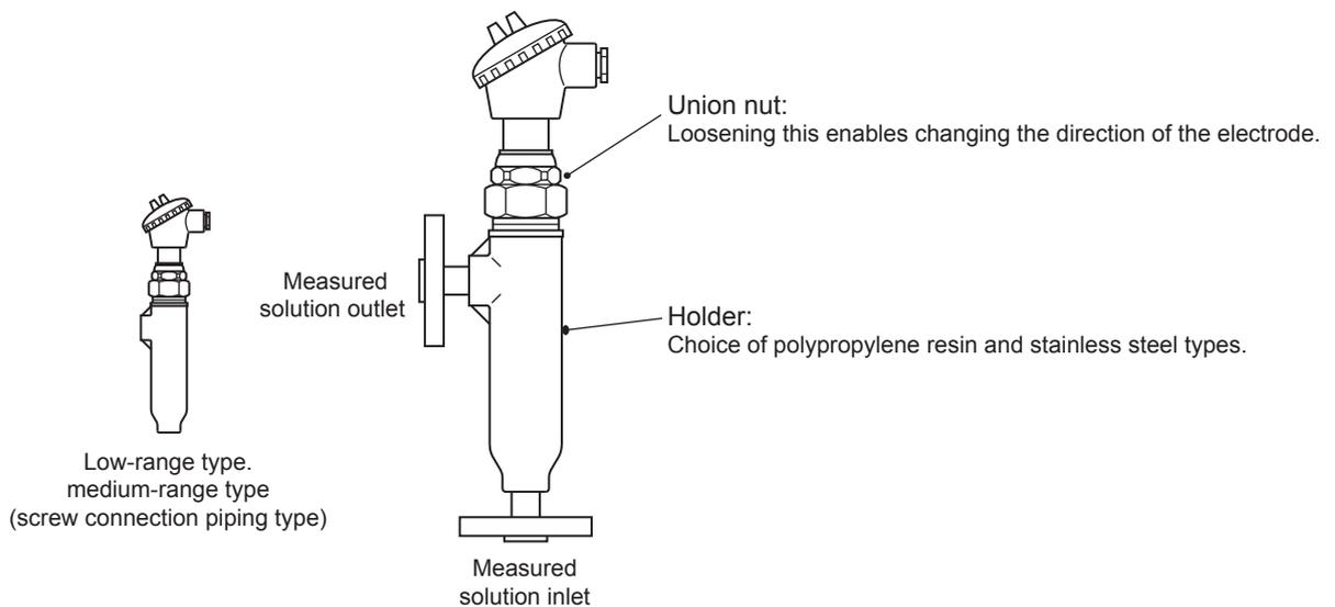
Figure 2.1 Conductivity Detector
