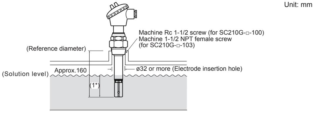
\*1: Always keep the electrode tip dipped more than 60 mm for SC210G-A, more than 100 mm for SC210G-B.
