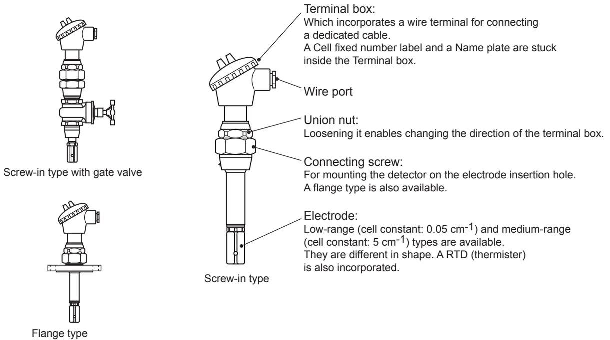
• Flow-through type conductivity detector
