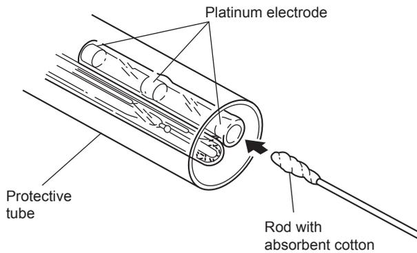
Figure 5.1 Cleaning an Electrode with a 5 cm<sup>-1</sup> Cell Constant
