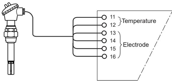
SC210G Conductivity Detector (two-electrode system)
