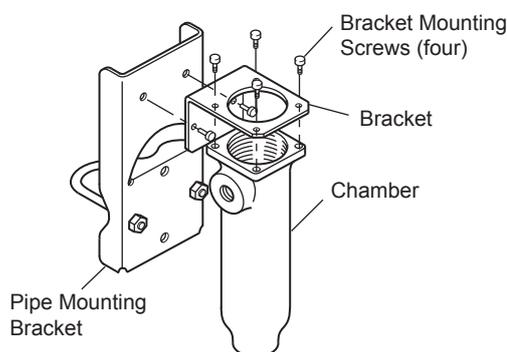
**Figure 3.6** Bracket for Fixing the Polypropylene Resin Holder
