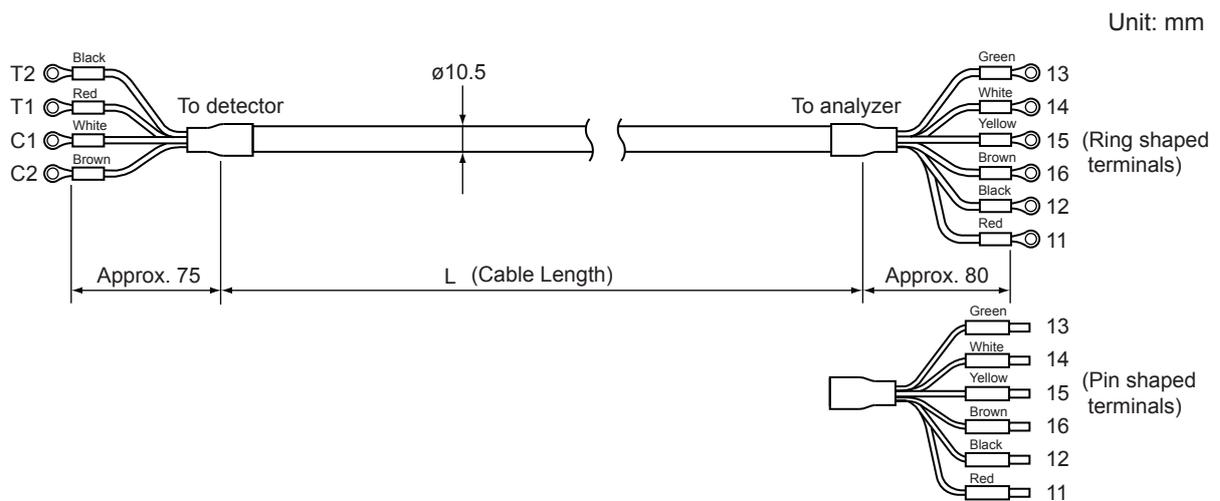
Figure 3.8 Detector Cable
