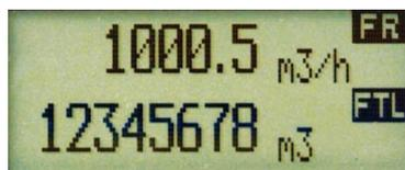
3 Lines (Flow Rate, Flow Total and Bar graph)
