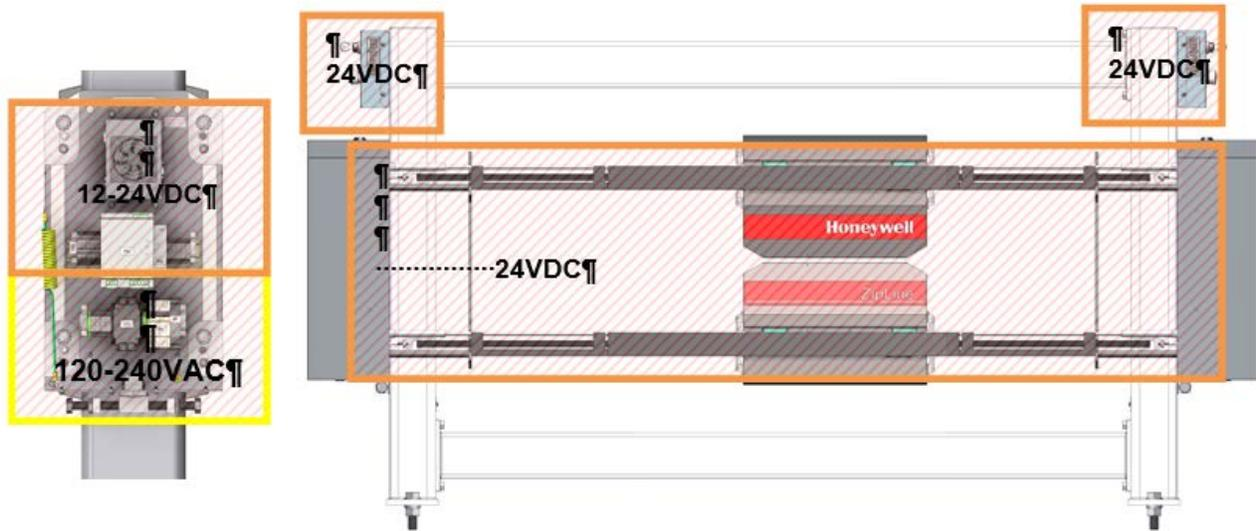
Figure 2-5: Scanner Voltage Zones
