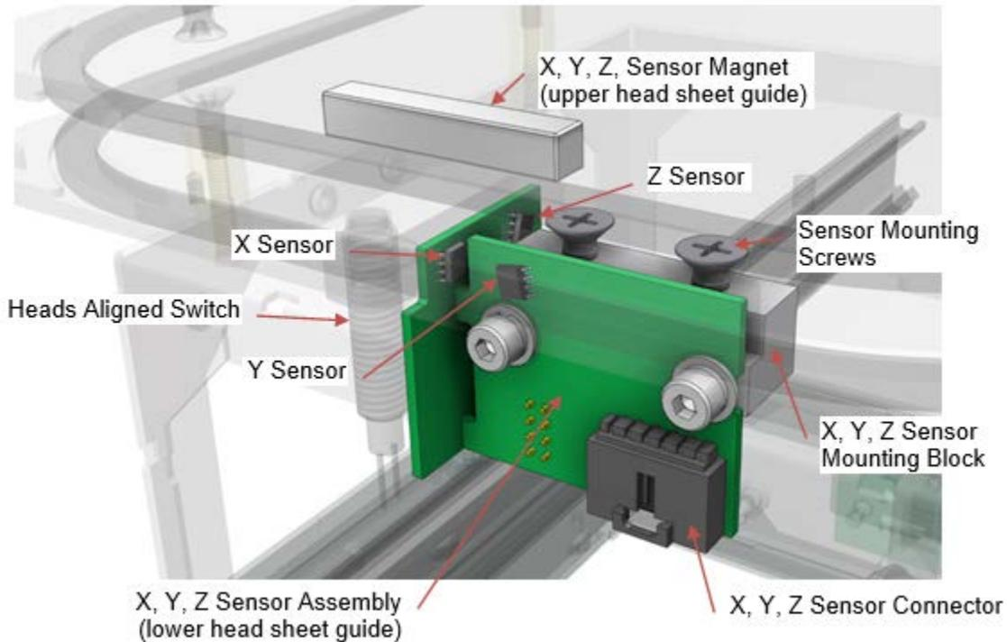
**Figure 6-32: X, Y, Z Sensor and Magnet**
