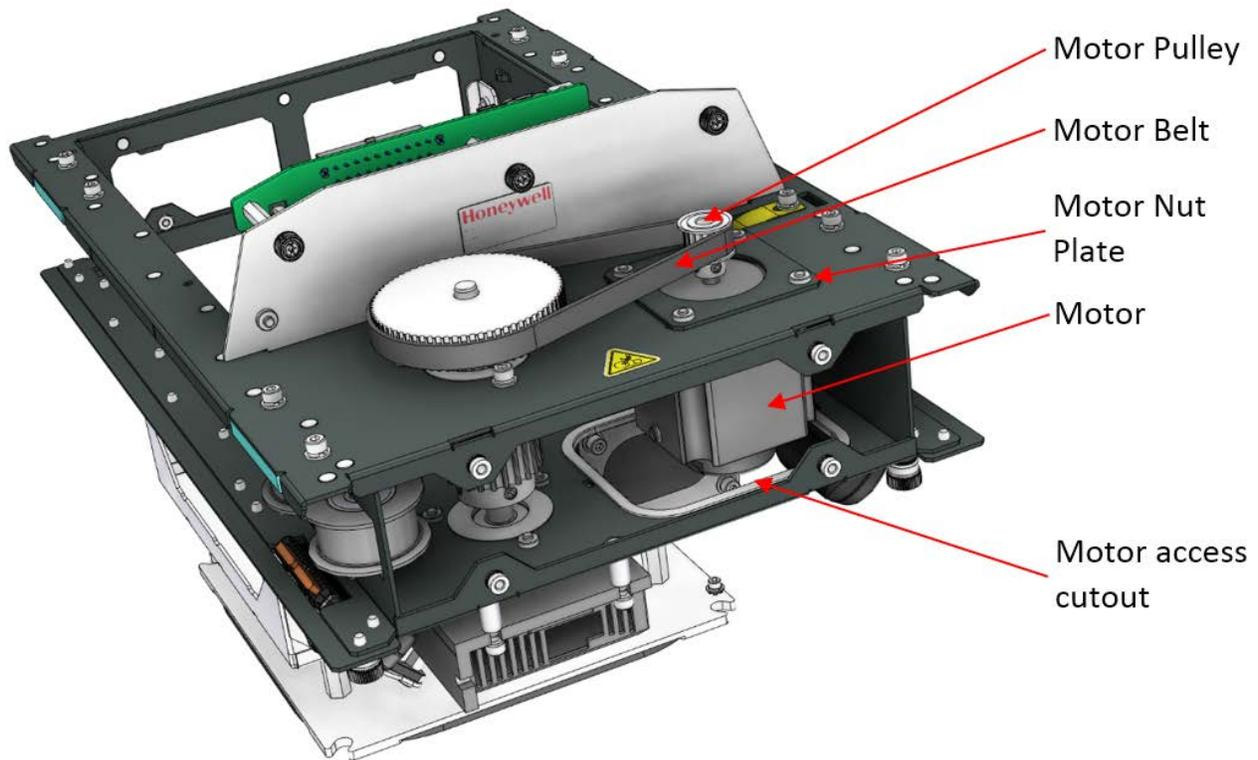
**Figure 8-62: Motor Belt and Motor Nut Plate**
