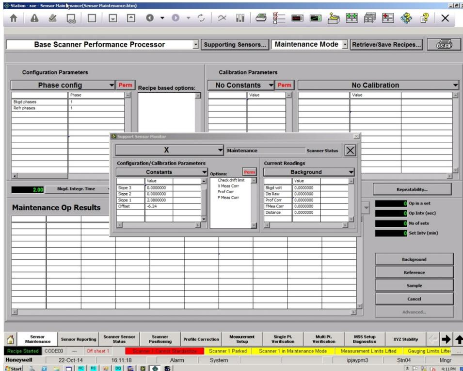
**Figure 8-92: Access X-sensor constants**
