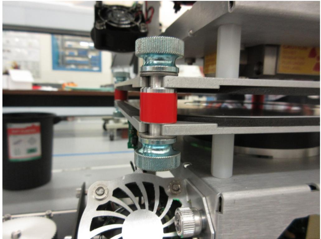
**Figure 8-83: Gap spacers maintain an exact 10mm alignment between heads.**
