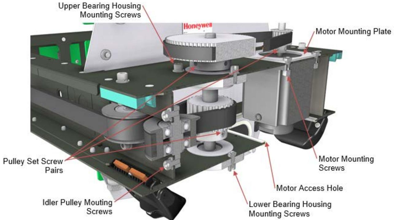
**Figure 6-25: Drive System Mounting Details**
