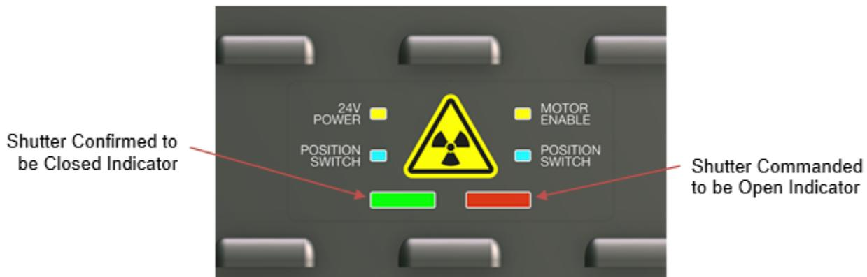
**Figure 2-19: Green and red radiation shutter status indicators on head**
