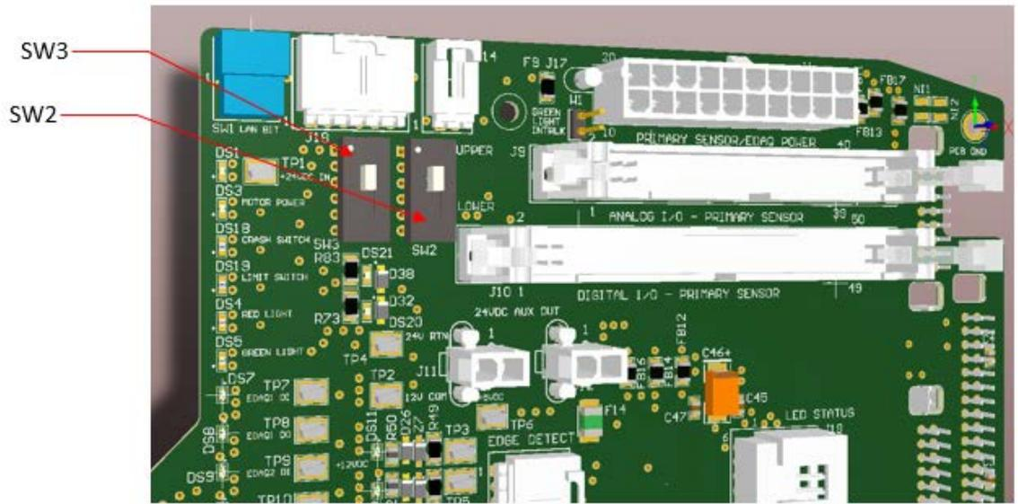
**Figure 8-58: Portion of PCBA depicted with switches SW2 and SW3 in the UP positions.**
