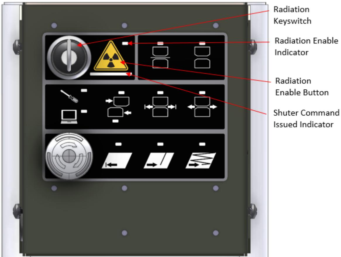
**Figure 8-3: Elements of the “Radiation Sensor Enable Section”**
