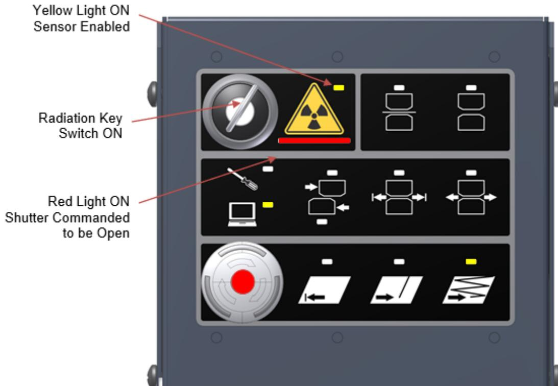
**Figure 2-20: Red shutter status indicator on user panel**
