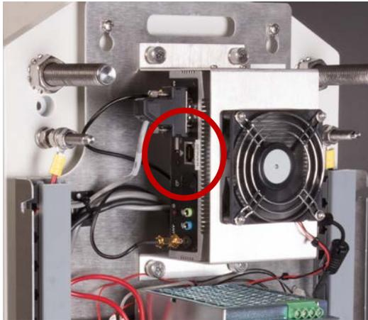
**Figure 4-3: LAN connection on MSS side**
