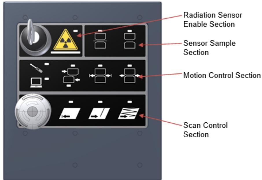
**Figure 6-34: User Control Panel Layout**
