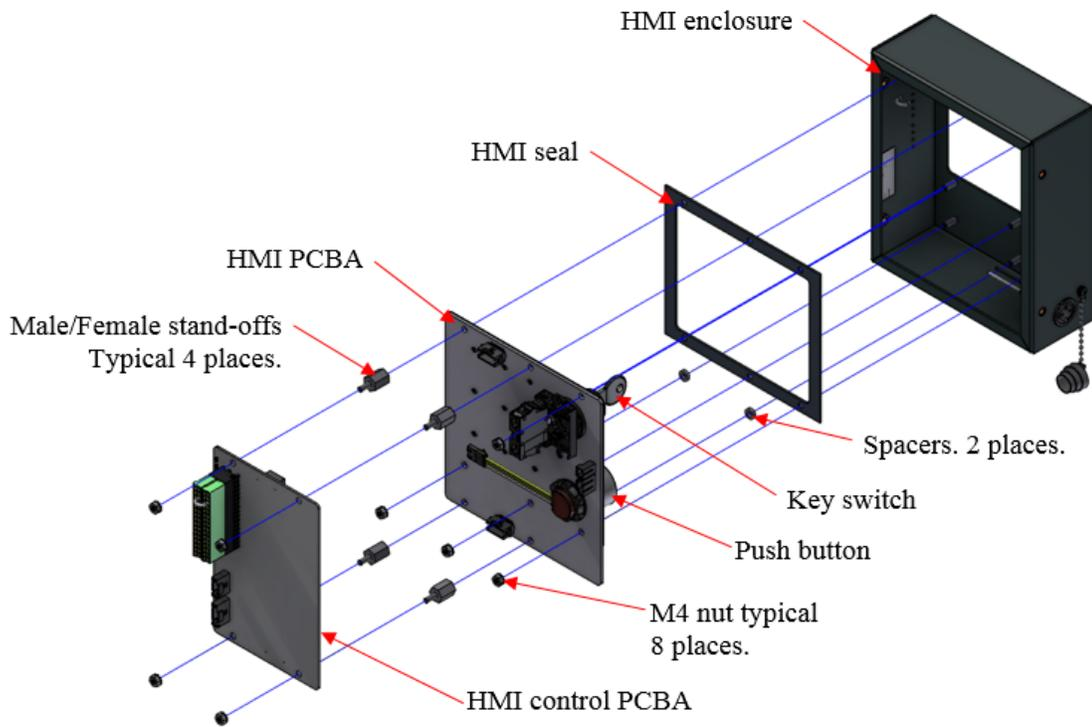
**Figure 8-23: HMI Panel exploded view**
