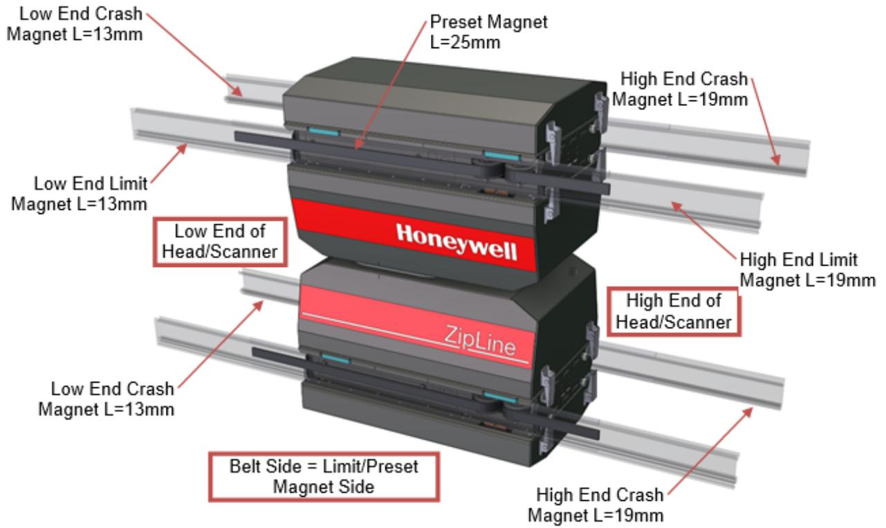
Figure 6-6: Position Magnet Locations Relative to Head Orientation
