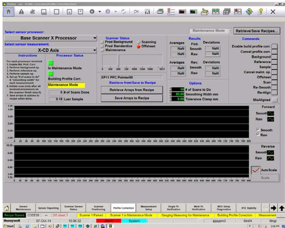
Figure 5-18: Profile correction display
