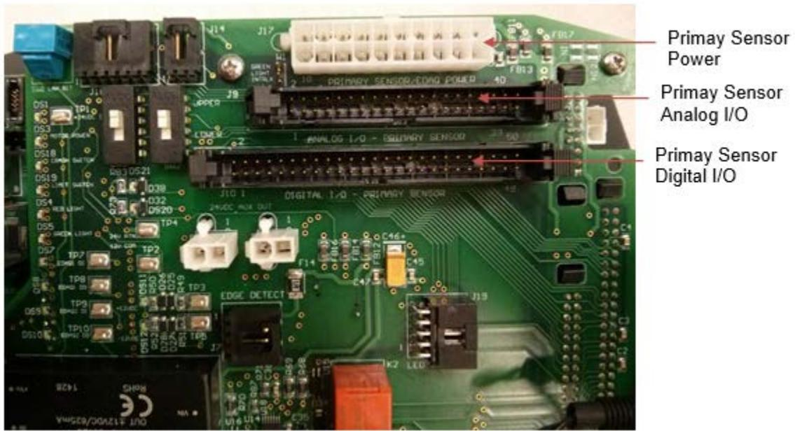
Figure 6-19: Primary Sensor Harness Connections
