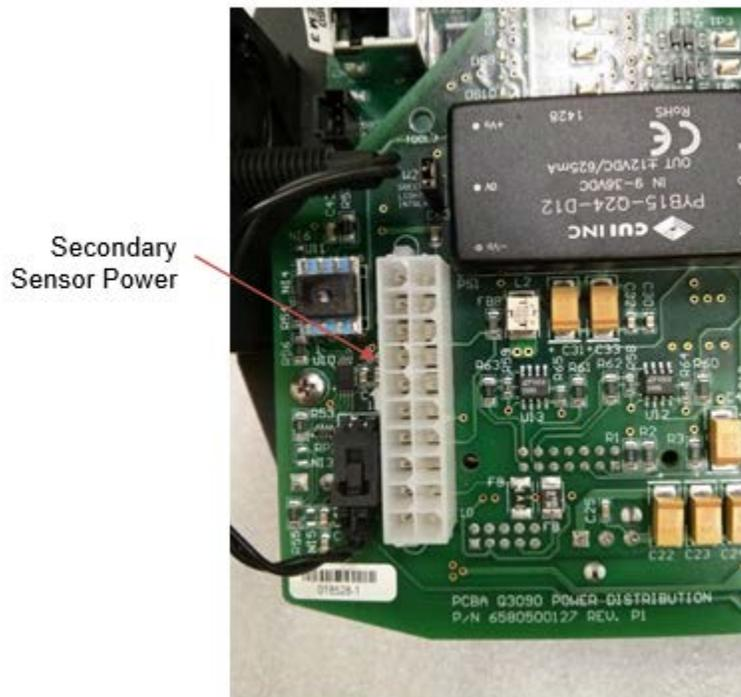
Figure 6-20: Secondary Sensor Harness Power Connection
