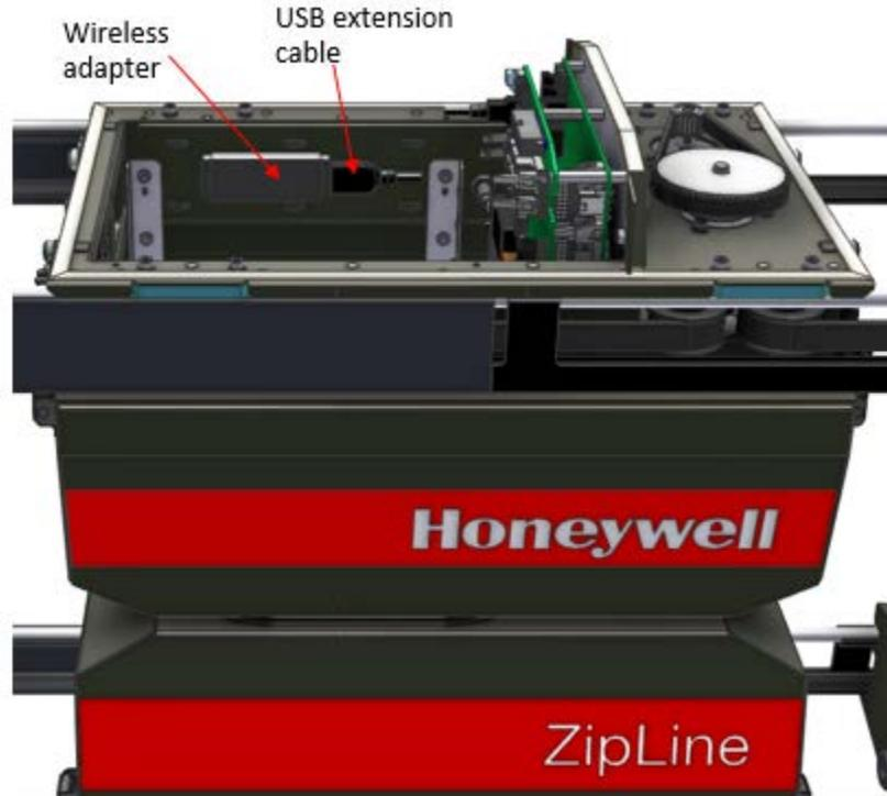
**Figure 8-42: Location of wireless adapter in the upper measurement module**
