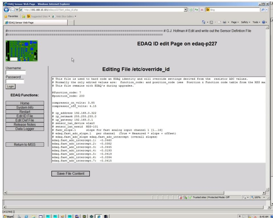
**Figure 5-9: Set pressure limits on upper EDAQ ID file**
