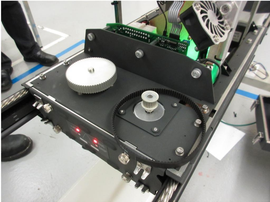
**Figure 8-82: Remove lower head motor belt from head drive system.**
