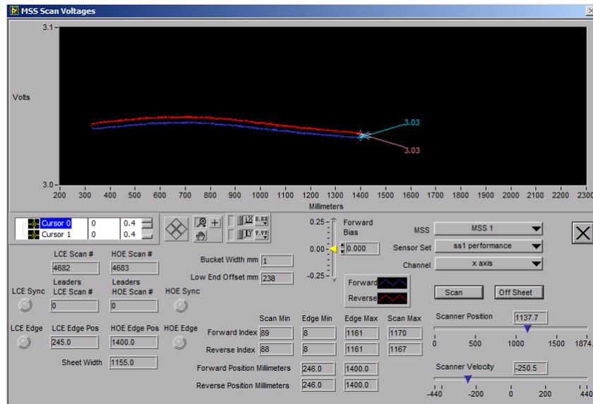
**Figure 8-91: MSS scan voltage showing x-signal when heads are aligned**
