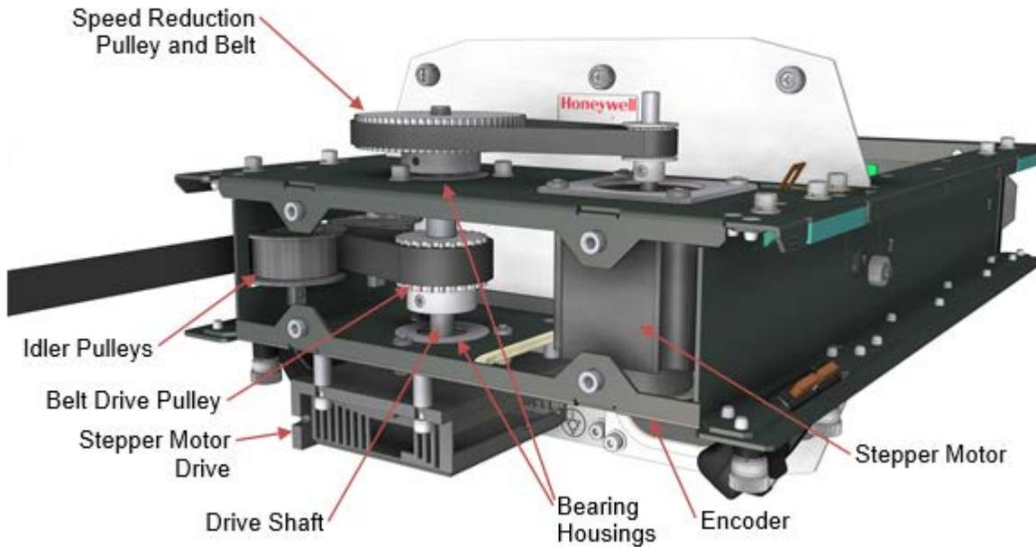
**Figure 6-23: Drive Components and Belt Access (End Cover Removed)**
