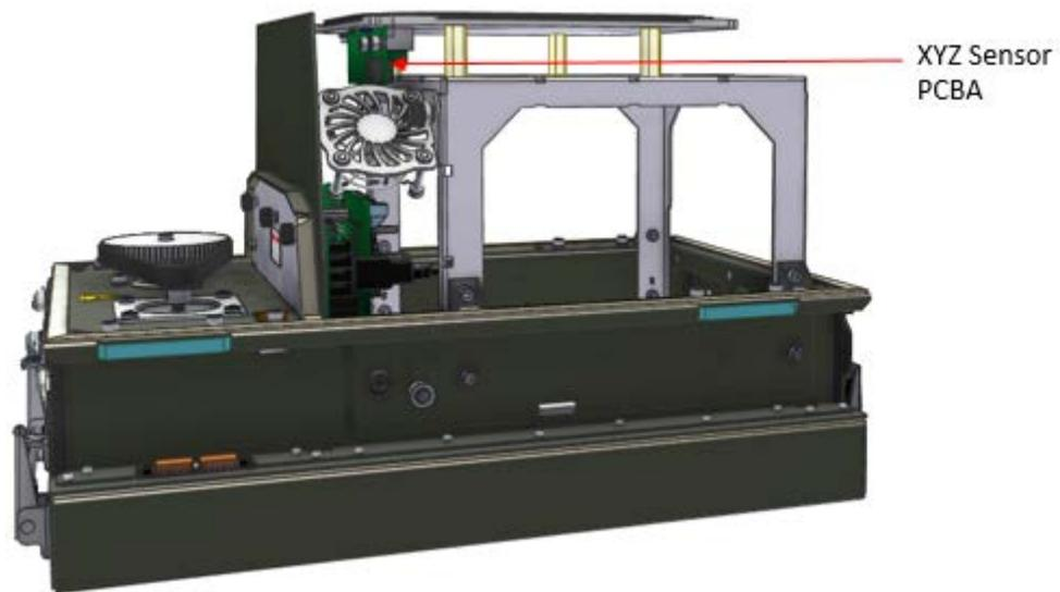
**Figure 8-48: Lower measurement module with upper cover removed**
