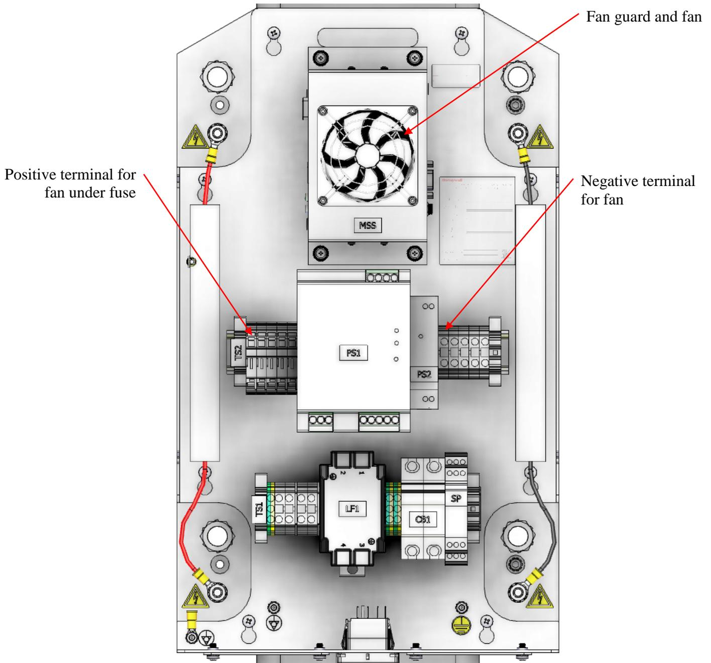
**Figure 8-27: Cable End electronics (cover removed)**
