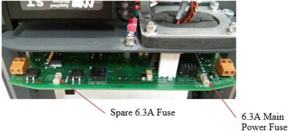
**Figure 6-17: Power Distribution Board Fuse Location**
