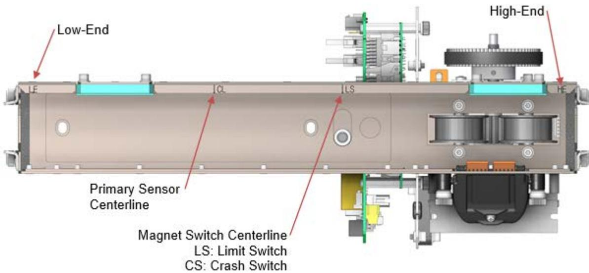
**Figure 6-7: Head Markings: Switch Location, Centerline, High End, Low End**
