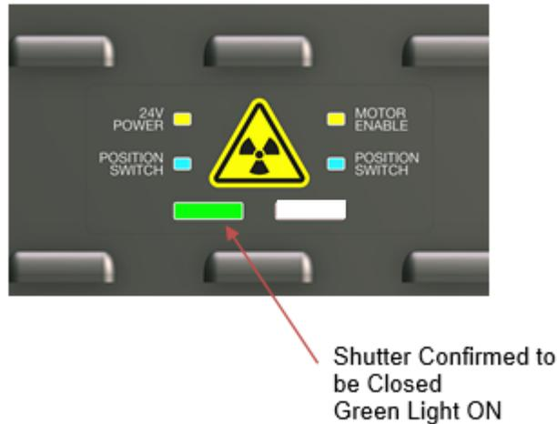
**Figure 2-18: Green shutter closed indicator on upper head**
