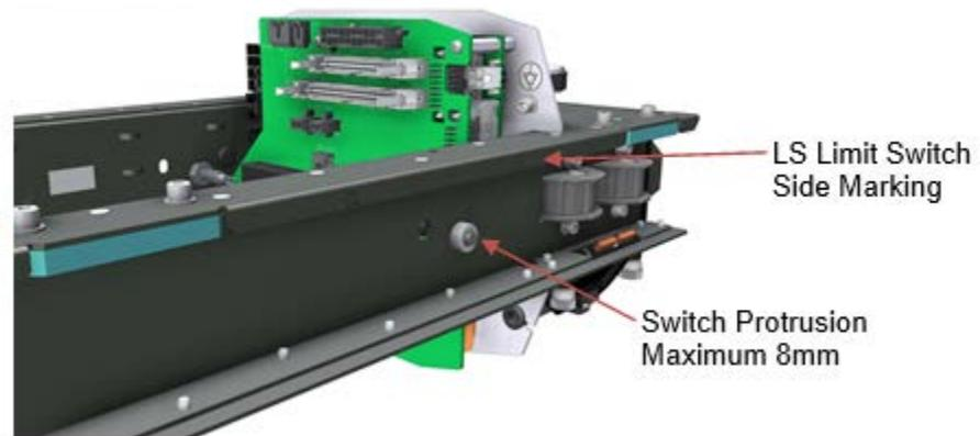
**Figure 6-29: Magnet Position Switch Protrusion Length**
