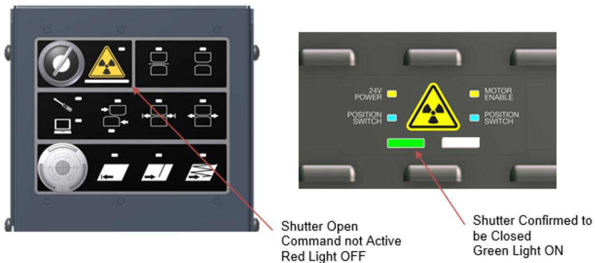
**Figure 2-10: Safe user panel radiation shutter status, green light on**
