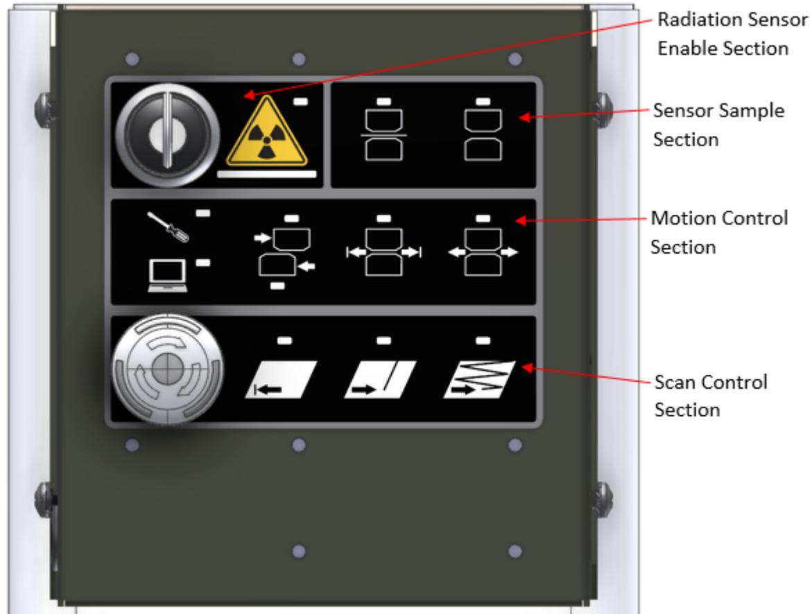
**Figure 8-2: HMI panel function groupings**
