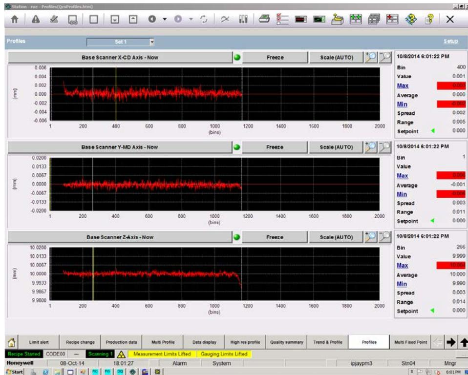
Figure 5-23: X, Y and Z profiles with heads locked together and profile correctors applied
