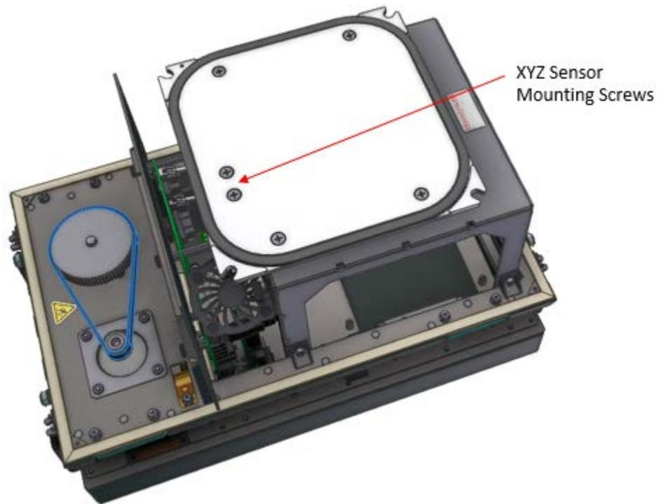
**Figure 8-50: Location of XYZ sensor assembly mounting screws on topside of sensor platform**
