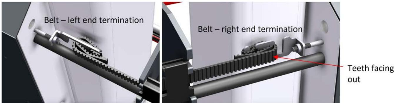
**Figure 8-80: Belt Left/Right End Terminations**
