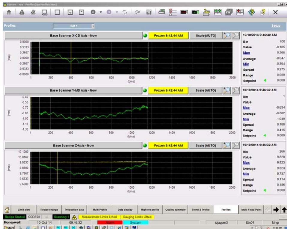
**Figure 8-96: Representative X, Y, and Z passing ZipLine alignment**
