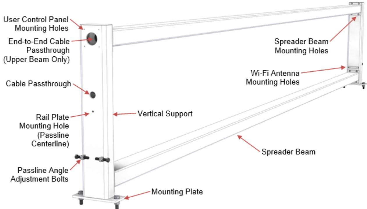
**Figure 6-2: Compression Frame Assembly**
