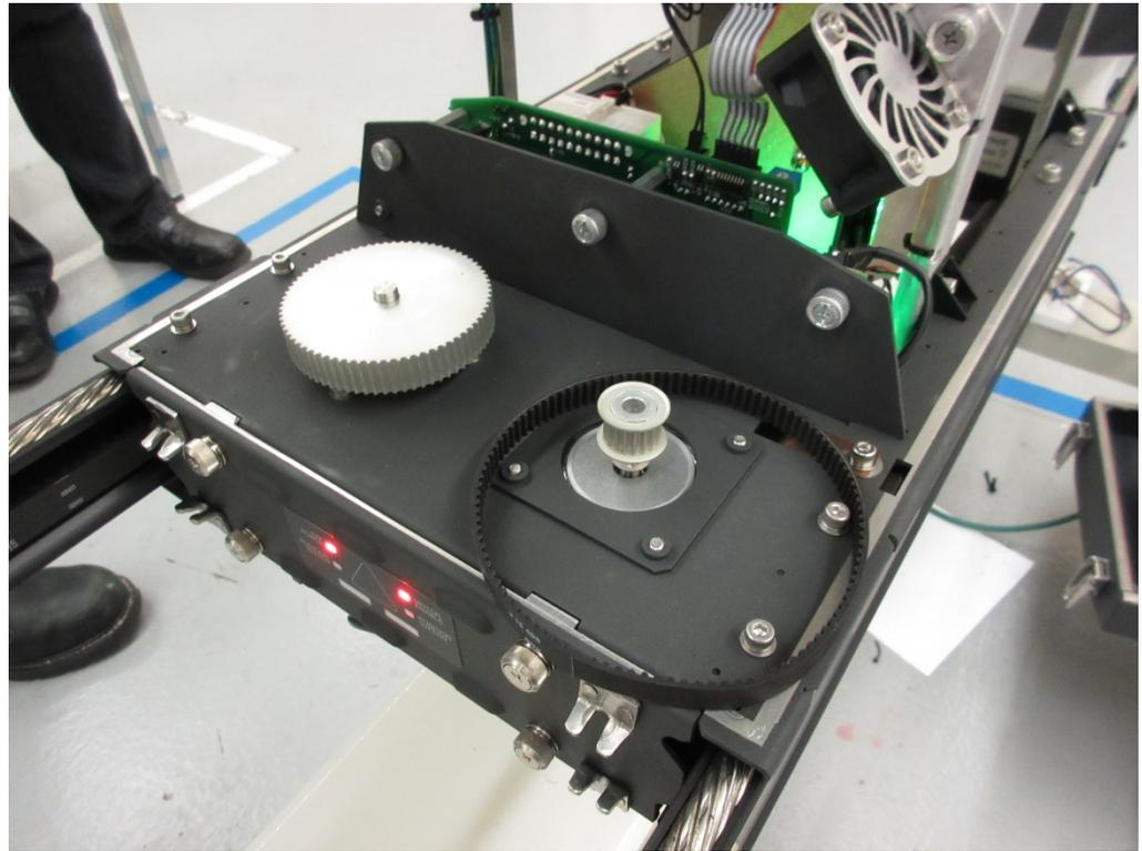
**Figure 5-16: Remove lower head motor belt from head drive system**
