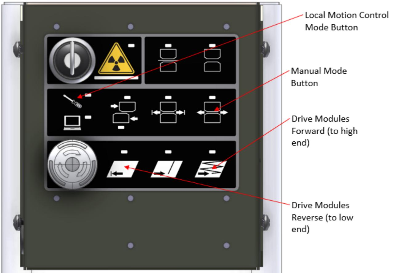
**Figure 8-9: Layout of user panel buttons used for Manual Mode control of the measurement modules**
