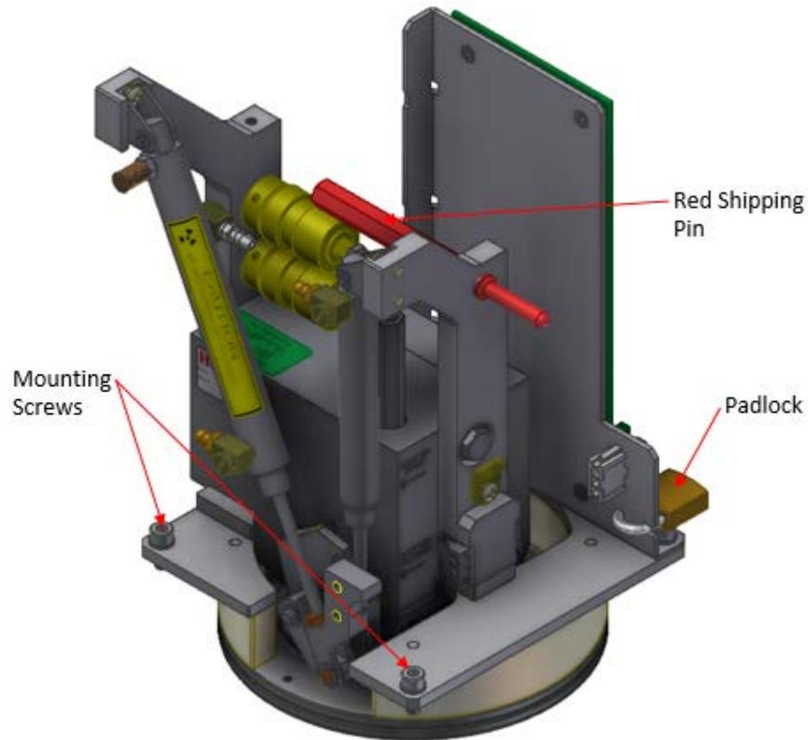
**Figure 8-28: SX18 nuclear gauge source side showing mounting screws, padlock, and shipping pin in its storage position**
