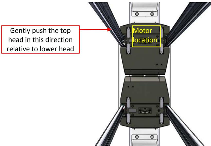
**Figure 8-72: Orientation of head to stimulate Y response.**
