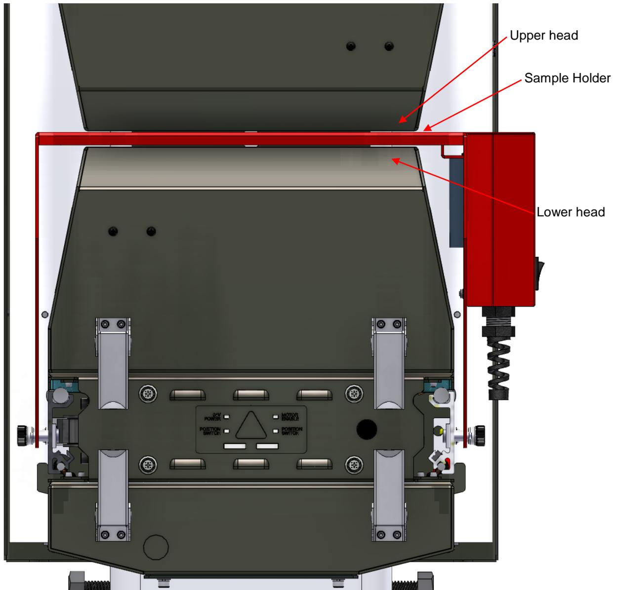
**Figure 8-103: Upper & Lower Heads over Sample Holder**
