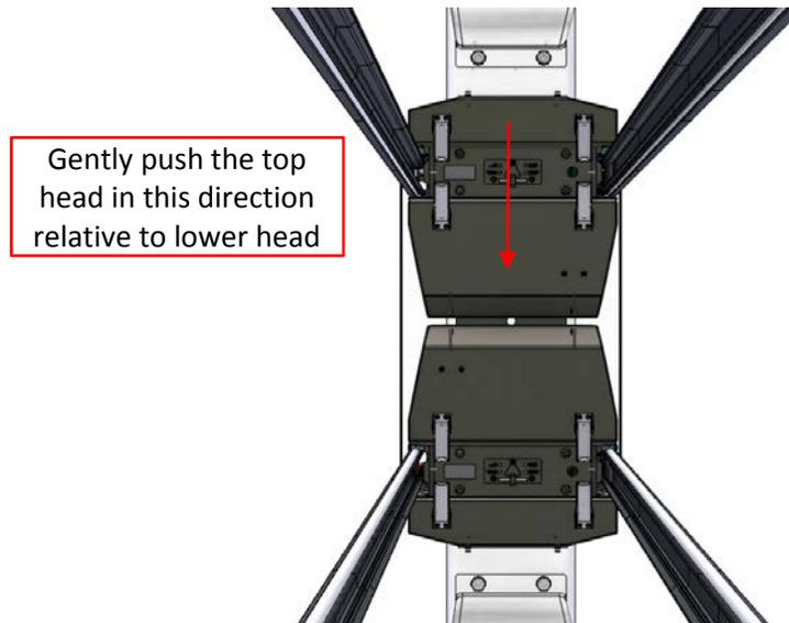
**Figure 8-73: Orientation of head to stimulate Z response.**
