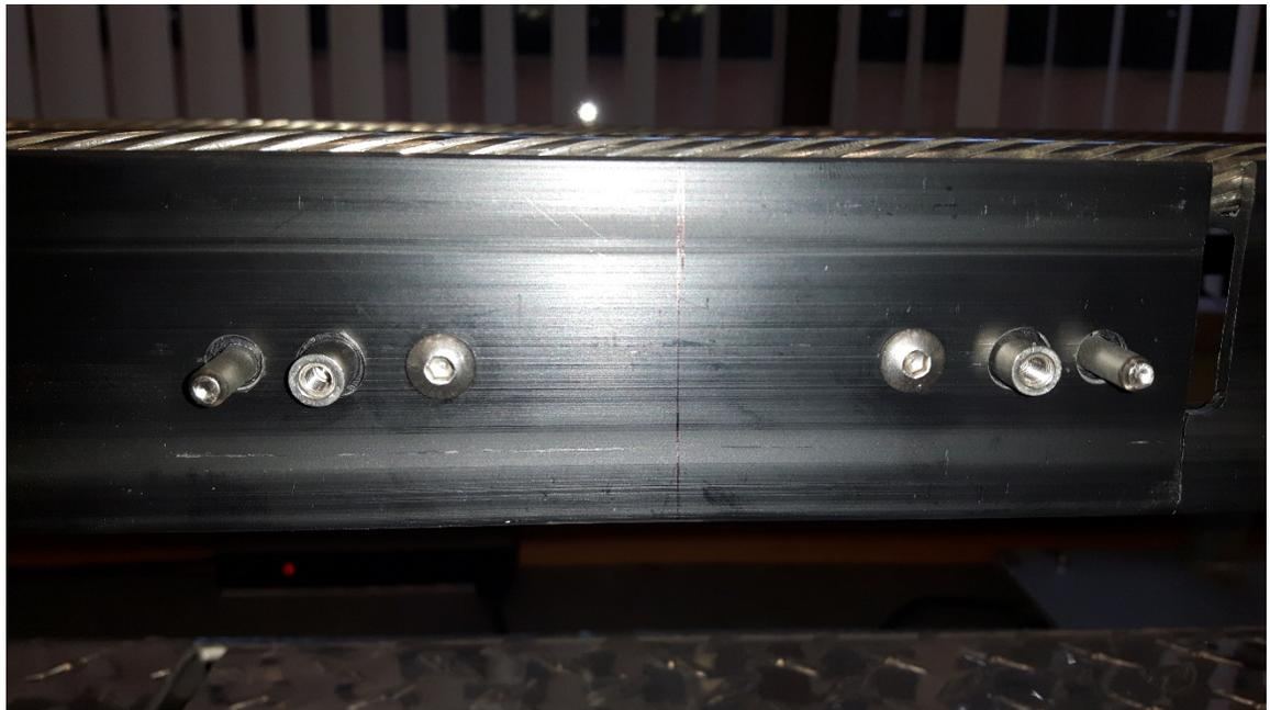
**Figure 8-101: Sample Nut Plate Holder installed**
