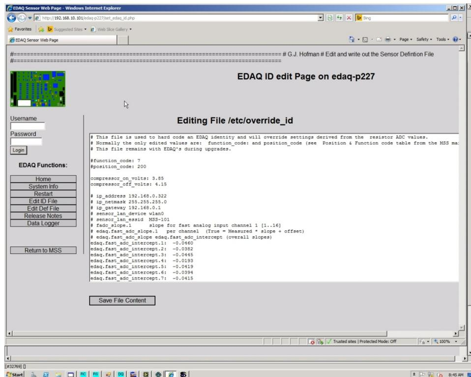
**Figure 8-68: Set pressure limits on upper EDAQ ID file**
