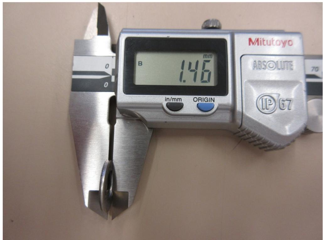
Figure 5-28: Physical measurement of additional spacing washer
