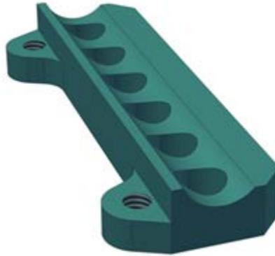
**Figure 6-22: Linear Bearing**
