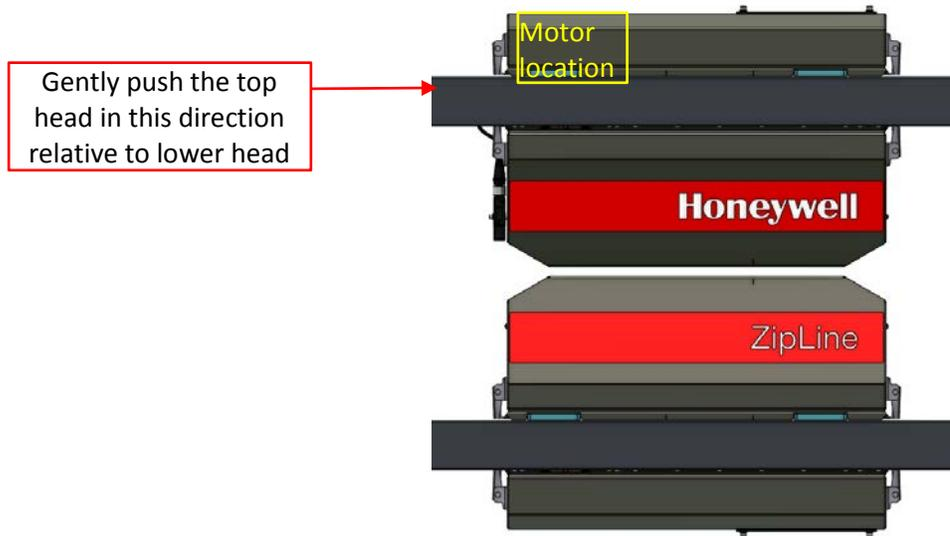
**Figure 8-71: Orientation of head to stimulate X response.**
