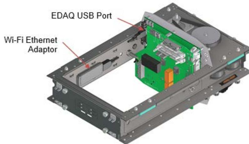
**Figure 6-21: Wi-Fi Ethernet Adapter**
