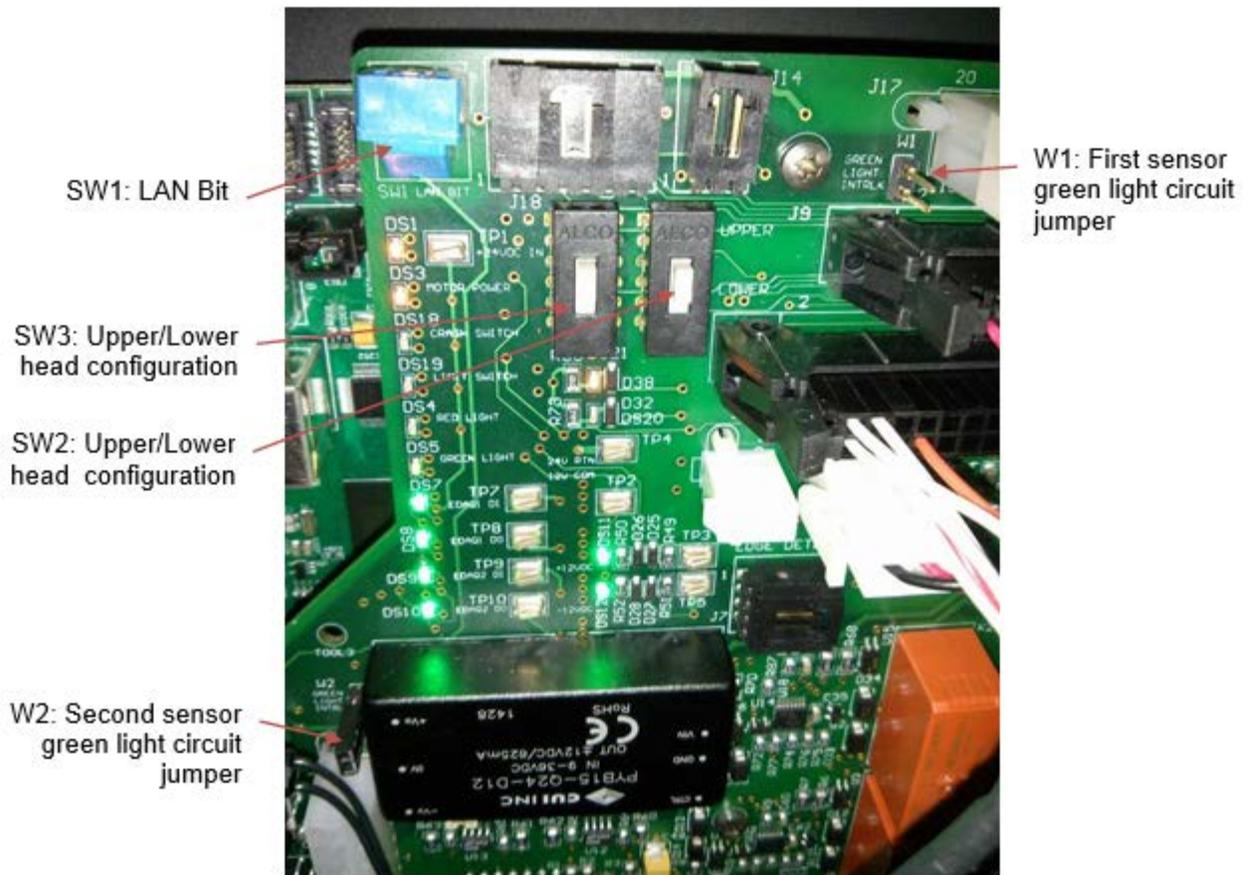
Figure 6-16: Power Distribution Board Jumper and Switch Configurations
