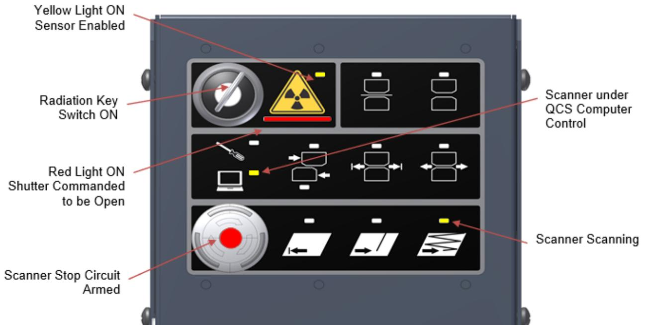
**Figure 2-9: Typical user control panel during scanning operation, red light shutter open radiation status on**
