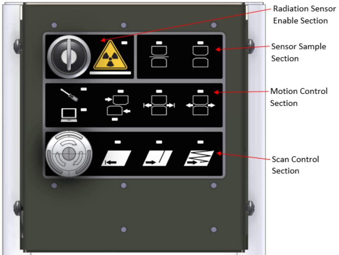
**Figure 8-5: HMI panel function groupings**
