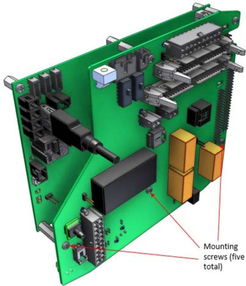
**Figure 8-56: Mounting screws mate the PDB to the standoffs connected to the EDAQ**
