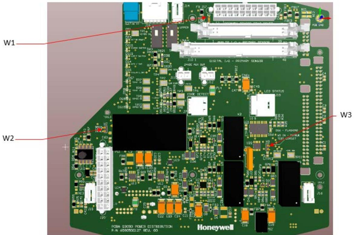
**Figure 8-59: Locations of jumpers W1, W2, and W3 on the Head Power Distribution PCBA**
