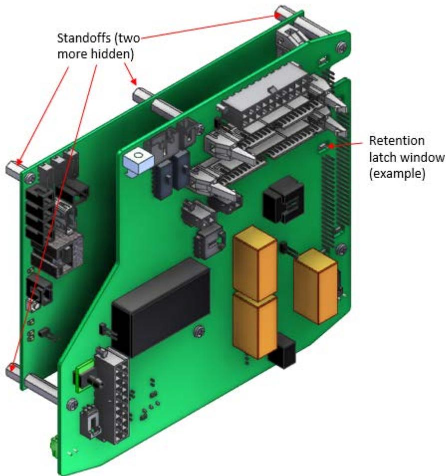
**Figure 8-52: PDB/EDAQ assembly removed from measurement module**
