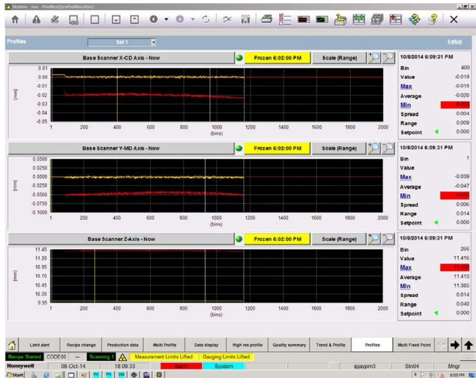
Figure 5-27: Z sensor measures the additional space after calibration
