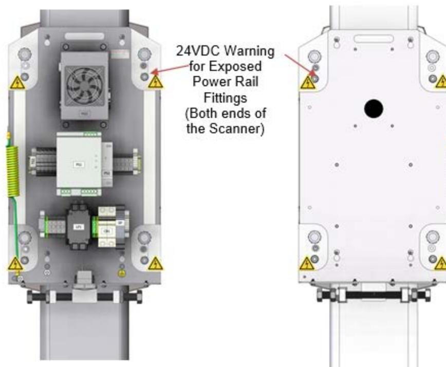
**Figure 2-7: End bell electrical warning for exposed 24 VDC power rail fittings**
