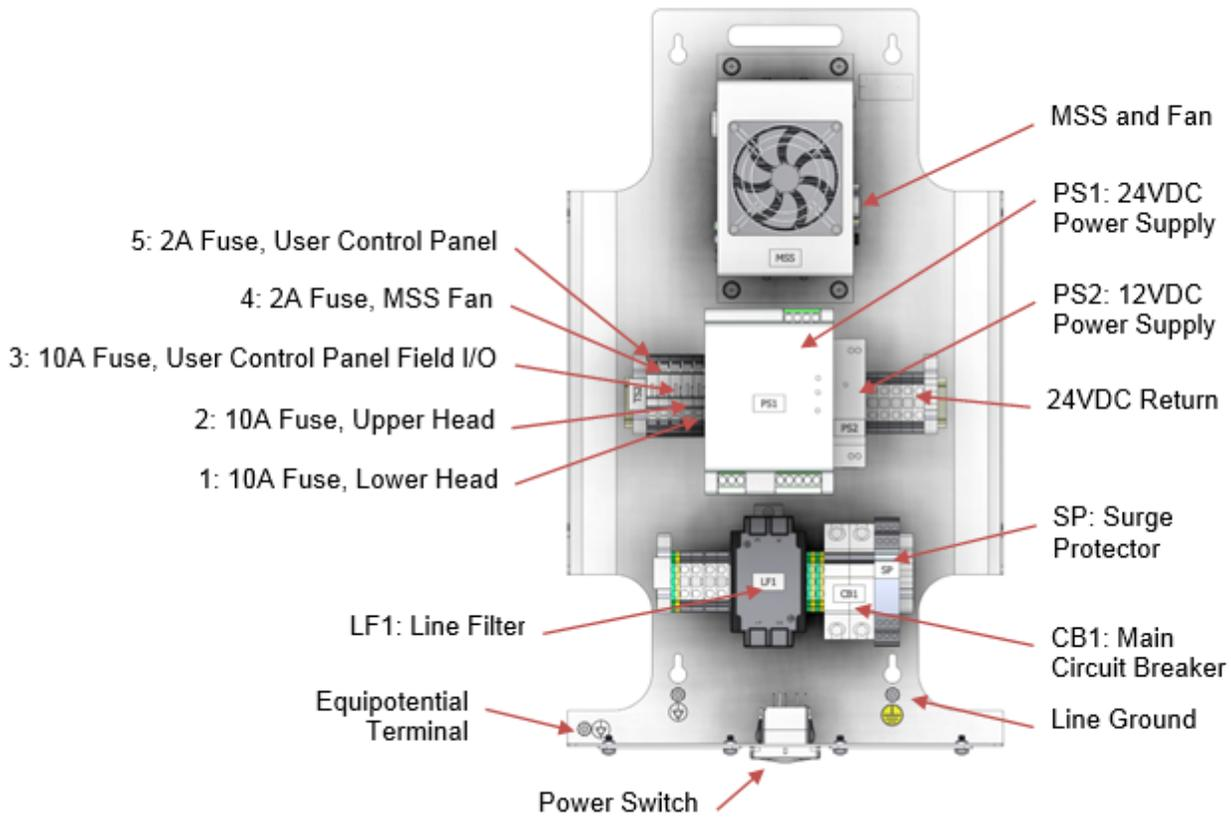
**Figure 6-11: Electrical Circuit Protection Devices**
