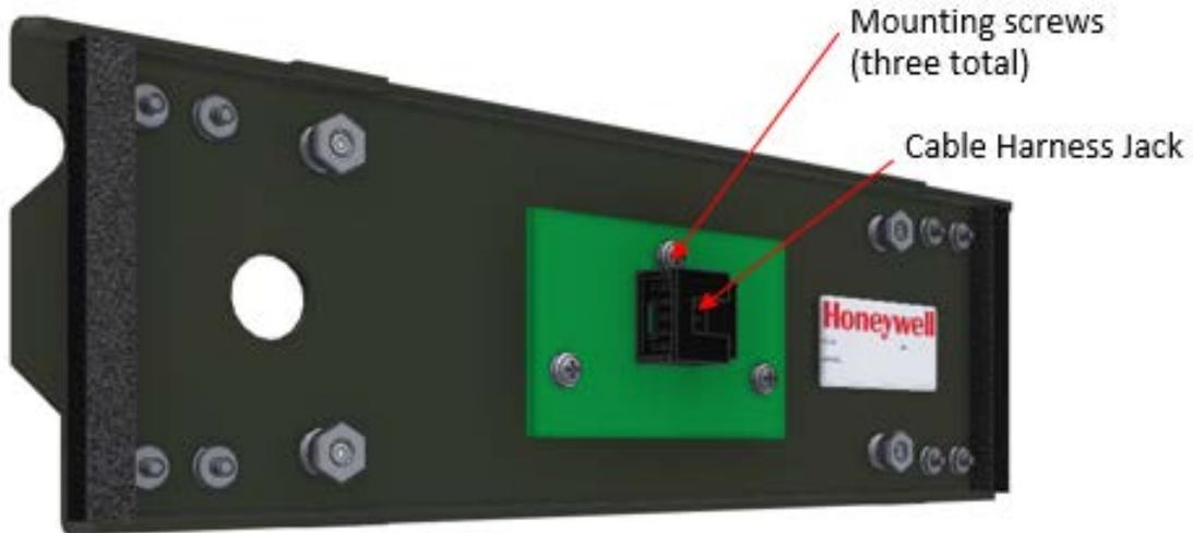
**Figure 8-39: Backside of the end plate cover with the backside of the head status LED PCBA visible as well as its three mounting screws**
