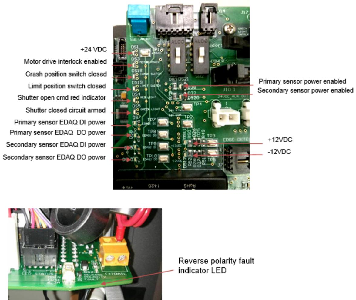
**Figure 6-18: Power Distribution Board Indicator LEDs**
