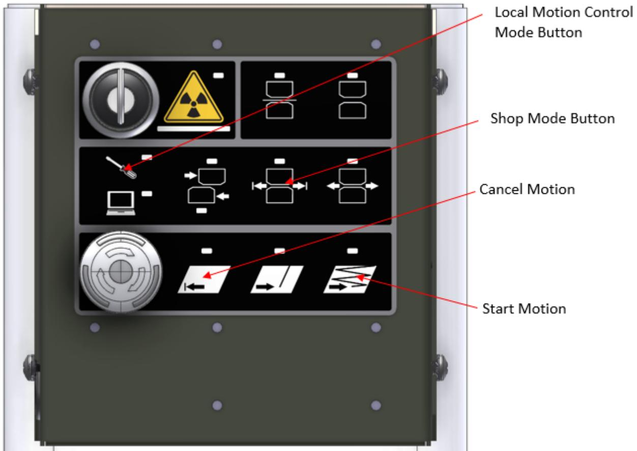
**Figure 8-12: Layout of user panel buttons for Shop Mode control of the measurement modules**
