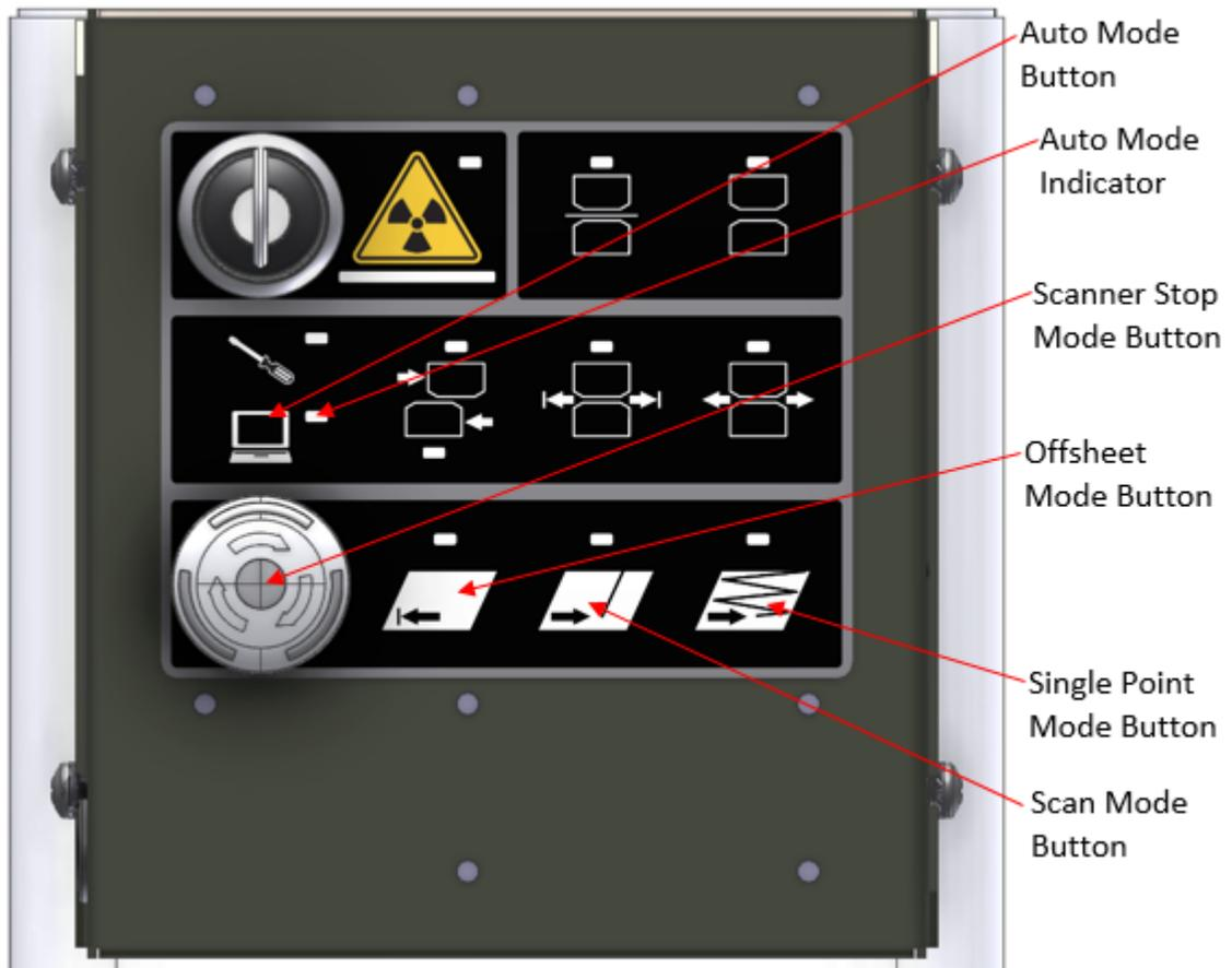
**Figure 8-6: Scanner Auto Mode indicators and actuation button layout**
