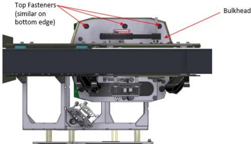
**Figure 8-55: Location of fasteners which secure the PDB/EDAQ assembly inside the measurement module**
