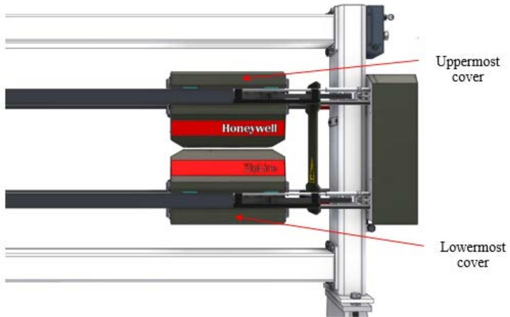
**Figure 8-41: Only need to remove one cover to replace the wireless adapter**
