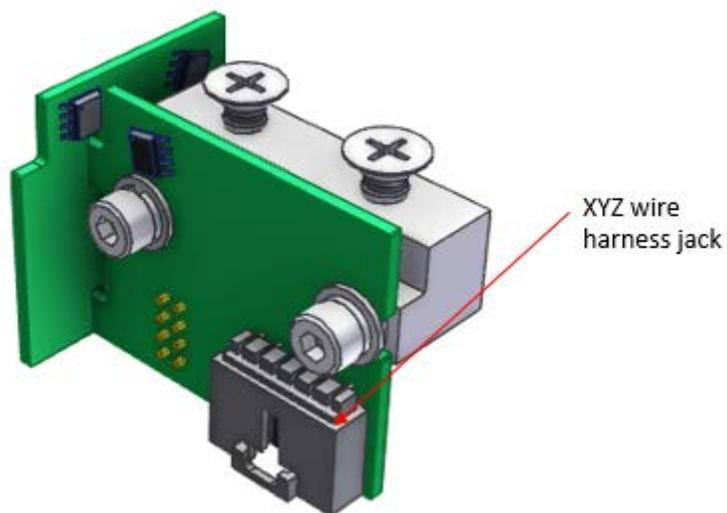
**Figure 8-49: XYZ sensor assembly with PCBA and mounting bracket**
