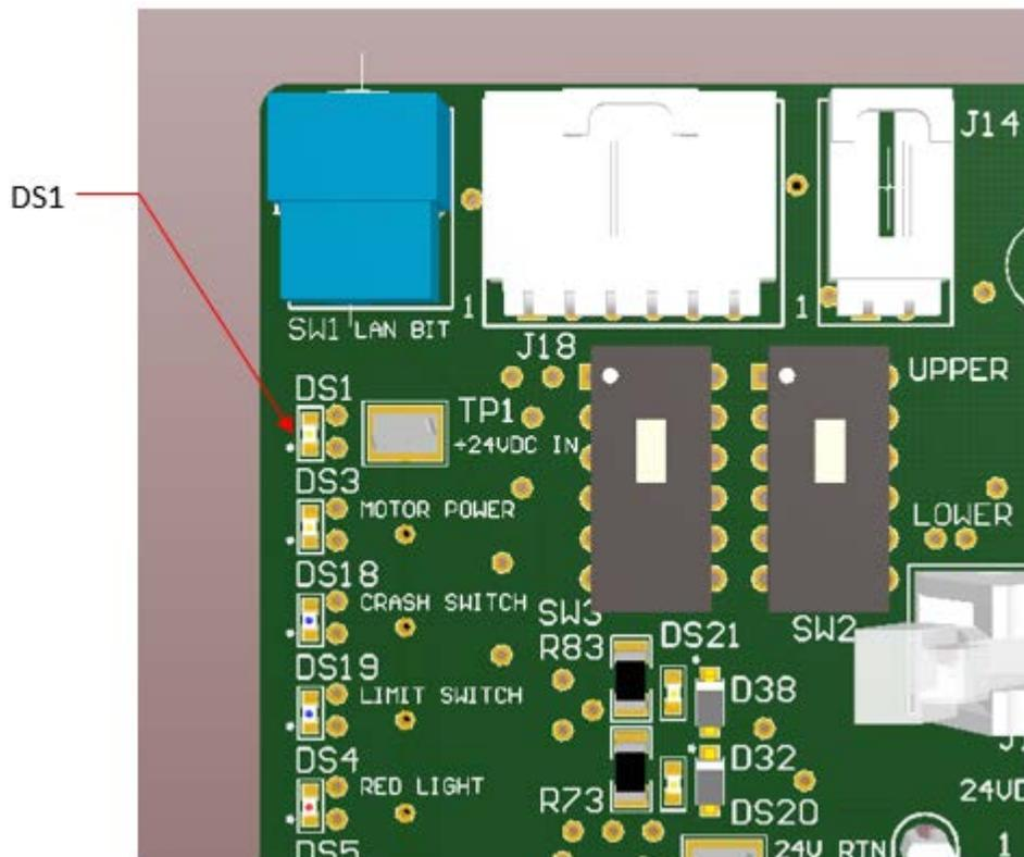
**Figure 8-44: Location of DS1 on the top left hand corner of the head power distribution PCBA on the front side**
