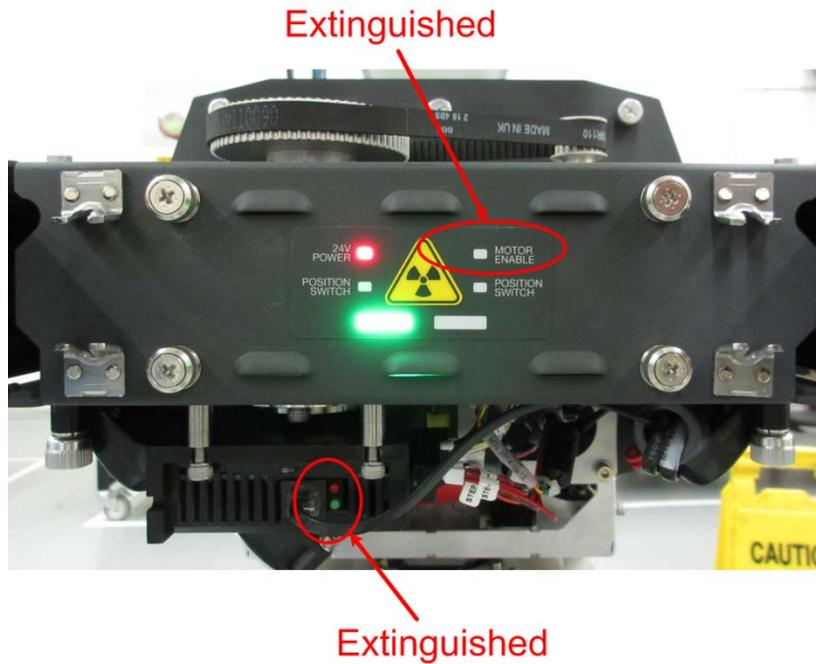
**Figure 5-2: Motor controller disabled.**
