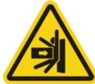
**Figure 2-3: Squeeze/Impact Warning Label**
