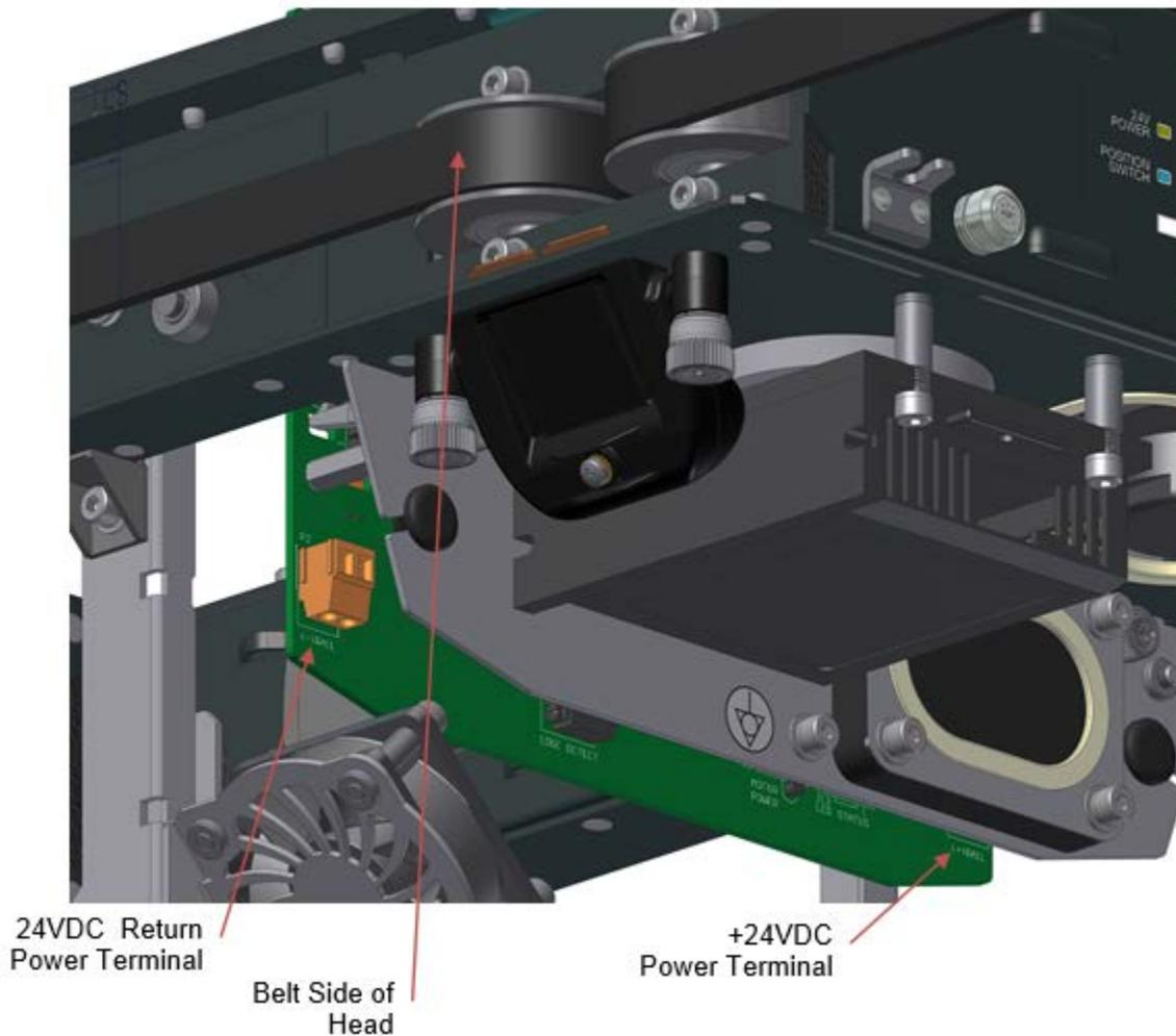
**Figure 6-10: Head Polarity Markings**
