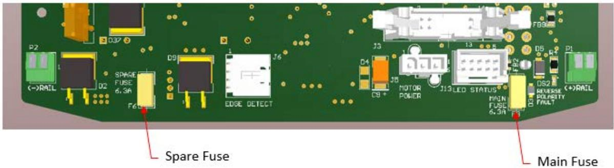
**Figure 8-43: Locations of the main power fuse and the spare fuse on the backside of the head power distribution PCBA**
