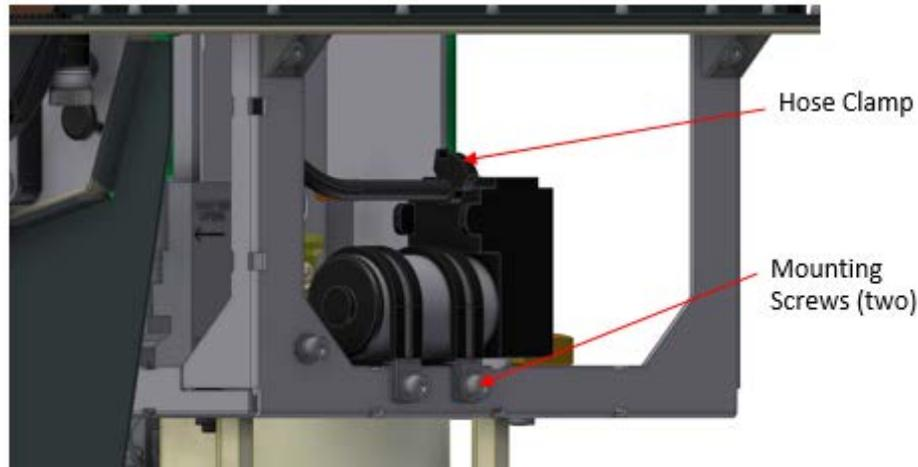
**Figure 8-36: Locations of the compressor clamp mounting screws and the hose clamp. Wire harnesses are not shown**
