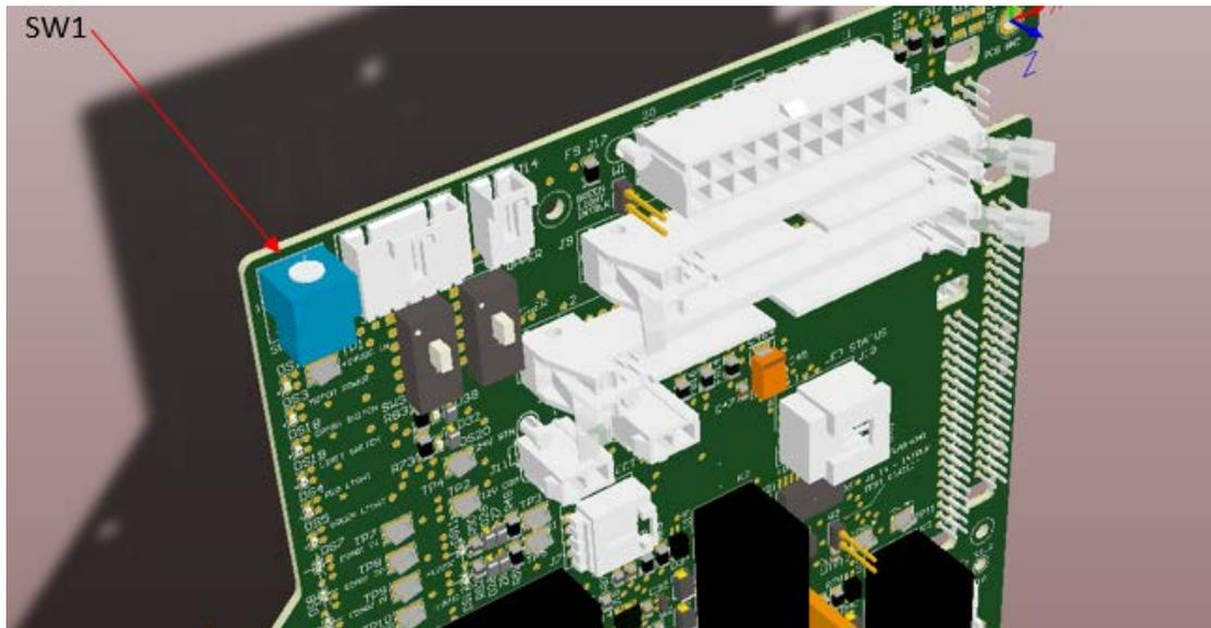
**Figure 8-53: Location of rotary switch SW1 on the PDB PCBA**
