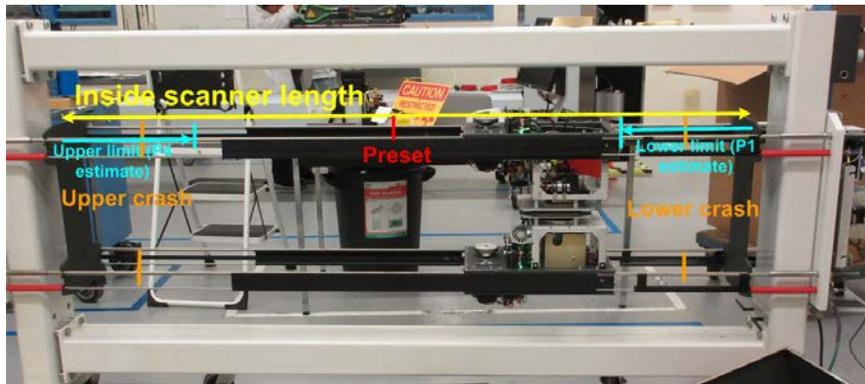
Figure 5-15: Position of limit magnets on the frame
