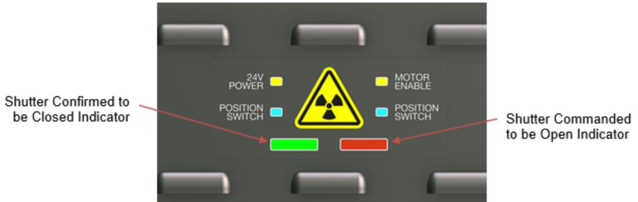
**Figure 2-8: Radiation shutter status indicator (red and green) on upper measurement module only**
