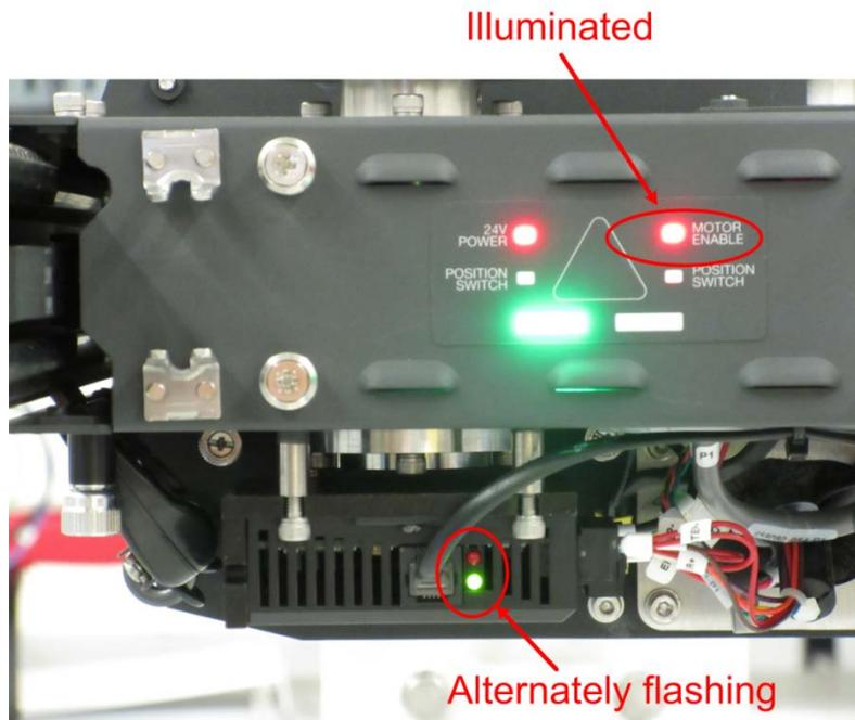
**Figure 5-1: Motor controller enabled**
