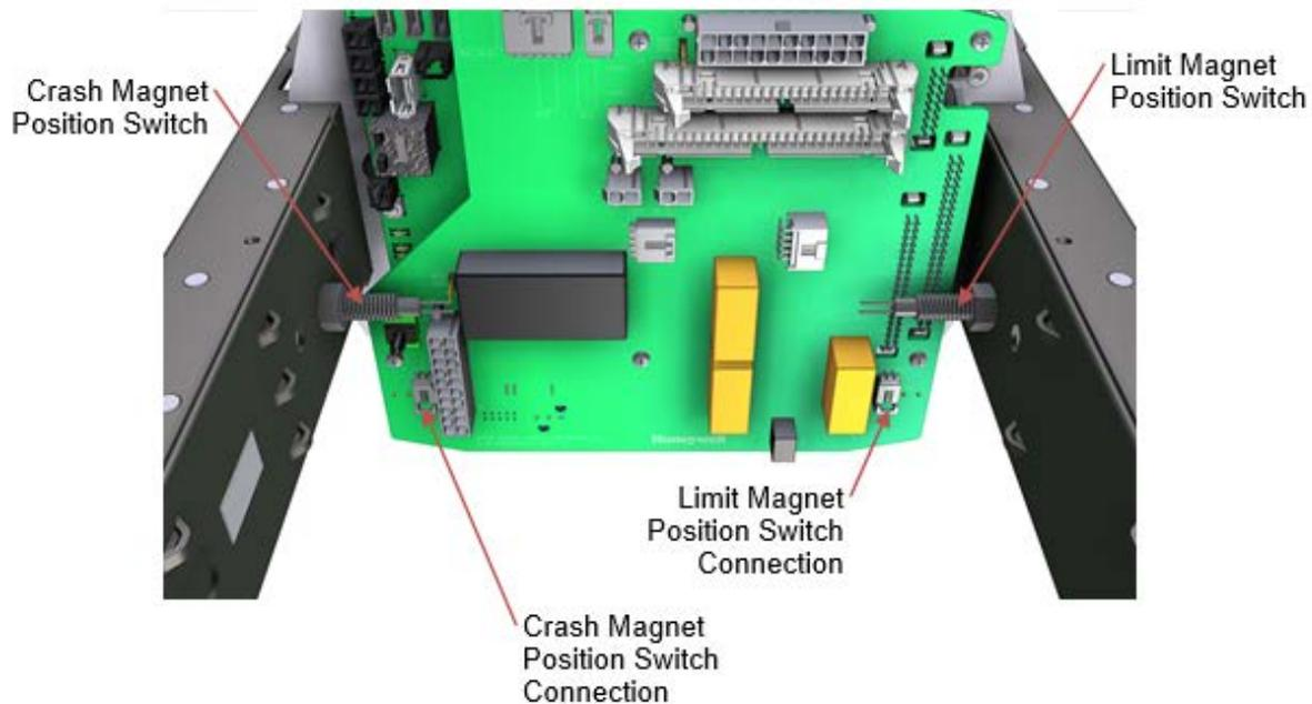
**Figure 6-28: Position Magnet Switches**
