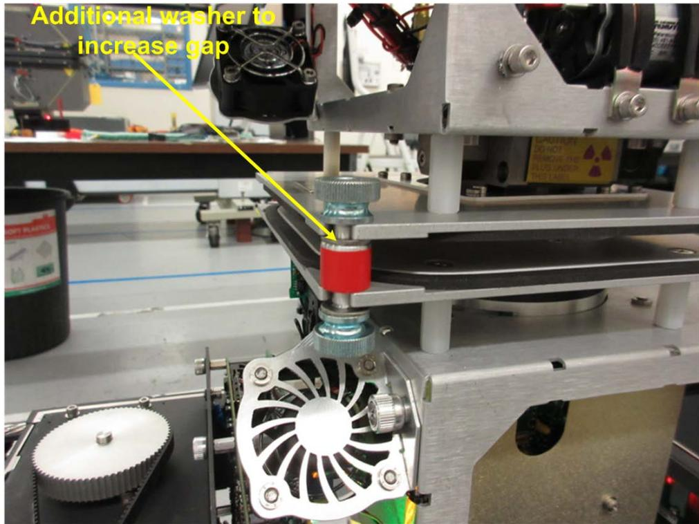
**Figure 5-26: Add additional washer in gap to further separate heads**
