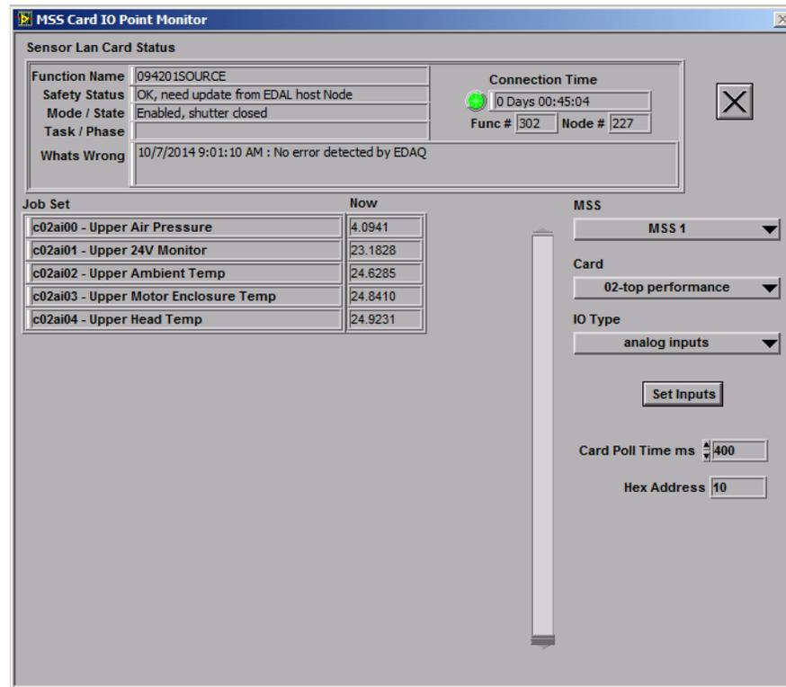
**Figure 5-8: MSS top performance analog inputs**
