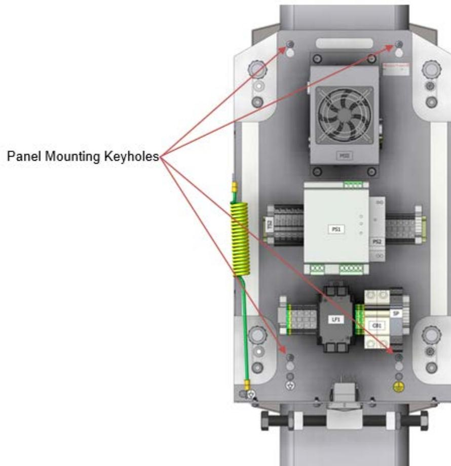
**Figure 6-12: Power Distribution Panel Mounting**
