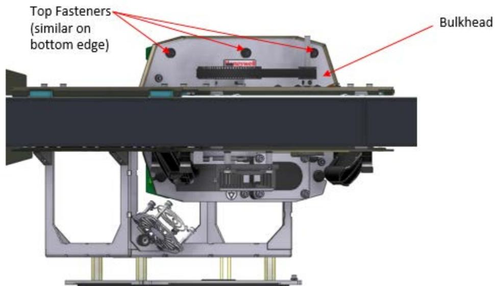
**Figure 8-51: Location of fasteners which secure the PDB/EDAQ assembly inside the measurement module**
