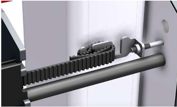
**Figure 8-78: Scanner Drive Belt End Termination Wrap**
