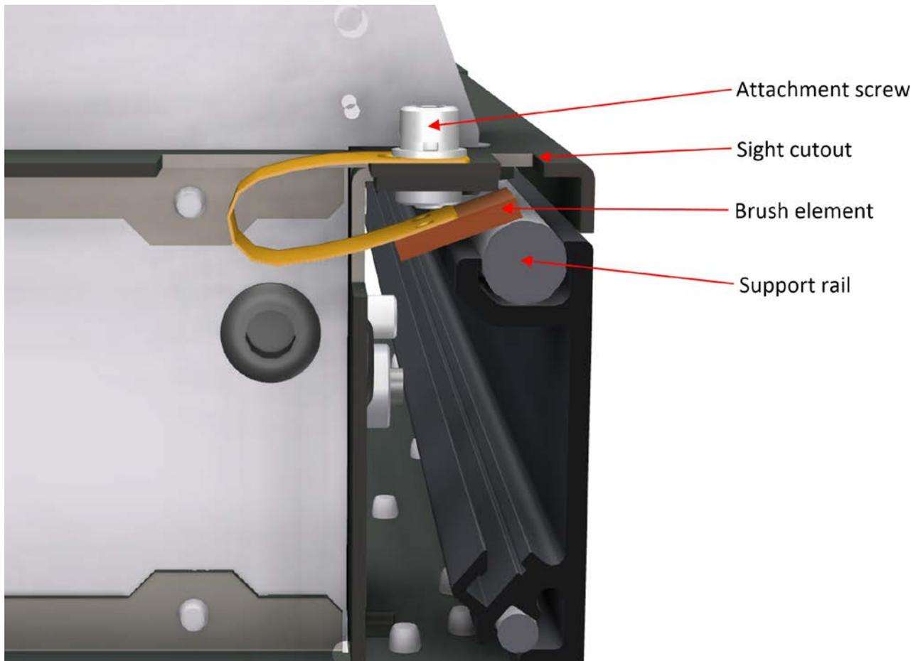
**Figure 8-32: Ground Brush Cross Section**
