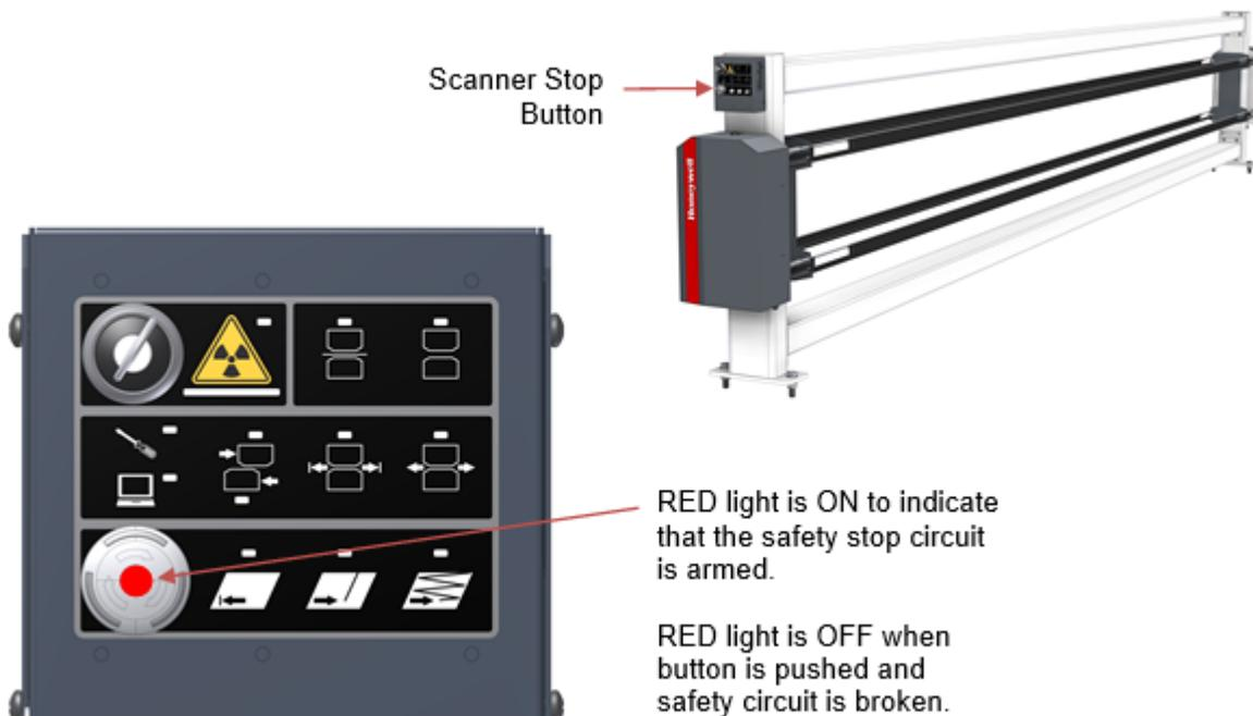
**Figure 2-16: Scanner stop button**
