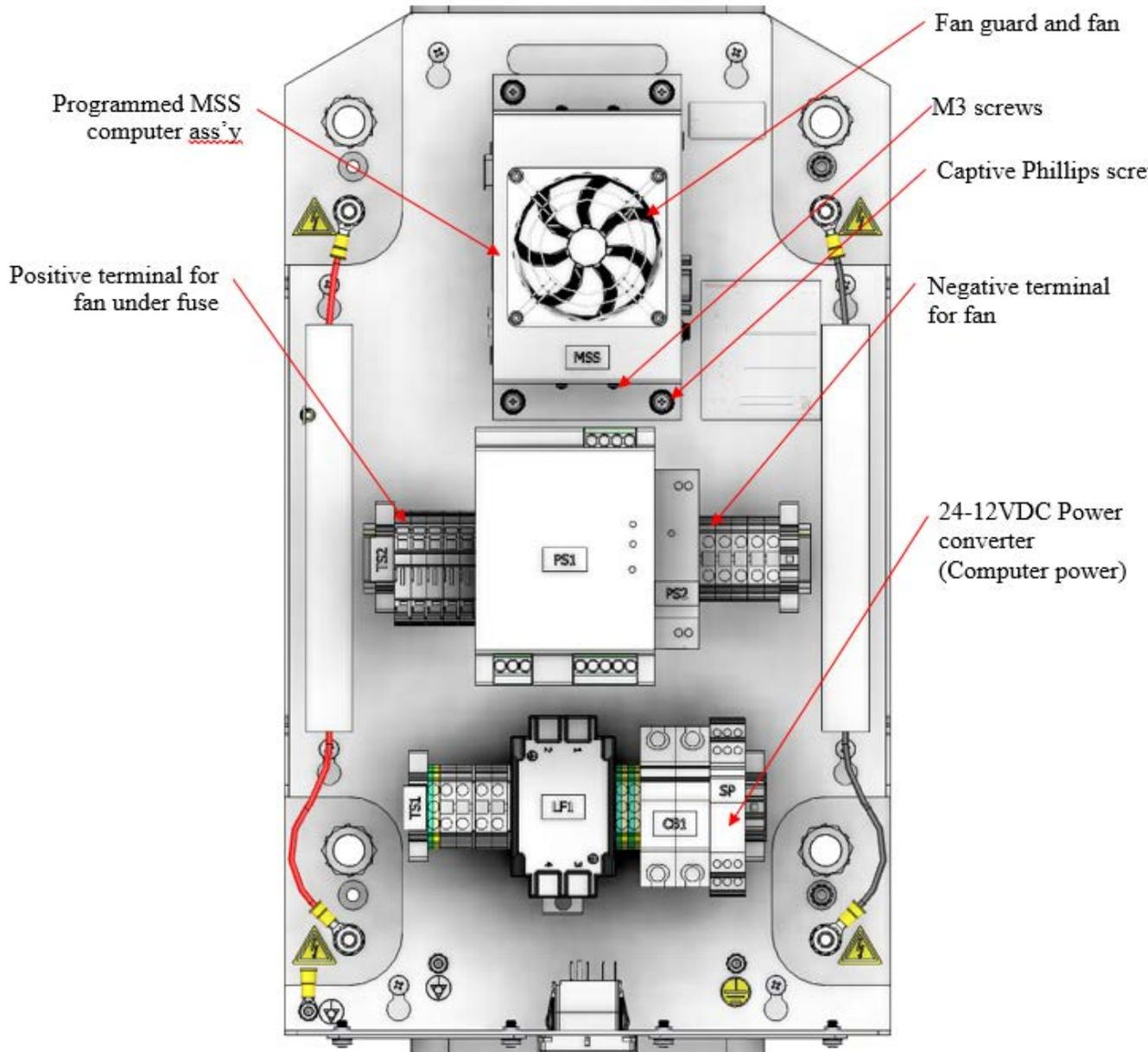
**Figure 8-26: Cable End electronics (cover removed)**
