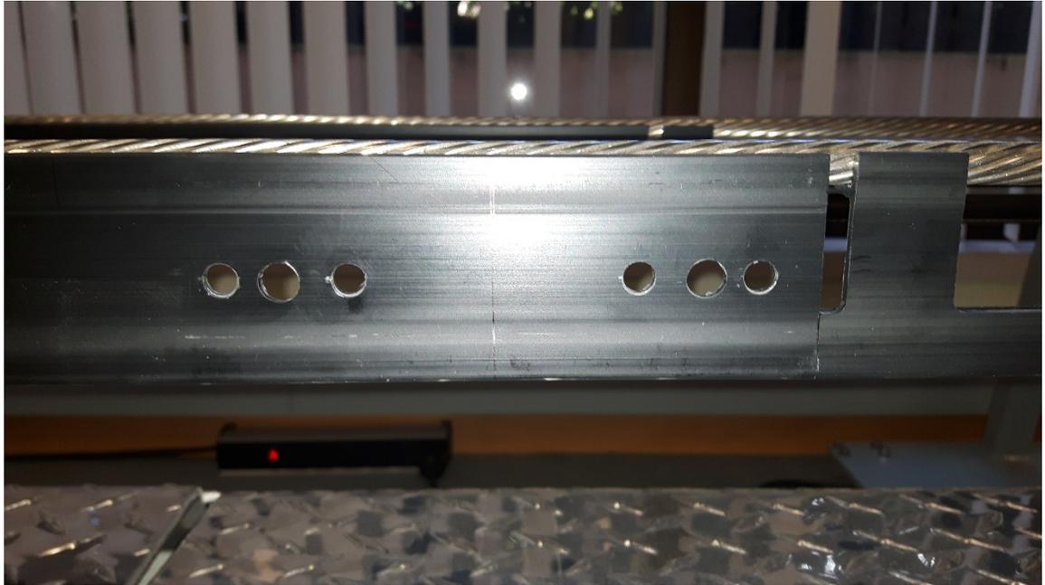
**Figure 8-100: Plastic Rail Cover drilled**
