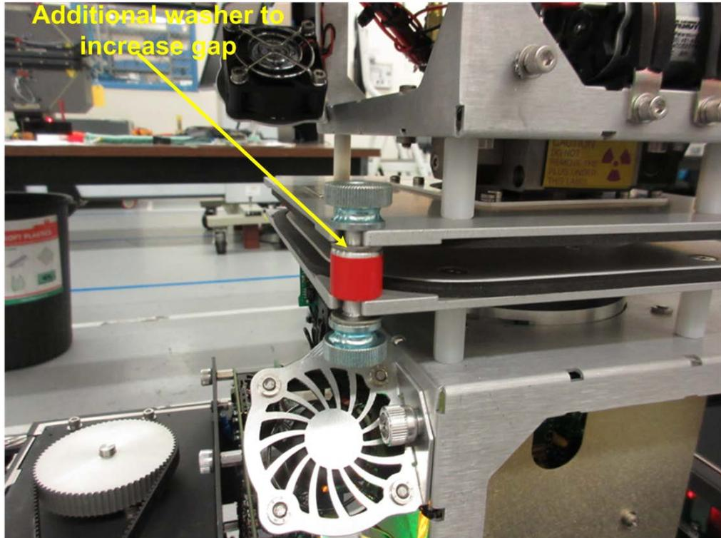
**Figure 8-93: Add additional washer in gap to further separate heads.**
