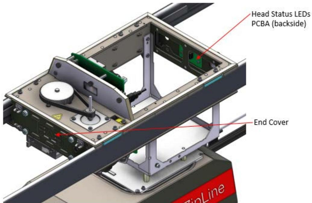
**Figure 8-37: Upper measurement module with head covers removed. One of two head status LED PCBA's is visible**
