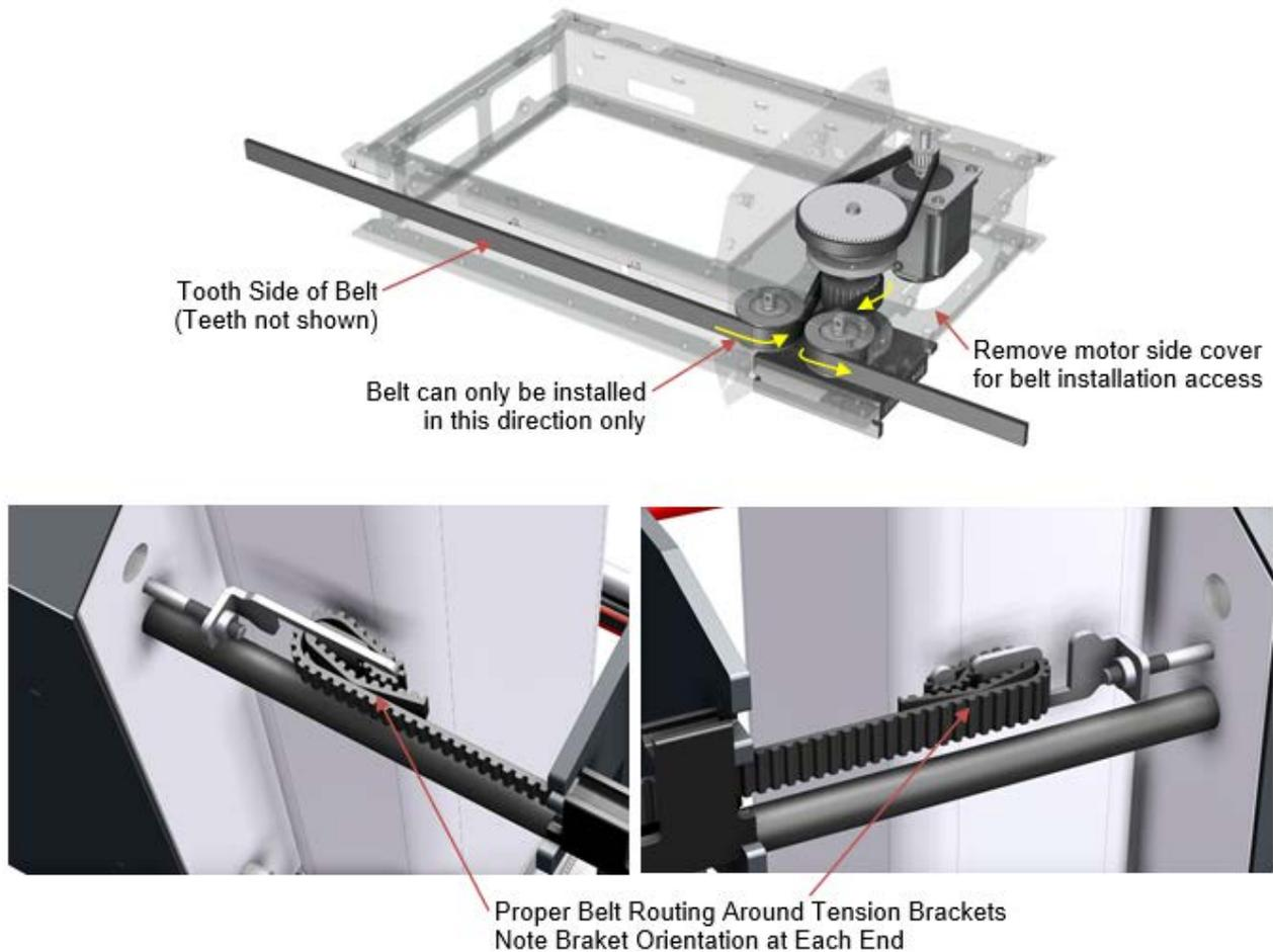
**Figure 6-4: Scanner Belt Routing Through Head and Tension Brackets**
