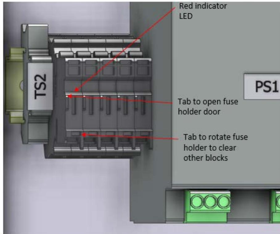
**Figure 8-21: Main features of the fuse block holder**
