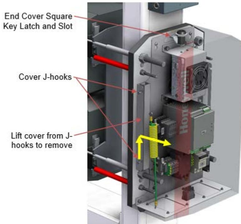
**Figure 6-5: Scanner End Cover Latch and Removal**
