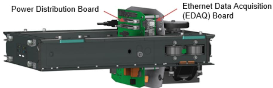
**Figure 6-15: Power Distribution Board**
