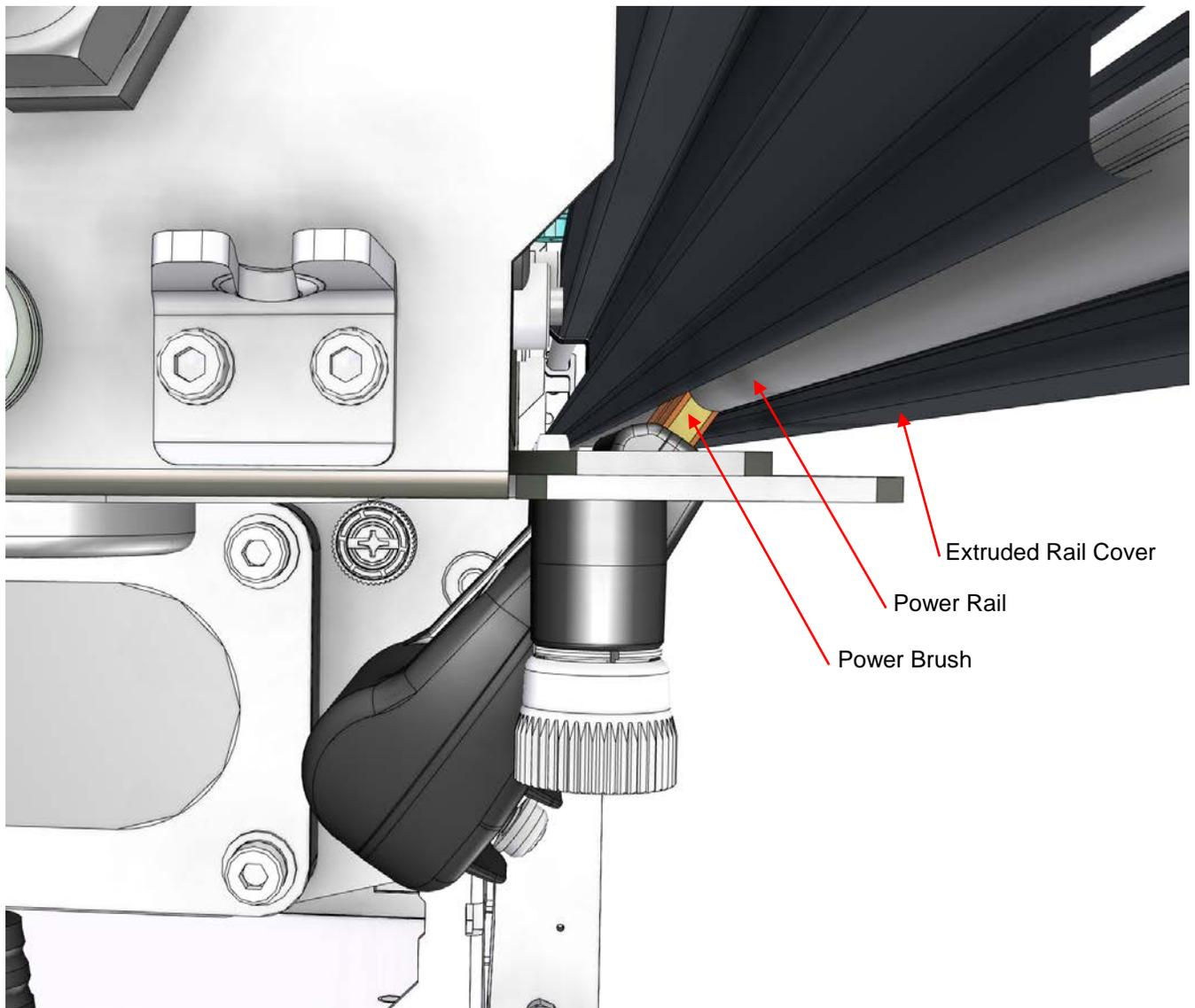
**Figure 8-33: Power Brush Alignment**
