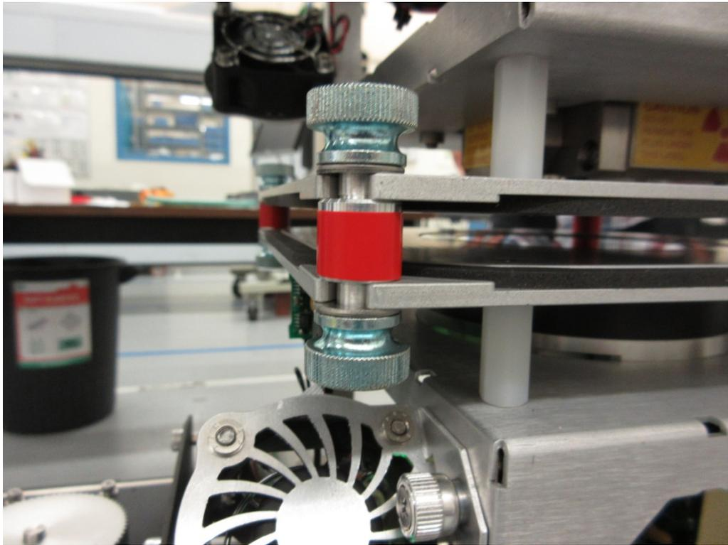
**Figure 5-17: Gap spacers maintain an exact 10mm alignment between heads**
