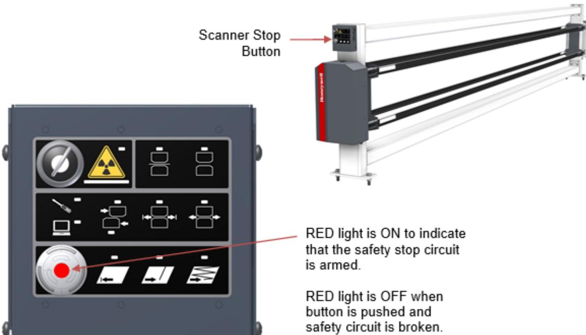
**Figure 2-12: Scanner Stop Button**
