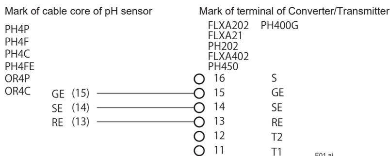
Note: Since RTD is not available, there is no wire connection to Converter/Transmitter 11 (T1) or 12 (T2).
