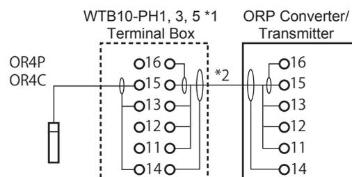
\*1: Terminal box is used only where pH/ORP transmitter is installed remotely from pH or ORP sensor (normally not needed). Refer to Table 2 for WTB10 type.
