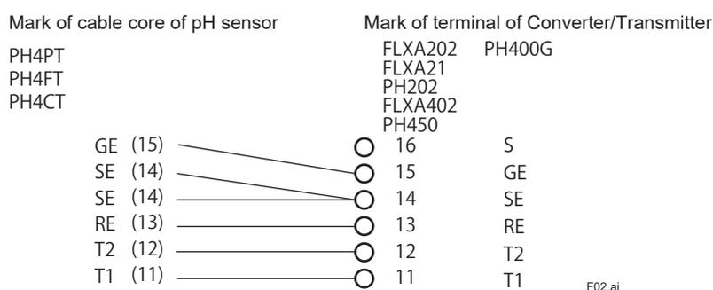
Note: 2 cable cores of pH sensor should be connected to the terminal of Converter/Transmitter 14 (SE).
