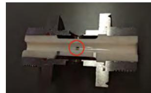
Ceramic liner tube with platinum-alumina cermet electrode (Mirror finished)
