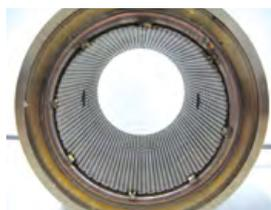
Structure of metal retaining plate for PFA liner
