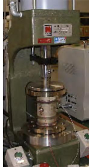
Testing with an Helium-leakage detector
