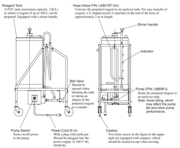
Figure 1 RC401G-C Reagent Tank Unit Components
