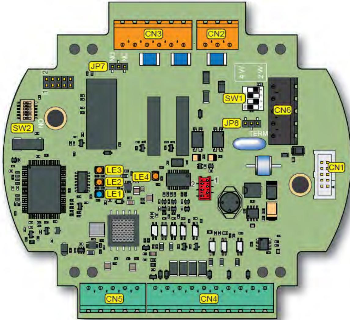
FIGURE 3-14 CAN-ADD-BLEND component location
