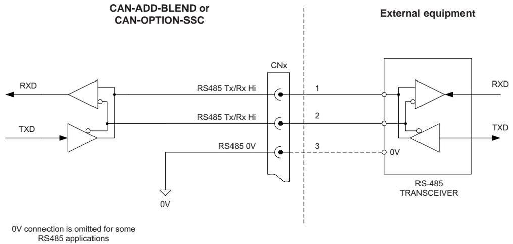
FIGURE 3-33 RS Communication 2-Wire connections
