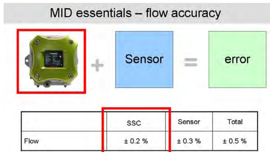
FIGURE 3-2 Component-level requirements (flow accuracy)
