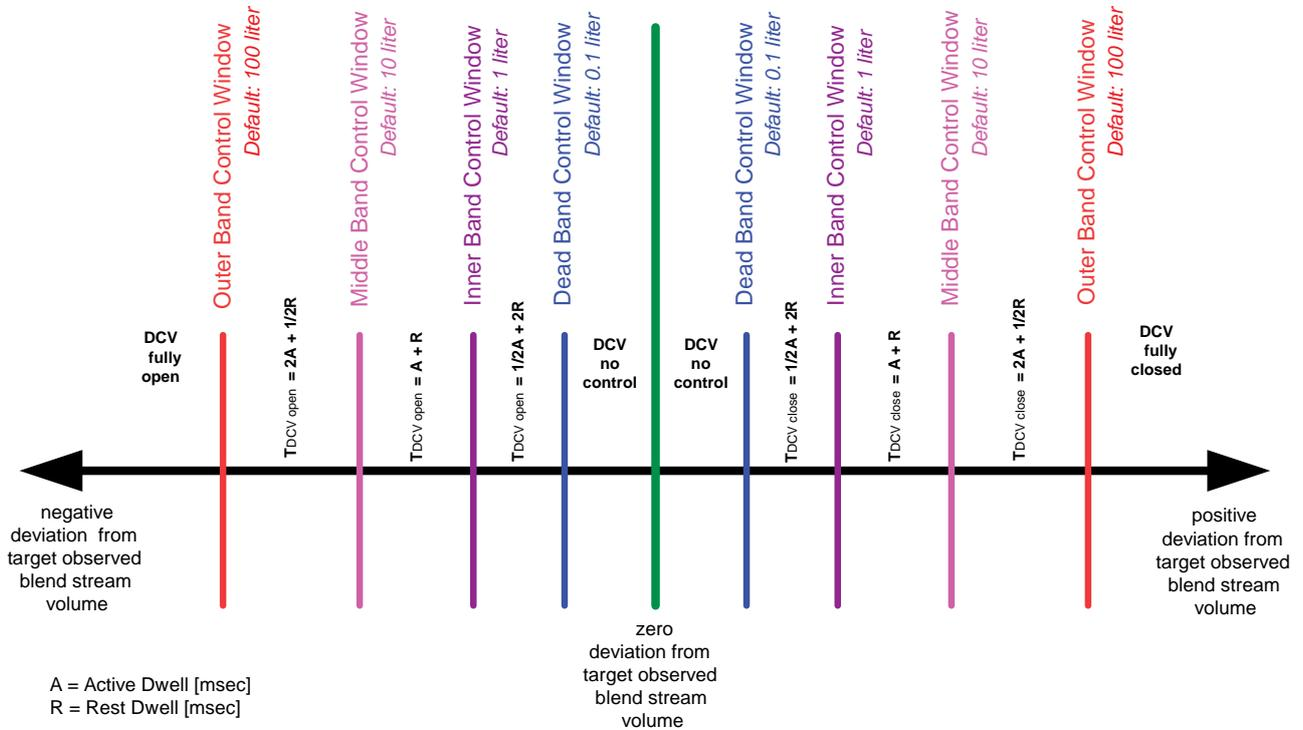
FIGURE 5-10 Visualization of the control windows
