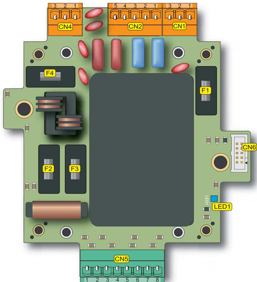
FIGURE 3-18 CAN-PSF-SSC component location
