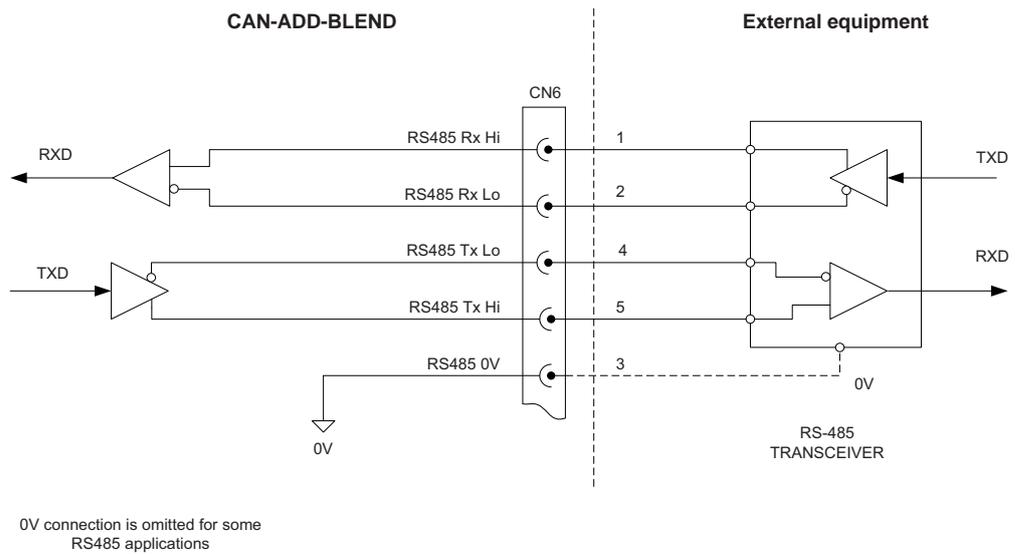
FIGURE 3-34 RS Communication 4-Wire connections (CAN-ADD-BLEND only)
