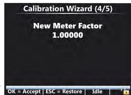
*NOTE: In case <ESC> is selected, the old meter factor is restored.*
