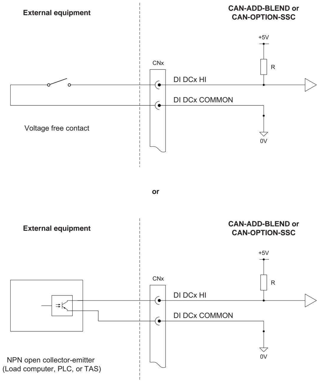
FIGURE 3-23 Digital Input DC connections
