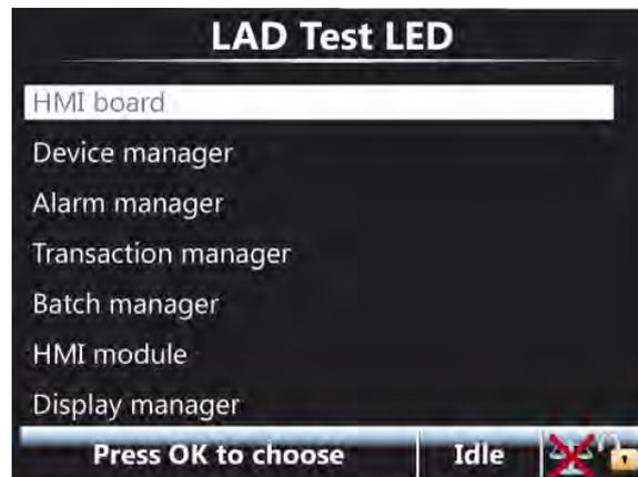
*NOTE: Test LED functions are inactive while retrieving other records from the LAD.*
