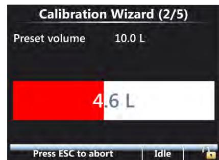
→ Enter the actual measured volume (calibrated vessel).
