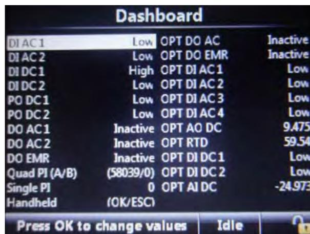
To change the value from **Inactive** to **Active** or vice versa for an output function (DO, DO EMR, AO, or PO), select the function and then select <OK>.
