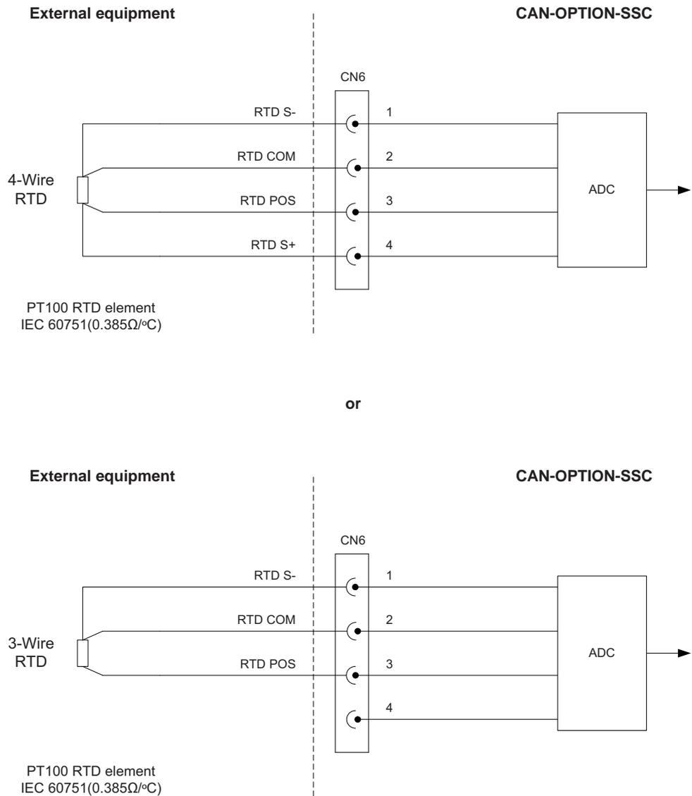
FIGURE 3-27 Resistance Temperature Detector connections
