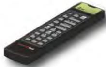
The Fusion4 IR Controller uses infrared (IR) signals to transmit ASCII characters to the SSC-B. This allows the operator to make adjustments in programming without removing the cover of the explosion-proof enclosure on-site.
