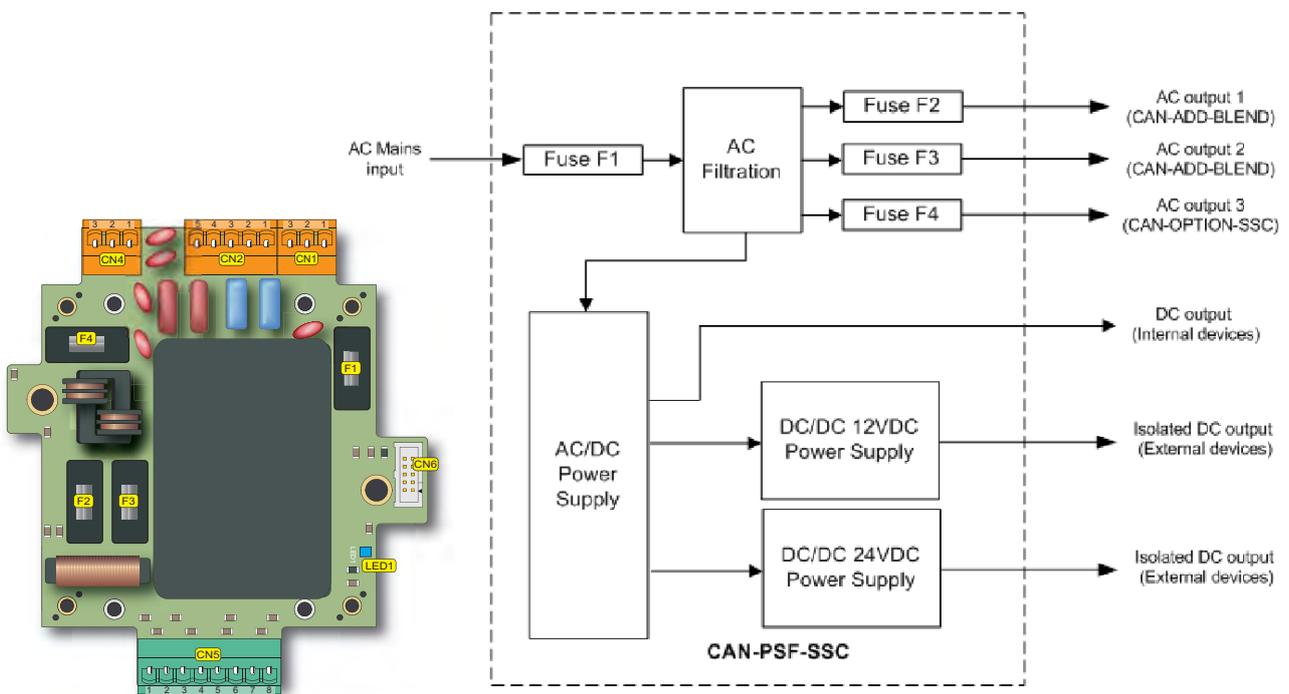
FIGURE 3-17 CAN-PSF-SSC functions (right) and physical layout (left)
