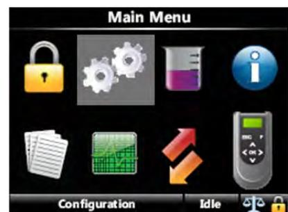
Now you can select a specific entity, for example, [Blend rate 1 permissive], [Pump feedback], and so on, and link it to a specific I/O function, for example, to <DI AC 1> (Digital Input AC<sup>1</sup>, number 1), <DO EMR> (Digital Output Electromechanical Relay), and so on.
