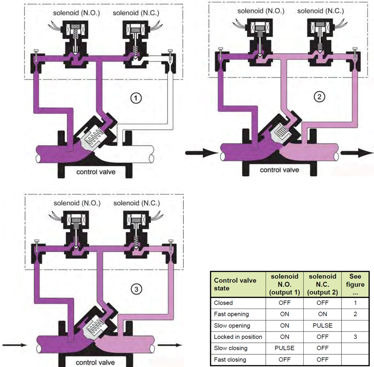
FIGURE 5-11 Blend stream control principle
