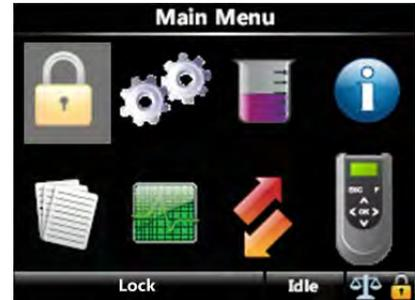
The "lock status" is shown at the status bar in the bottom right corner (padlock). See the following screen.
