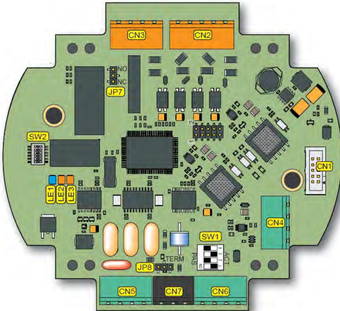
FIGURE 3-16 CAN-OPTION-SSC component location
