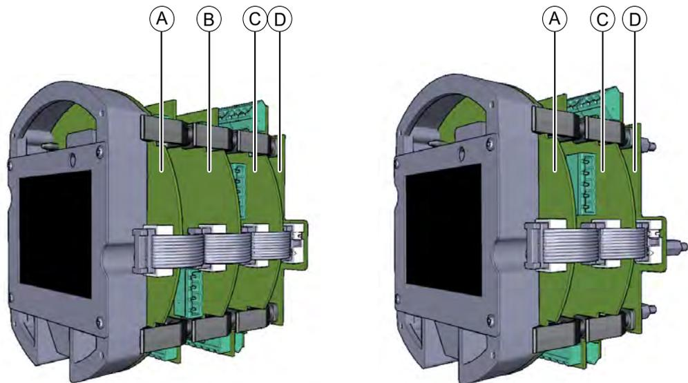
FIGURE 4-5 Full-configuration SSC-B (left) and 3-PCBs configuration (right)
