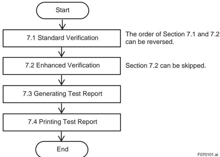
Figure 7.1.1 General Procedure of Verification
