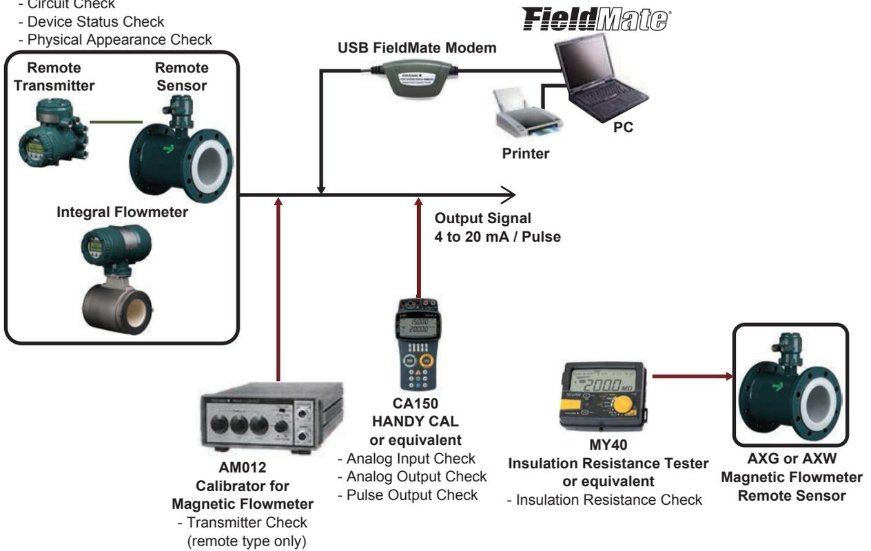
Figure 2.1.1 System Configuration
