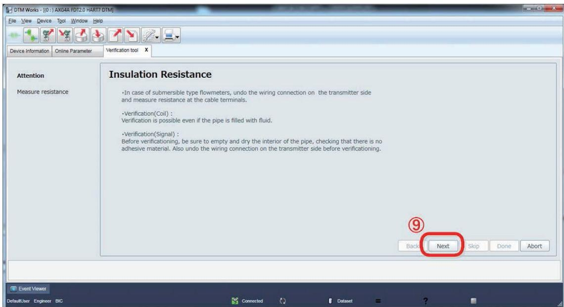
Figure 7.2.47 Continuing Insulation Resistance Check
