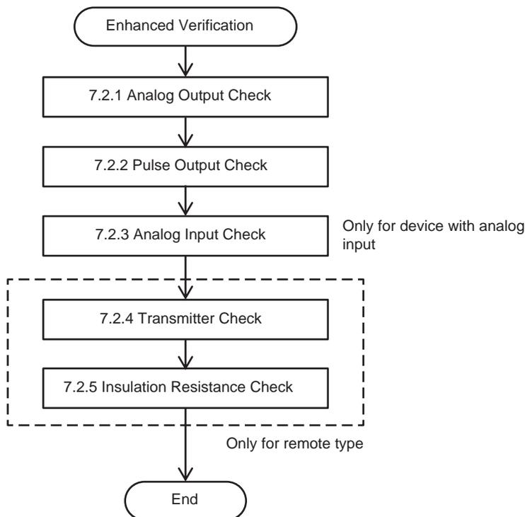
Figure 7.2.1 Procedure of Enhanced VF
