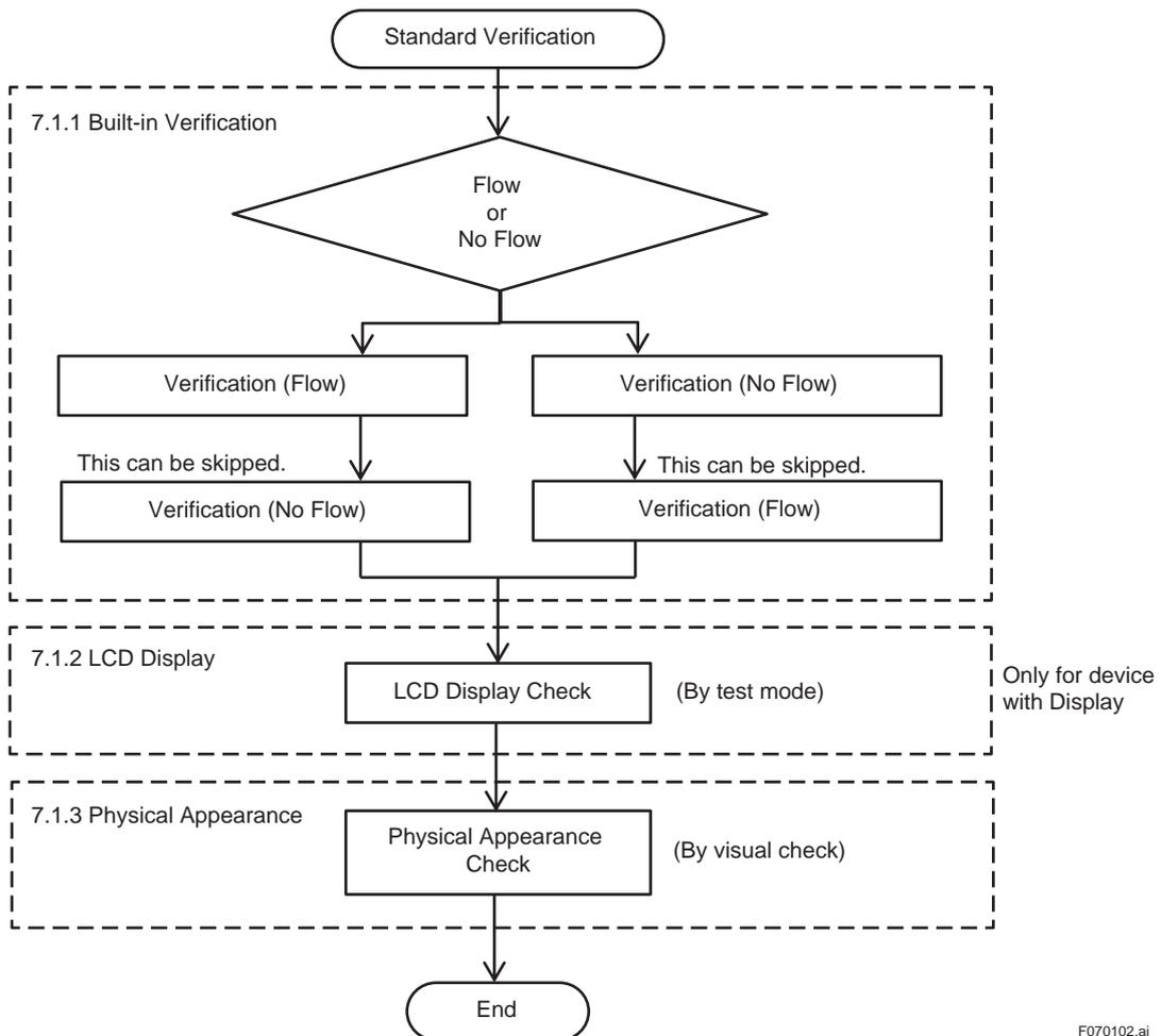
Figure 7.1.2 Procedure of Standard Verification
