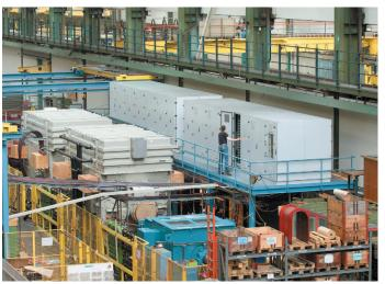
Back-to-back test 48 MW / 3,500 rpm
