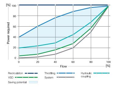
Power consumption for various pump control methods
