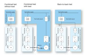
Illustration of extended test layouts
