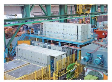
Back-to-back test 8 MW / 3,600 rpm
