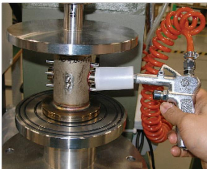
Testing with an Helium-leakage detector
