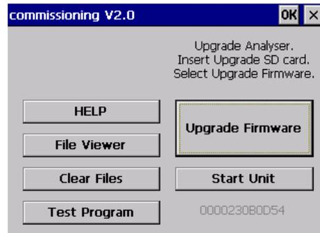
12. To upgrade the existing system software, press the **↵** key to start the process. The software is transferred to the analyzer in sections.
