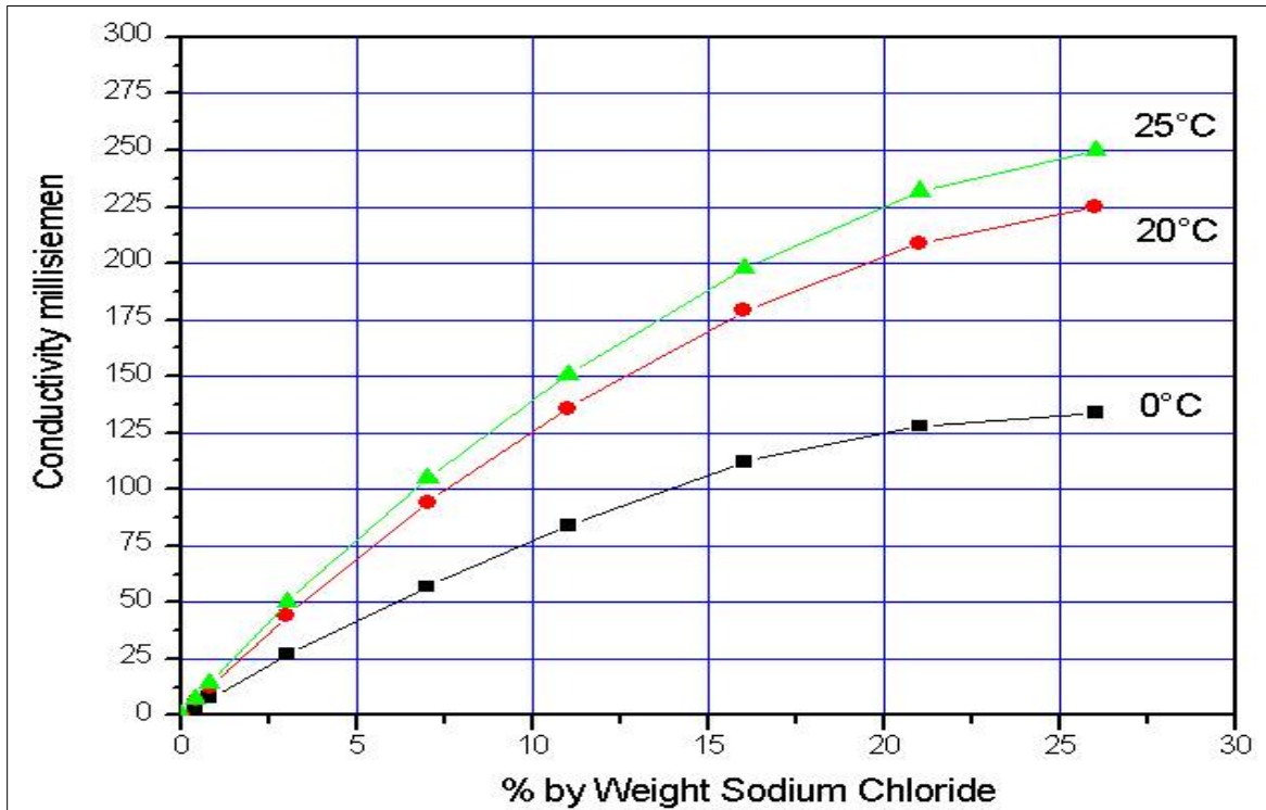
Illustration 24: NaCl conductivity vs. percent by weight NaCl
