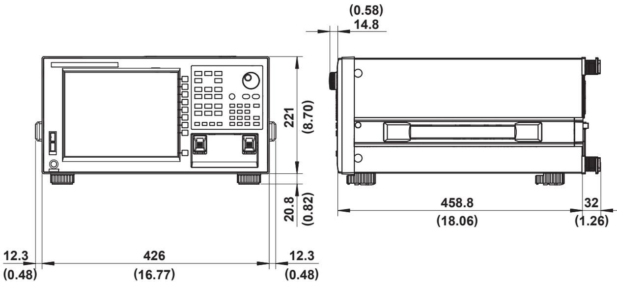
If not specified, the tolerance is  $\pm 3\%$ . However, in cases of less than 10 mm, the tolerance is  $\pm 0.3$  mm.
