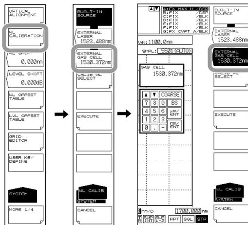
**Using the Instrument's Internal Calibration Wavelength Value**
