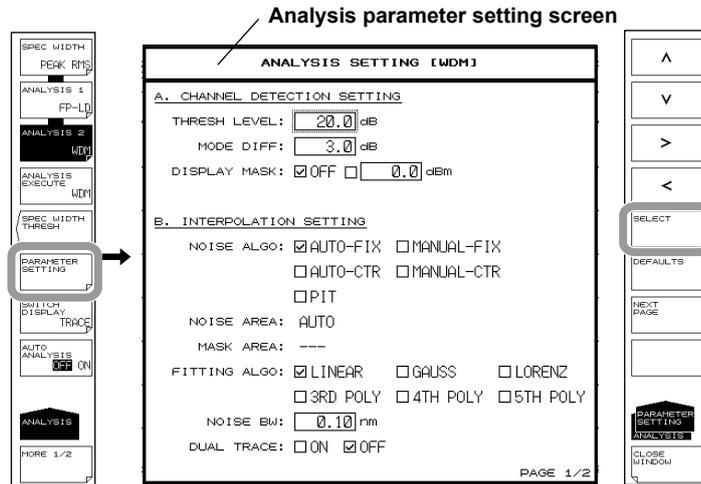
6. Press the **CLOSE WINDOW** soft key. The WDM analysis parameter setting screen closes, and the soft key menu returns to the previous stage.
