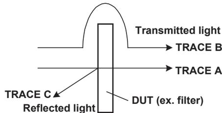
The value of k is an absorption coefficient which is used in determining the DUT reflectivity and transmission efficiency. Different algorithms are used depending on whether transmission efficiency or reflectivity is estimated, so the k value also varies accordingly.
