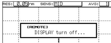
To keep the display turned ON, use a remote command, or press LOCAL to switch the instrument from remote to local mode.
