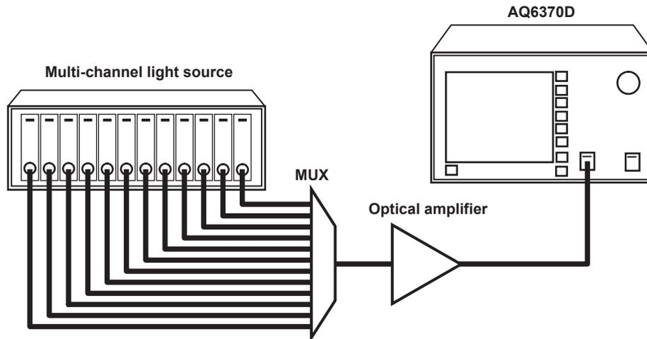
Measure the WDM signal light and write the waveform to the active trace.
