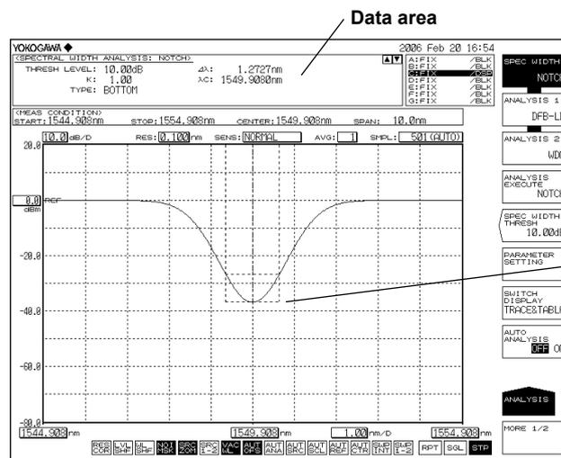
Analyzes the waveform with the minimum level value as a reference.
