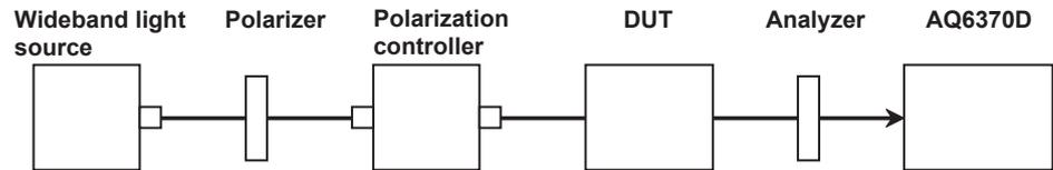
1. Enter measurement conditions so that the entire wavelength range of the wideband light source is measured. Set the resolution to about 0.050 nm.
