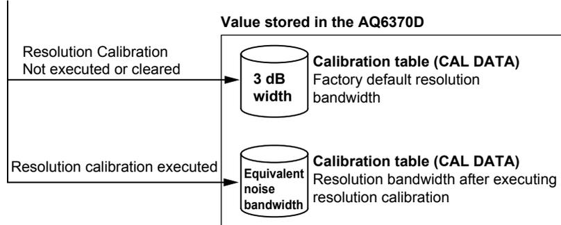
The analysis algorithm other than EDFA-NF uses the value stored in the AQ6370D.
