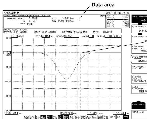
Analyzes the waveform with the maximum level value as a reference.
