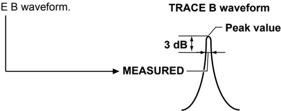
If the RES BW parameter is set to “CAL DATA,” the resolution bandwidth stored in the AQ6370D is used.
