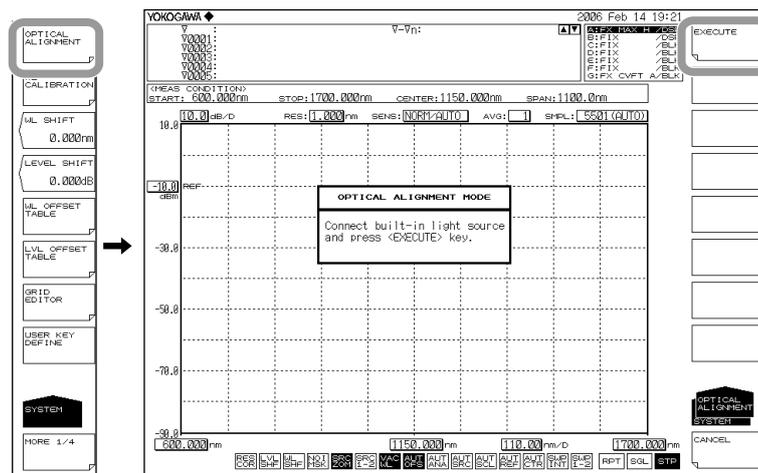
5. Press the **EXECUTE** soft key. Alignment adjustment is automatically executed. Adjustment finishes a few minutes thereafter, and you are returned to the original screen.
