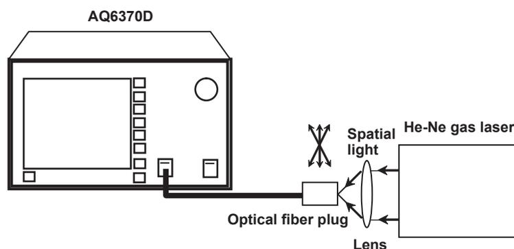
The sweep width is set to 0 nm, the center wavelength is fixed, and measurement of the single-wavelength light only is taken. Finely adjust the optical fiber plug while observing the displayed waveform so as to set the light source input level to the peak.
