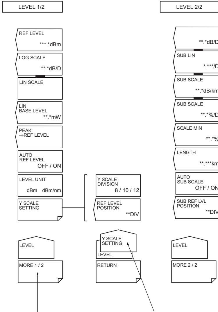
The LEVEL soft key menu is split into two parts. This key switches between the menus. In addition, in some cases this may change to a function that closes the window. For example, when the MORE 1/2 soft key is pressed, the menu changes to the LEVEL 2/2 soft key menu, and the key display changes to MORE 2/2.
