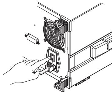
3. Press the **POWER** switch on the front panel of the instrument. The color of the switch turns from orange to green. The operating system starts up, and initialization of the instrument begins.
