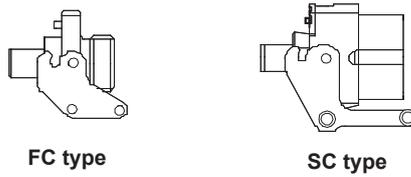
The optical input connector adapter (AQ9447) comes in the following two types.
