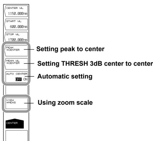
Also, you can set the wavelength of the moving marker placed on the measured waveform as the center wavelength or center frequency.
