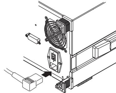
2. Turn ON the **MAIN POWER** switch on the rear panel of the instrument. The **POWER** switch on the front panel of the instrument lights orange.
