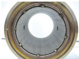
Structure of metal retaining plate for PFA liner
