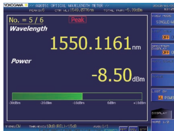
The horizontal bar graph easily identifies the optical power variation and flatness of the signal.
