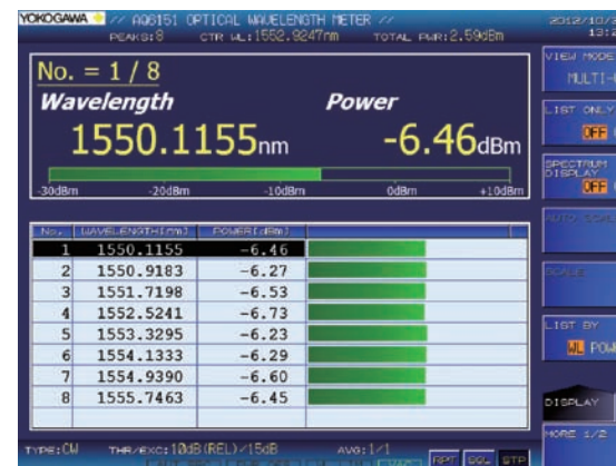
The horizontal bar graph easily identifies the optical power variation and flatness of the signal.
