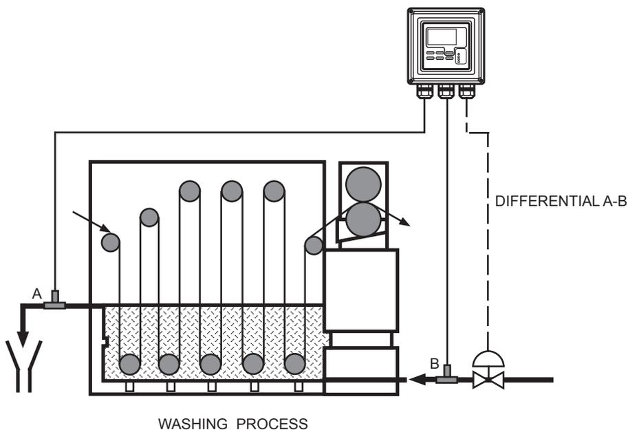
Fig. 10.3 Differential output water flow to optimize washing efficiency.
