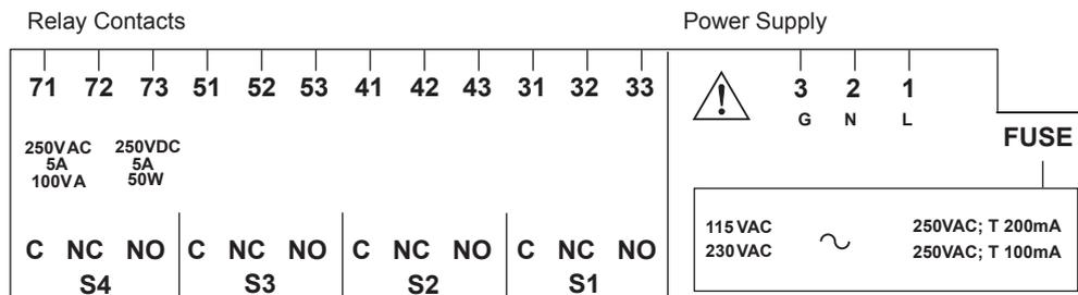
Figure 3.8 Input and output connections
