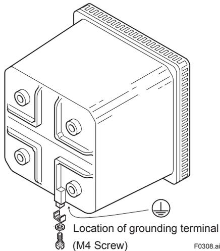
**Figure 3.9** Grounding the housing
