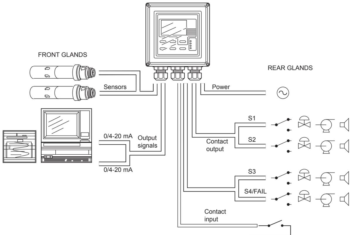
Figure 3.7 System configuration
