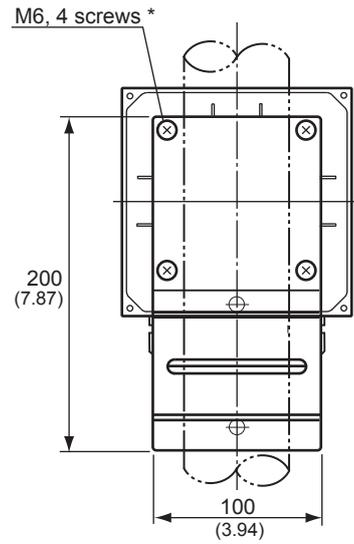
Example of bracket used for wall mounting
