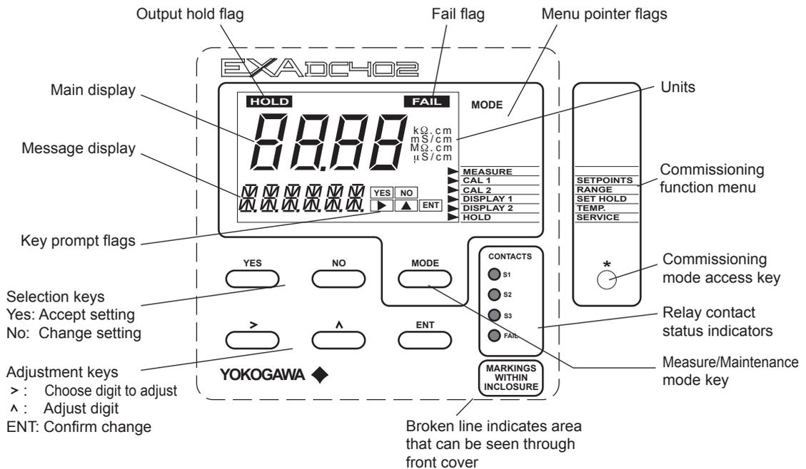
Figure 4.1 DC402G operator interface
