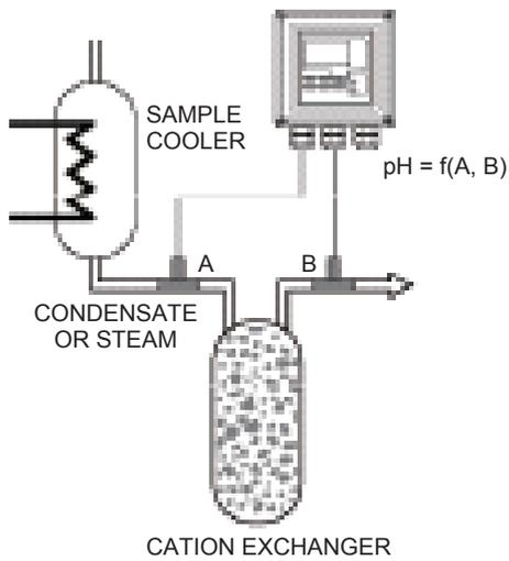
Fig. 10.5 pH output as a function of two conductivity values before and after the cation exchanger.
