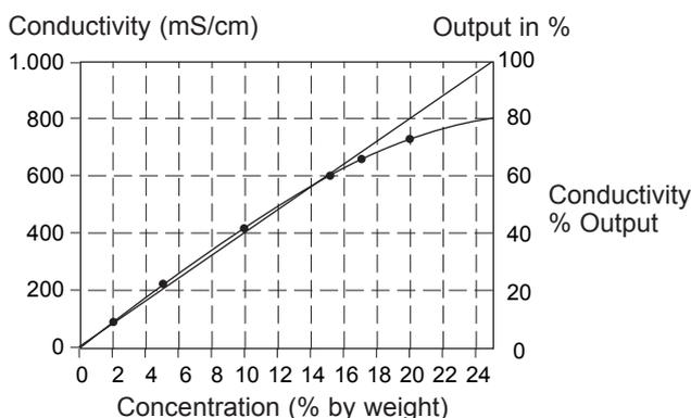
Fig. 5.1 Linearization of output Example: 0-25% Sulfuric acid
