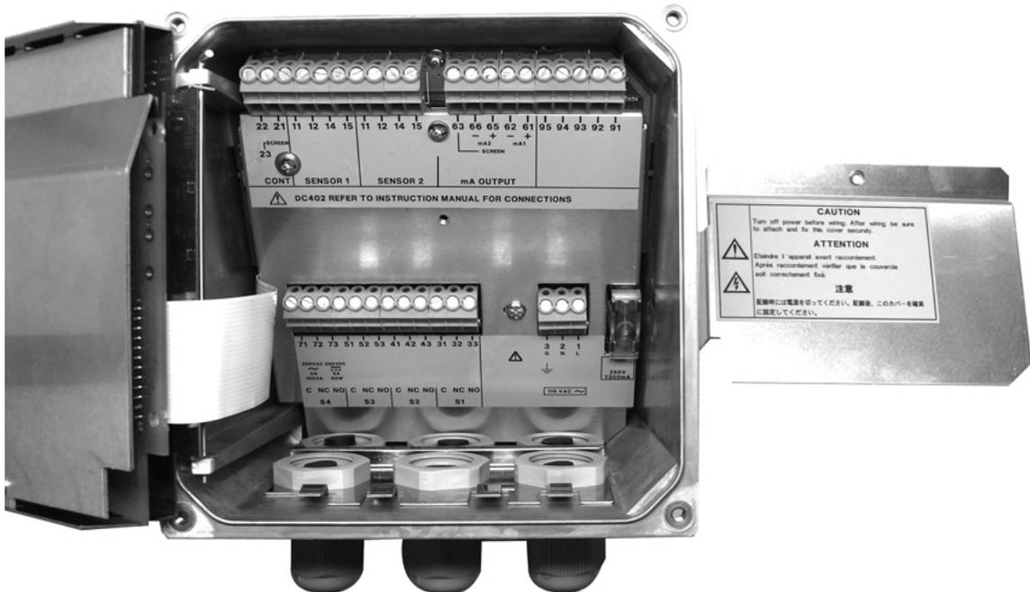
Figure 3.4 Internal view of DC402G wiring compartment
