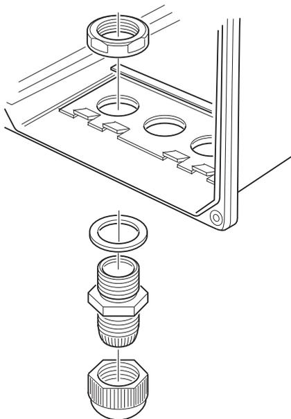
Figure 3.13 Sensor cable connections
