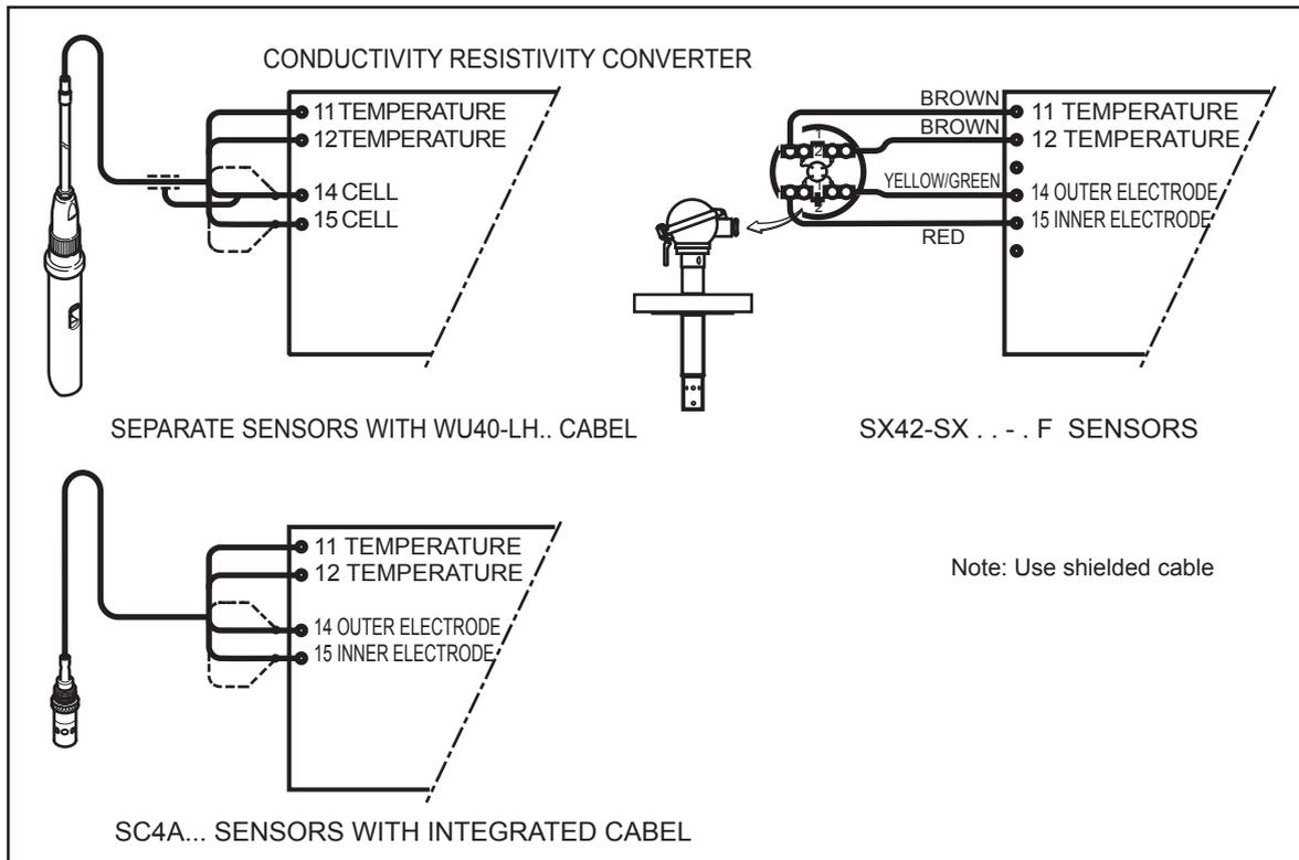
Figure 3.10 Sensor wiring diagrams
