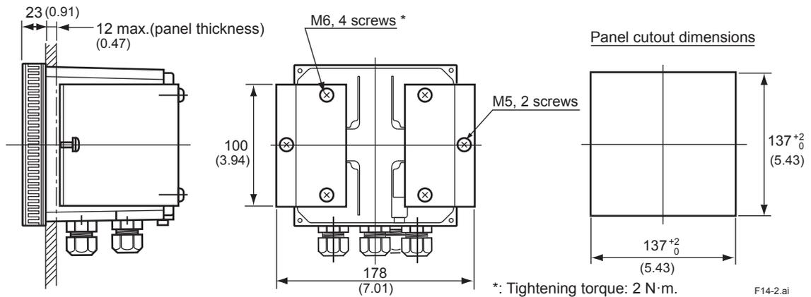
Figure 3.2 Panel mounting diagram (Option Code: /PM)
