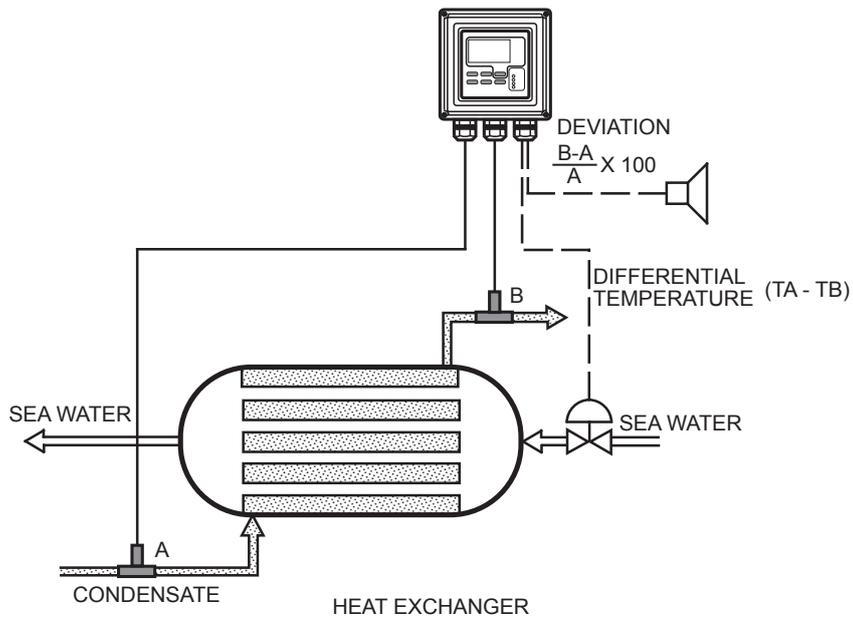
Fig. 10.4 Deviation output alarms directly after leakage in the heat exchanger.
