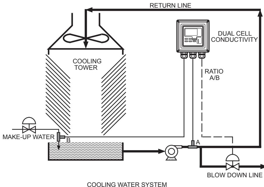
Fig. 10.2 Ratio output controls blow-down of cooling tower based on concentration factor.
