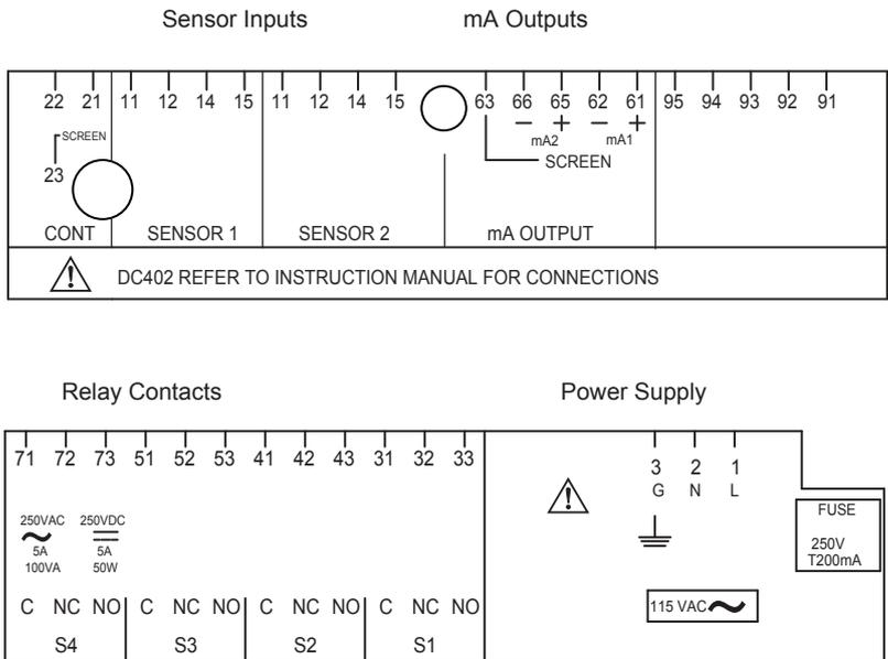
Figure 3.12 Terminal identification labels example
