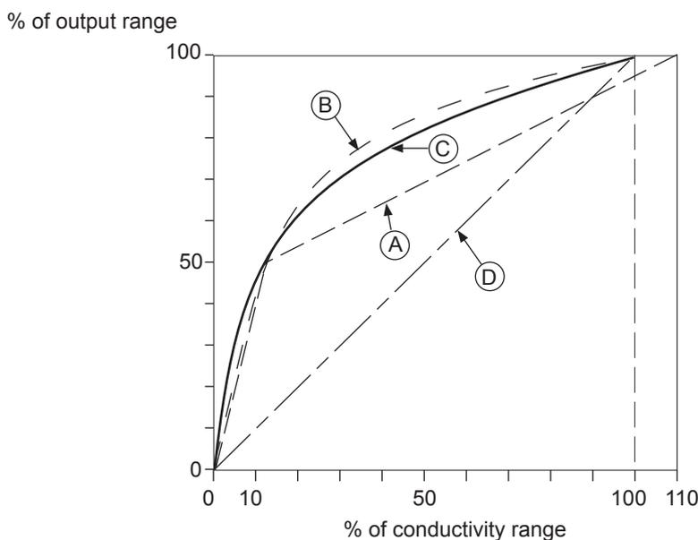
Fig. 5.2 Percentage of mA-output range versus percentage of conductivity range
