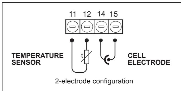
Figure 3.11 Connection diagram for other sensors
