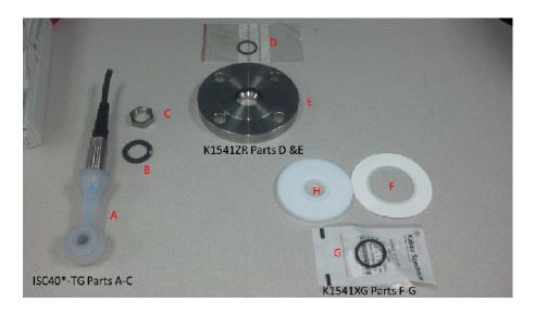
First remove parts B & C. Then install parts F,G,& H from the K1541XG sealing ring kit. Then install the flange and then part C, the nut from the ISC40\*-TG sensor as shown below.
