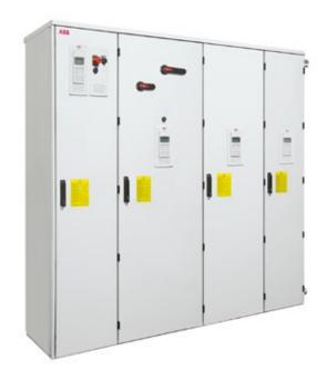
ABB's multidrives are built from ABB industrial drive modules connected to a common DC bus. This enables a single power entry and common braking resources for several drives.
