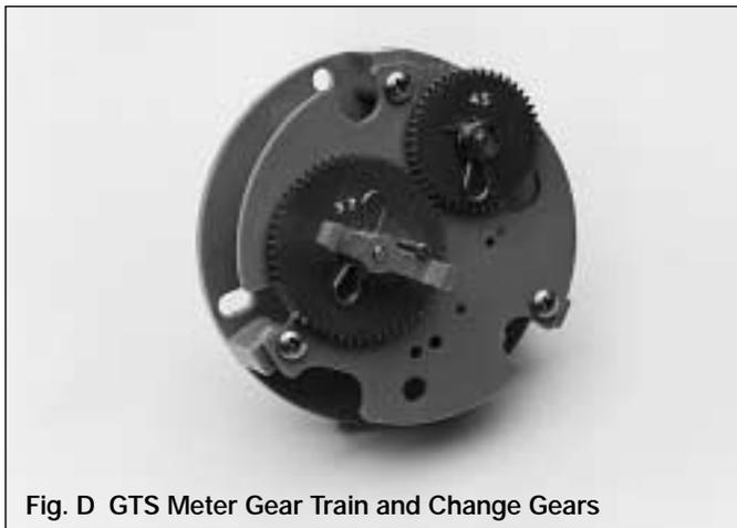
Fig. D GTS Meter Gear Train and Change Gears
