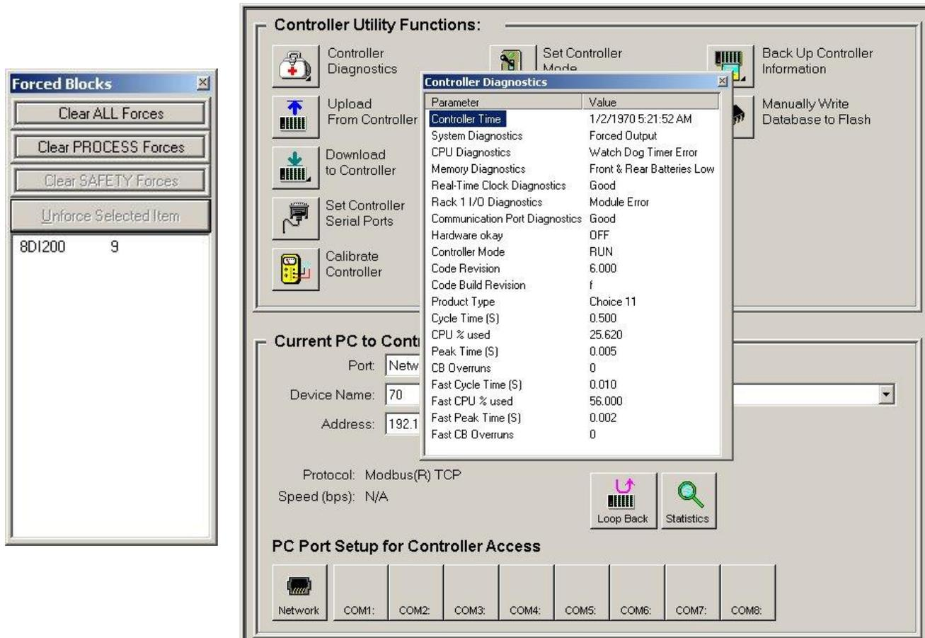
Figure 7 - Forced blocks window (left), Diagnostic monitoring window
