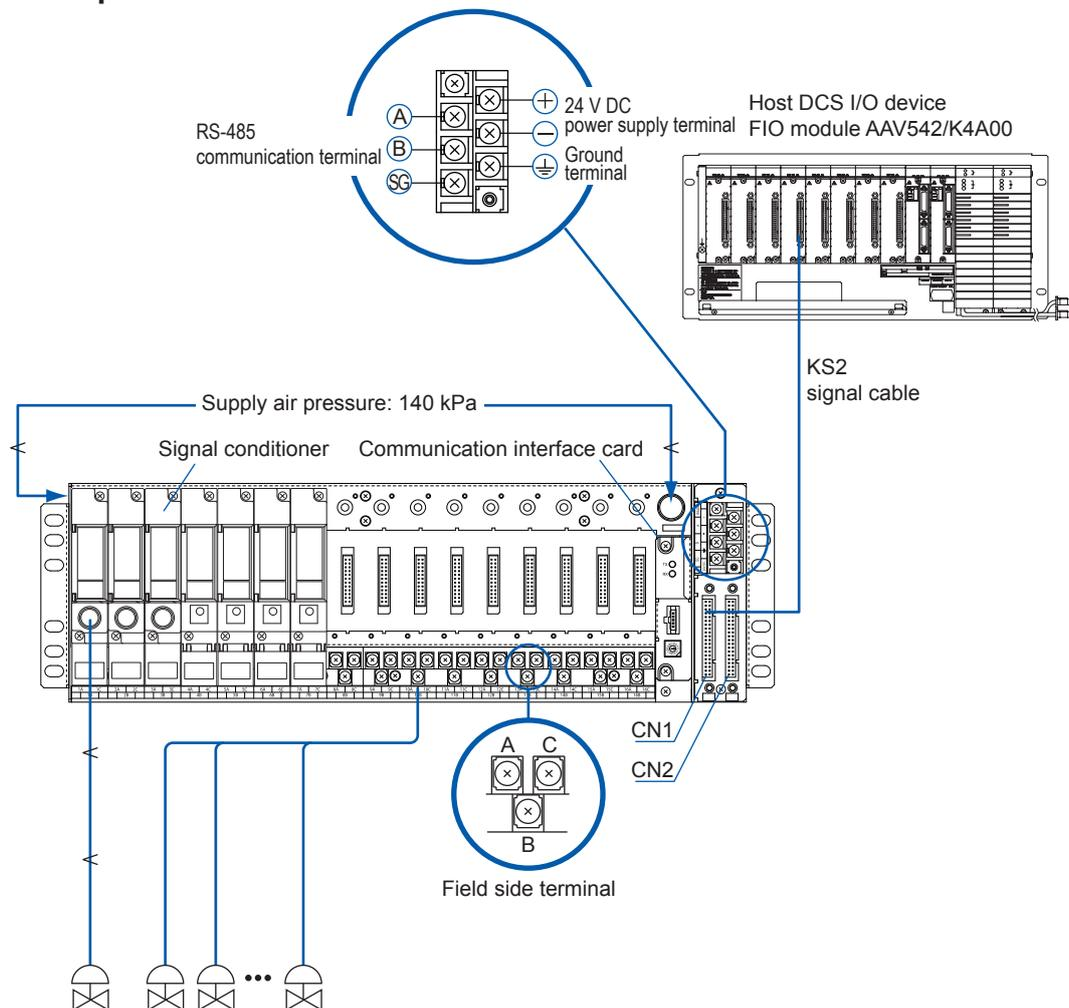
► The figure above is the example of connection to the multipoint analog output module. For the signal conditioners mountable to the nest, see the section 1.3 in this manual.
