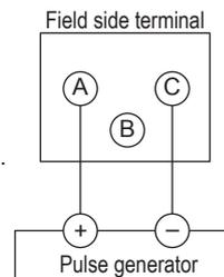
(Note) "B" is used in cases where the power is supplied from a converter. When using two-wire type, B is the power supply, and A is the signal. When using three-wire type, B is the power supply, A is "+", and C is "-".
