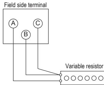
(Note) The wiring resistance should be equal.
