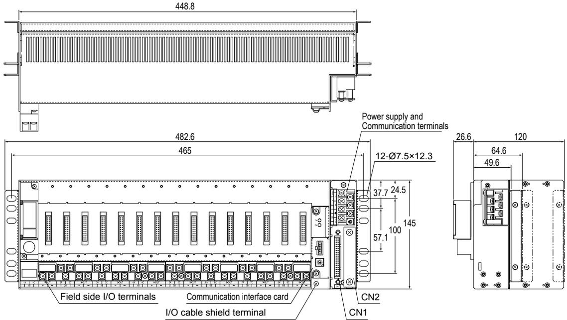
**DMP Nest for Control Input/Output (Electric, P/E, and E/P Mixed Mounting Type)**
