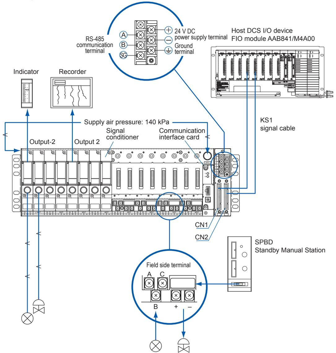
► The figure above is the example of connection to the multipoint analog I/O module. For the signal conditioners mountable to the nest, see the section 1.3 in this manual.
