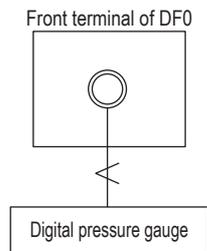
(Note) DF0 should be mounted directly to the nest without using DXT card.
