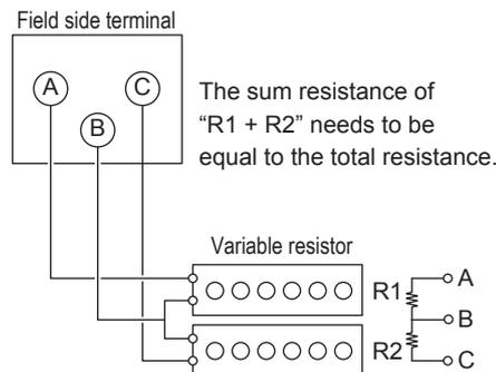
(Note) The wiring resistance should be equal.
