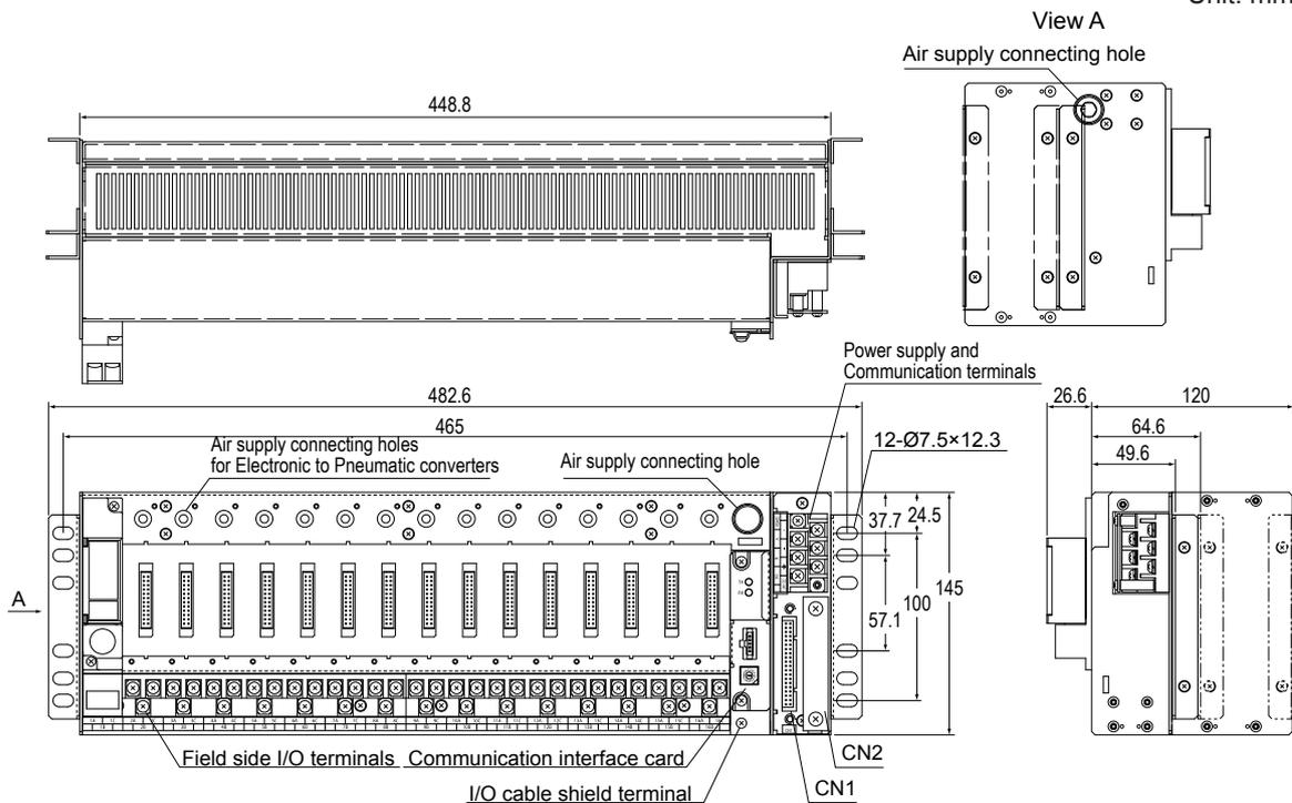
**DME Nest for Control Input/Output (Electric, and P/E Mixed Mounting Type)**
