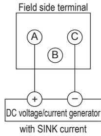
(Note) When not using each internal power supply of DA1, DA2, DA5 and DA7, C is "+", and B is "-".
