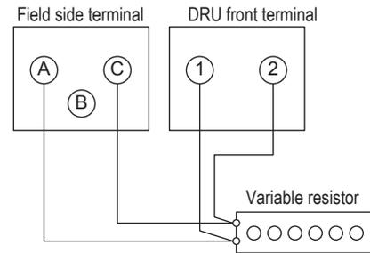
(Note) The wiring resistance should be equal.
