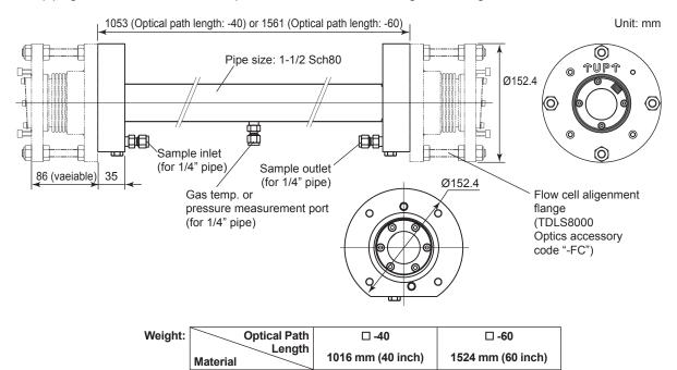
Weight of the Flow cell aligenment flange (TDLS8000 Optics accessory code "-FC"): Approx. 5 kg/pc
