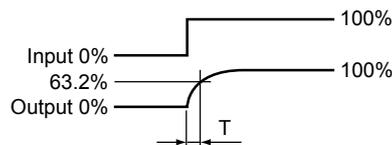
Setting range of time constant: 1.0 to 100.0 sec. (0.010 to 1.000 V); minimum unit is 0.1 sec.
