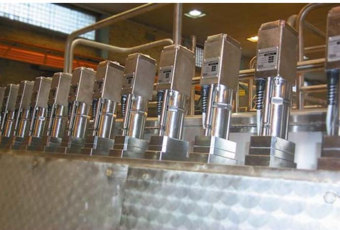
With Honeywell controls, the AutoSlice system improves CD basis weight profiles leading to improvements in moisture, caliper and coating profiles, as well as calendering, winding, converting and runnability.
