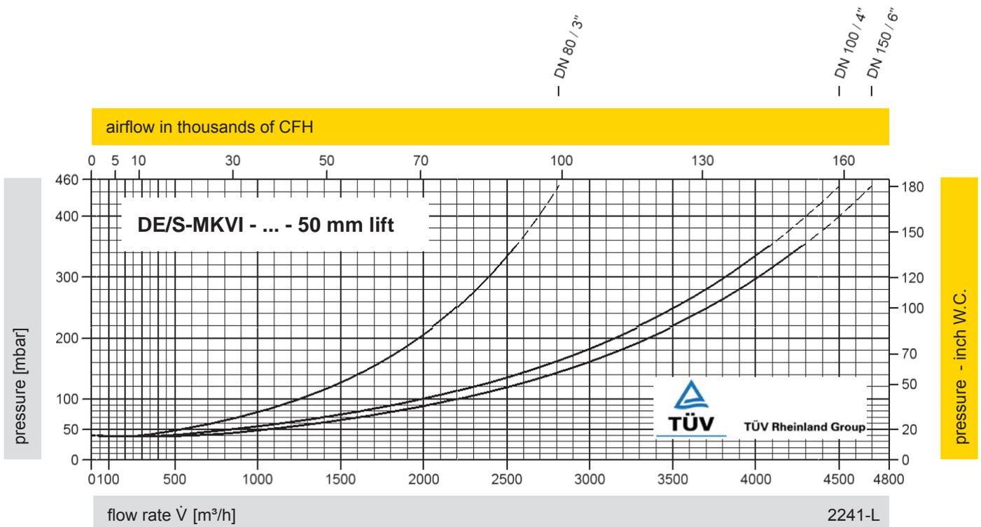
The flow capacity charts have been determined with a calibrated and TÜV certified flow capacity test rig. Volume flow  $\dot{V}$  in [m³/h] and CFH refer to the standard reference conditions of air ISO 6358 (20°C, 1bar). Conversion to other densities and temperatures refer to Technical Fundamentals.
