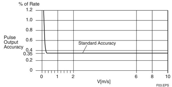
**Current Output “◇”:** Pulse output accuracy plus ±0.05% of Span
