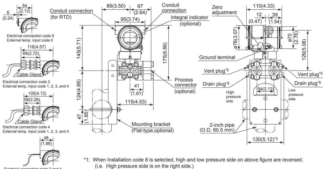
\*1: When Installation code 8 is selected, high and low pressure side on above figure are reversed.
