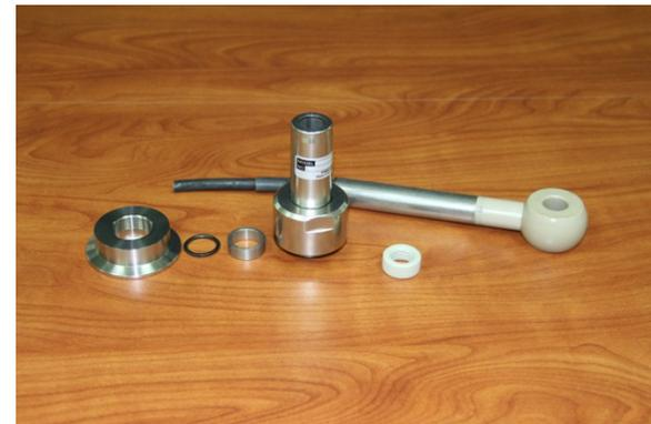
3. Slide the tri-clamp piece onto the ISC40G(S)-GS sensor, followed by the o-ring and then the metal sealing ring.
