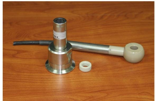
2. Unscrew the sanitary fitting pieces and locate the O-ring **(A)** and a metal sealing ring **(B)**.
