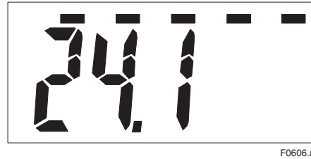
Figure 6.6 Display showing Confirm Connecting Status State
