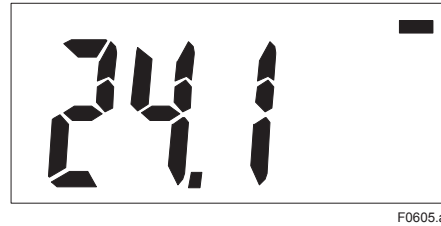
Figure 6.5 Display showing Ready and Pause State
