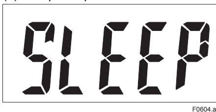
Figure 6.4 Display showing Deep Sleep State
