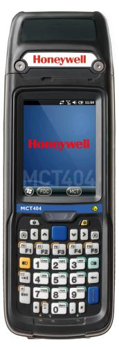
The MCT404 is compatible with Honeywell's PIE tool to configure Honeywell UDA2182 Analyzers and UDC controllers through it's IrDa port.
