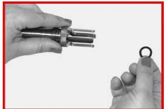
4. Insert the O-ring inside of the sensor tip as show in the image, until it seats in the O-ring groove.
