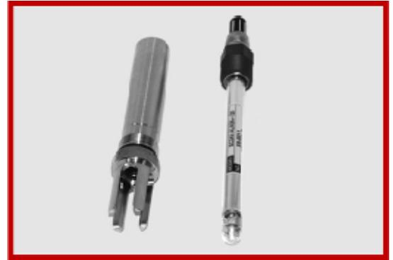
17. Slide the electrode into the protection tip and thread the PG13.5 connector in place.
