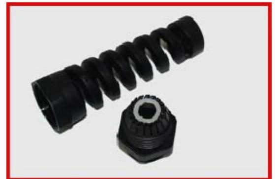
22. Thread the taped end of the cable thru the squeezing tube portion of the cable strain relief plastic piece. Then thread the taped end of the cable thru the plastic tube portions of the cable strain relief.
