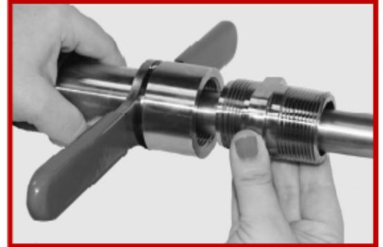
The side that contains a bevelled end on the inside has the Gas straight thread (**A**), where the side that is flushed has the NPT thread (**B**).
