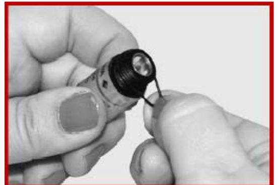
8. Place the electrode into the tip portion of the holder.
