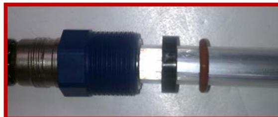
16. Set aside the metal tube that comes in the bag with the manual it will not be used. You will just be using the sensor tip from the PR10 holder and the electrode with the PG13.5 connection.
