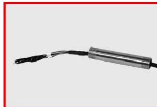
13. Once the cable is threaded thru the metal tube attach the cable to the sensor and screw the metal tube and the sensor tip together as seen here.
