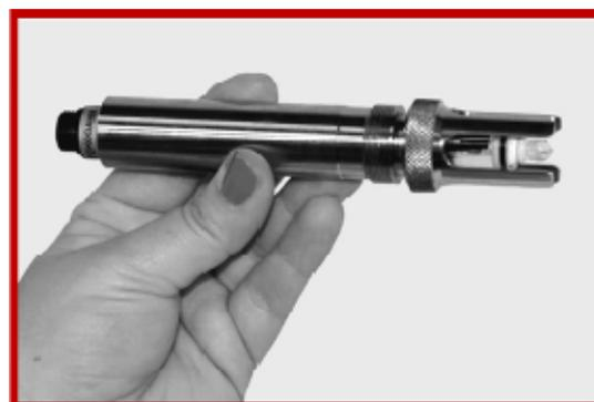
10. Take the electrode tip and the largest O-ring (A) that is provided in the bag with the Instruction manual, and place it on the protection tip below the threads and next to the knurled finger grip.
