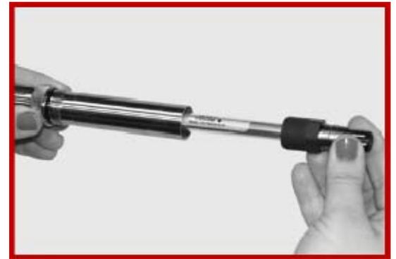
18. Once the electrode is tightened in place, take the largest O-ring (A) that is provided in the bag with the Instruction manual, and place it on the protection tip below the threads and next to the knurled finger grip.
