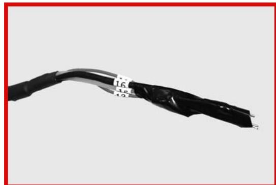
20. Attached the cable to the sensor and feed it thru the PR10 holder assembly. Insert the sensor tip, into the PR10 holder assembly thread it sealed.
