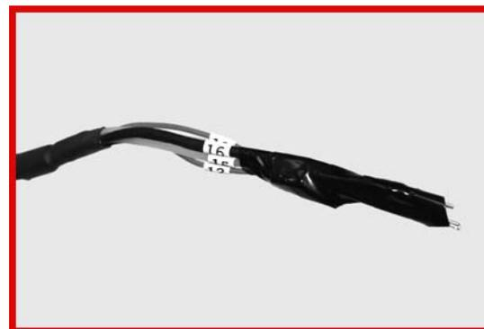
12. At this point take the taped end of the cable and feed it thru the back end of the metal tube provided in the bag with the manual, as shown in the images here.
