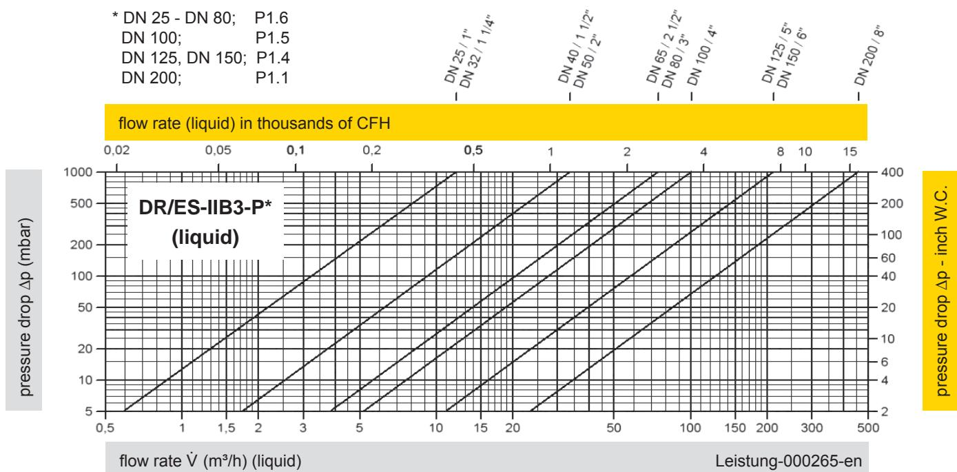
$$\text{Conversion: } \dot{V}_{\text{liquid}} = \dot{V}_{\text{water}} * \sqrt{\frac{\rho_{\text{water}}}{\rho_{\text{liquid}}}}$$
