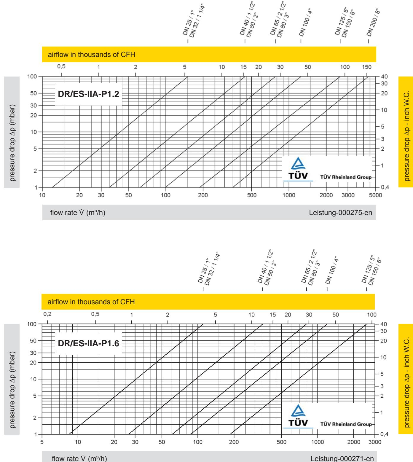
The flow capacity charts have been determined with a calibrated and TÜV certified flow capacity test rig.
