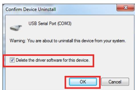
**Step 5** Right-click “USB Serial Converter” under “Universal Serial Bus controllers,” and click Uninstall.
