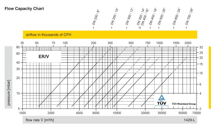
The flow capacity chart has been determined with a calibrated and  $T\ddot{U}V$  certified flow capacity test rig. Volume flow  $\dot{V}$  in [m³/h] and CFH refer to the standard reference conditions of air ISO 6358 (20°C, 1bar). Conversion to other densities and temperatures refer to Vol. 1: "Technical Fundamentals".
