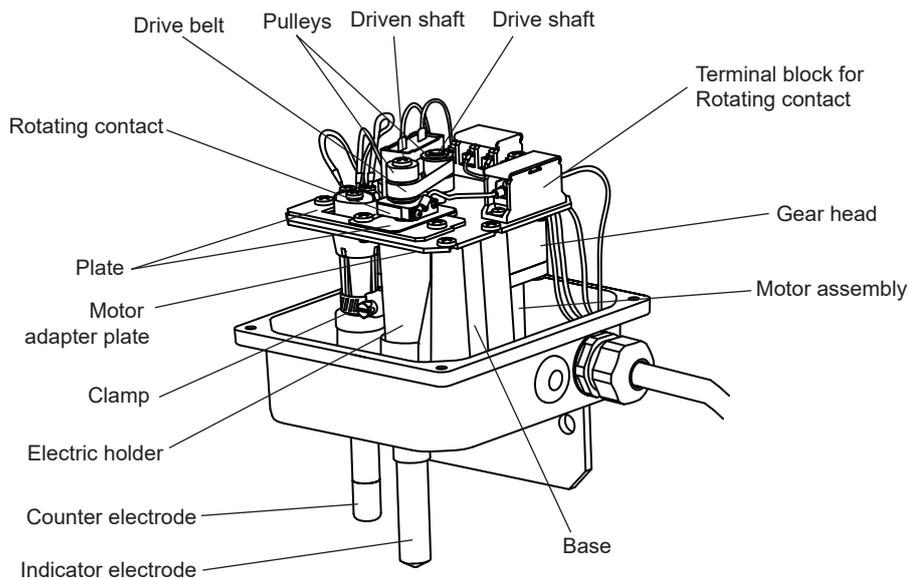
Figure 6.2 Electrode Mechanism Block
