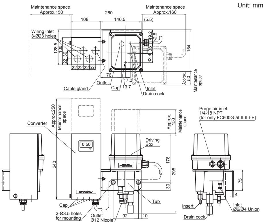
Figure 1.4 Model FC500G Free Available Chlorine Analyzer External Dimensions
