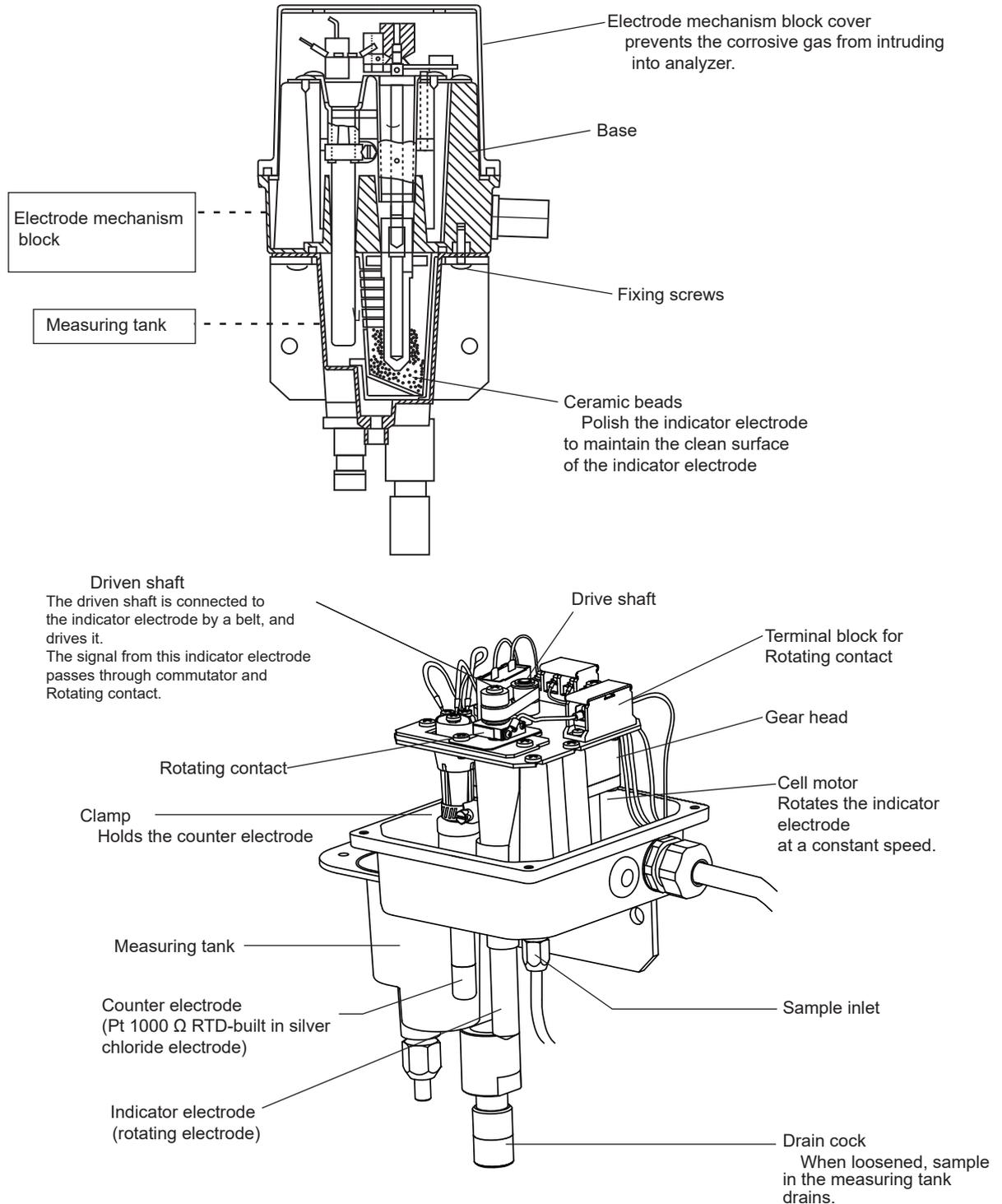
Figure 2.1 Component Names and Functions of the Detector
