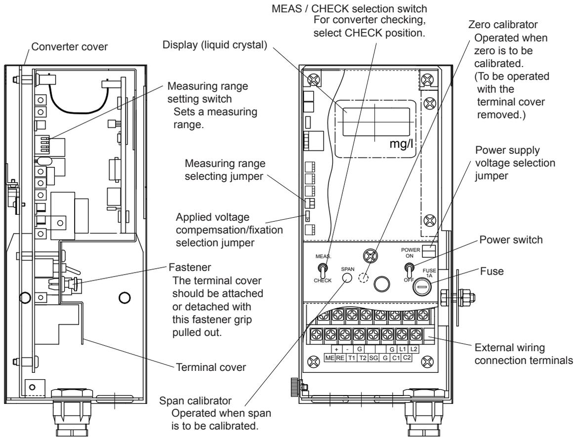
Figure 2.2 Converter Component Names and Their Functions
