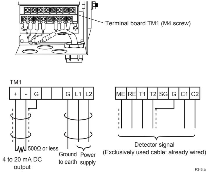
Note: Make grounding to earth (grounding resistance 100 Ω or less).
