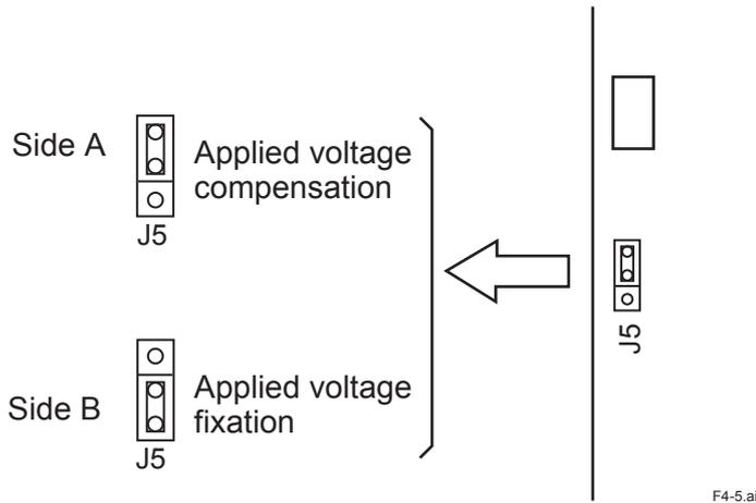
Figure 4.5 “Applied Voltage Compensation/Applied Voltage Fixation” Selection Jumper
