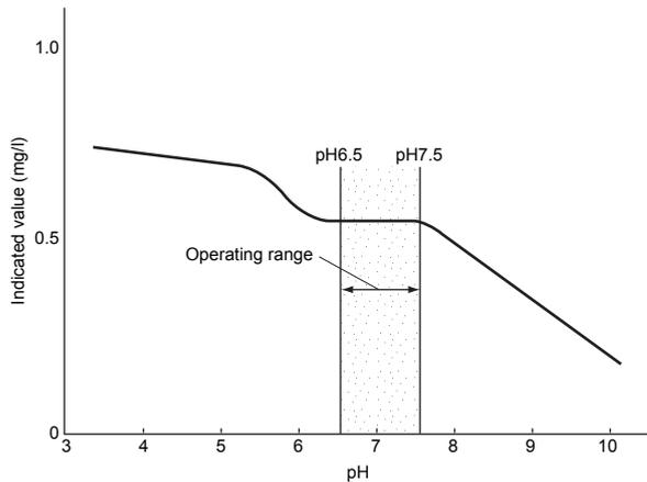
Figure 1.2 Sensitivity characteristics of diffusion current by pH value
