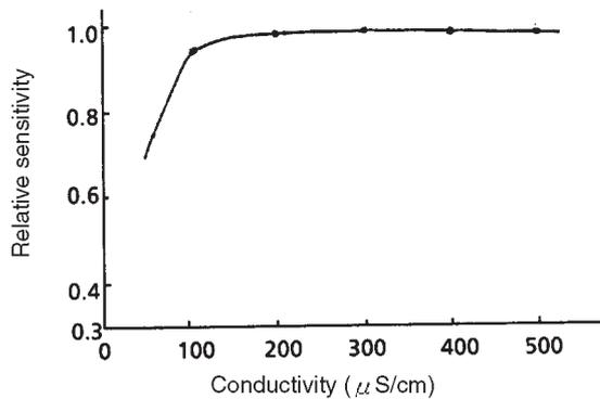
Figure 1.3 Sensitivity characteristics of diffusion current by conductivity
