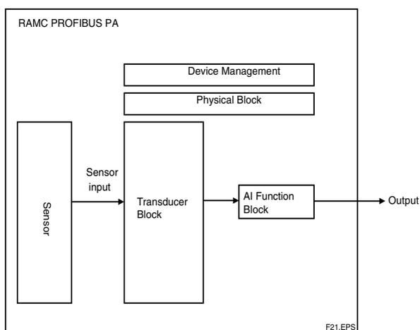
Figure 2.1 Logical Structure of Each Block
