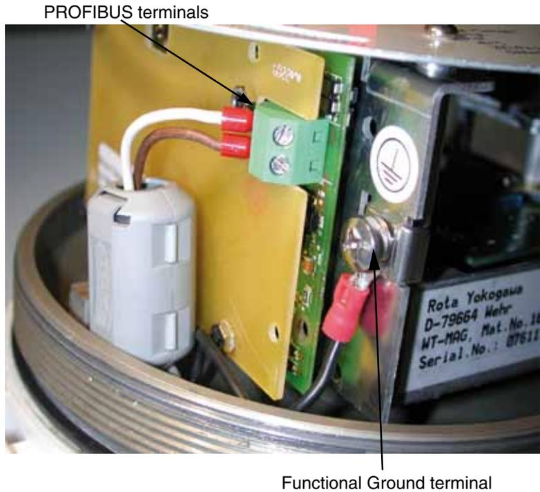
**Cable shield grounded only on bus- side**
