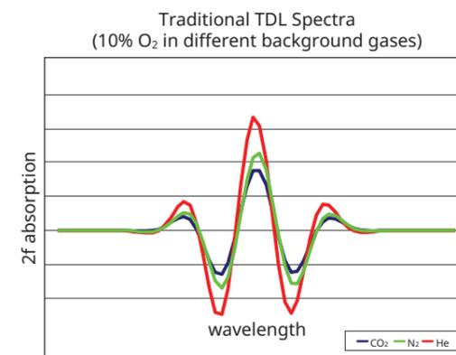
The TruePeak we can measure the area of the absorbance peak. This eliminates effects from changing background gases, allowing for simple pressure and temperature compensation.
