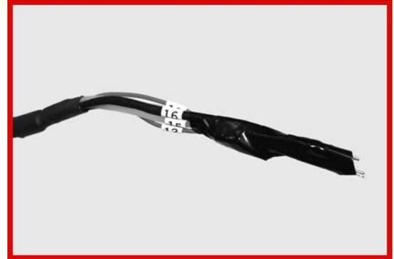
4. Thread the sensor tip onto the ISC40G(S)-GR sensor.
