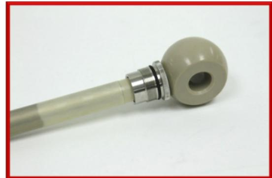
5. Then thread the entire sensor and sensor tip assembly thru and onto the PR10 holder.
