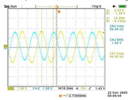
When the frequencies are different, the signals move respective to each other. If the "speed" is low enough, the board may generate a SYNC pulse.
