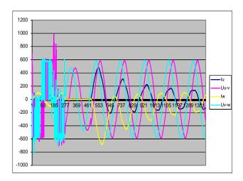
The graph below shows the drive output voltage, network voltage and one phase current.
