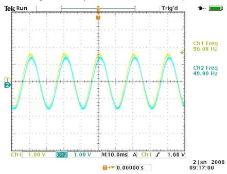
When there is a phase difference, the waveforms are as shown in the graphic below.
