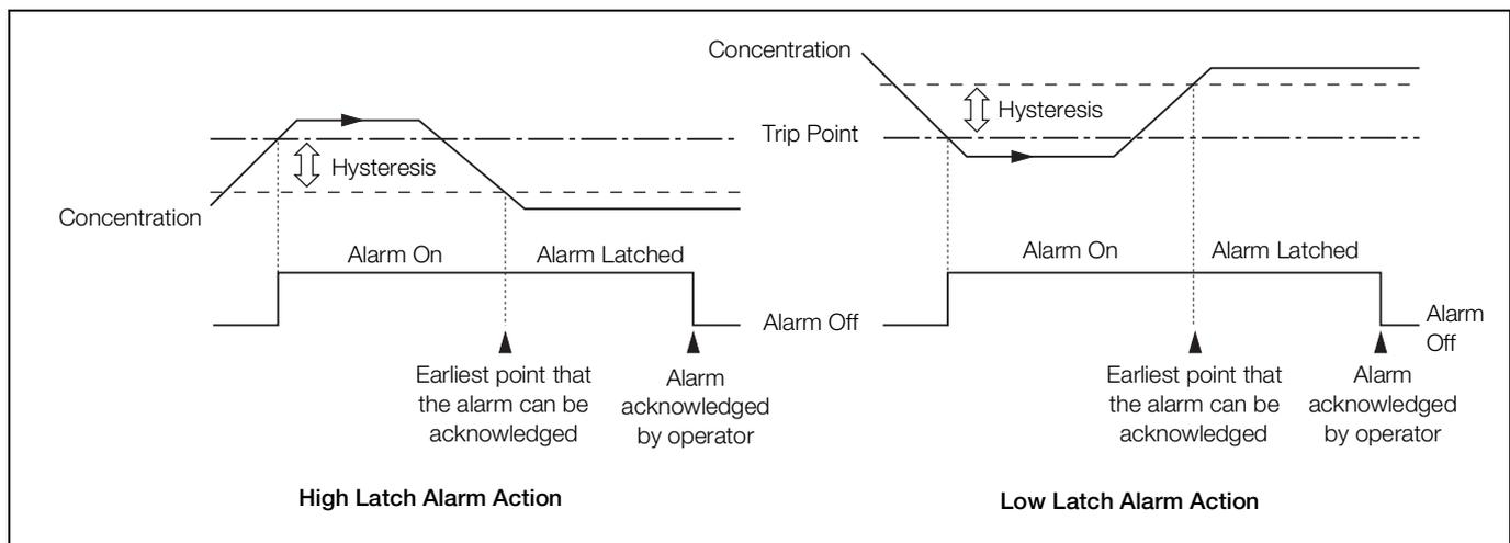
Fig. 6.4 High/Low Latch Alarms
