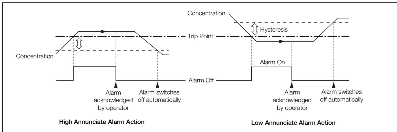
Fig. 6.5 High/Low Annunciate Alarms
