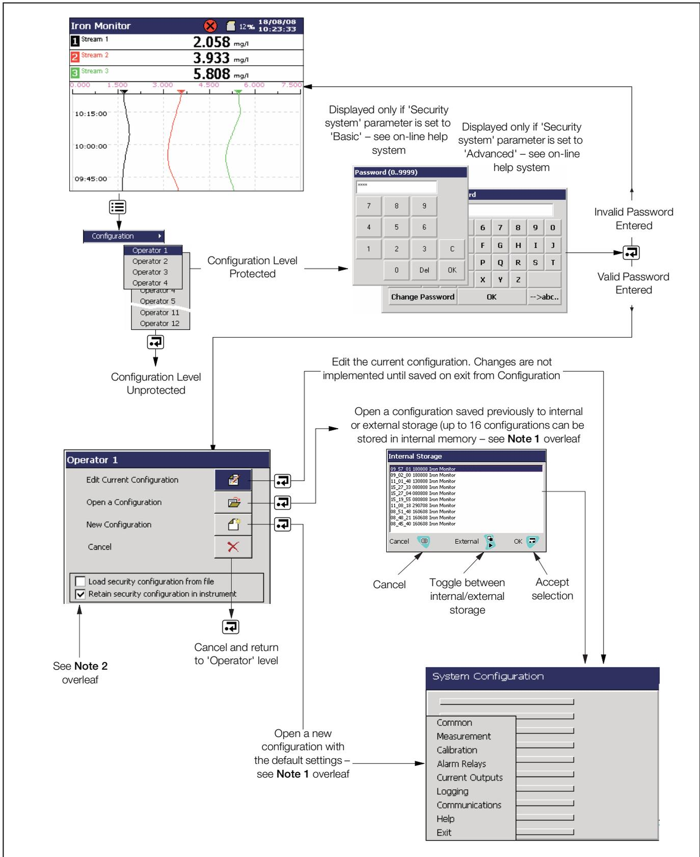
Fig. 6.1 System Configuration
