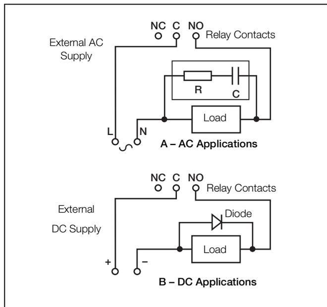
Fig. 4.9 Relay Contact Protection
