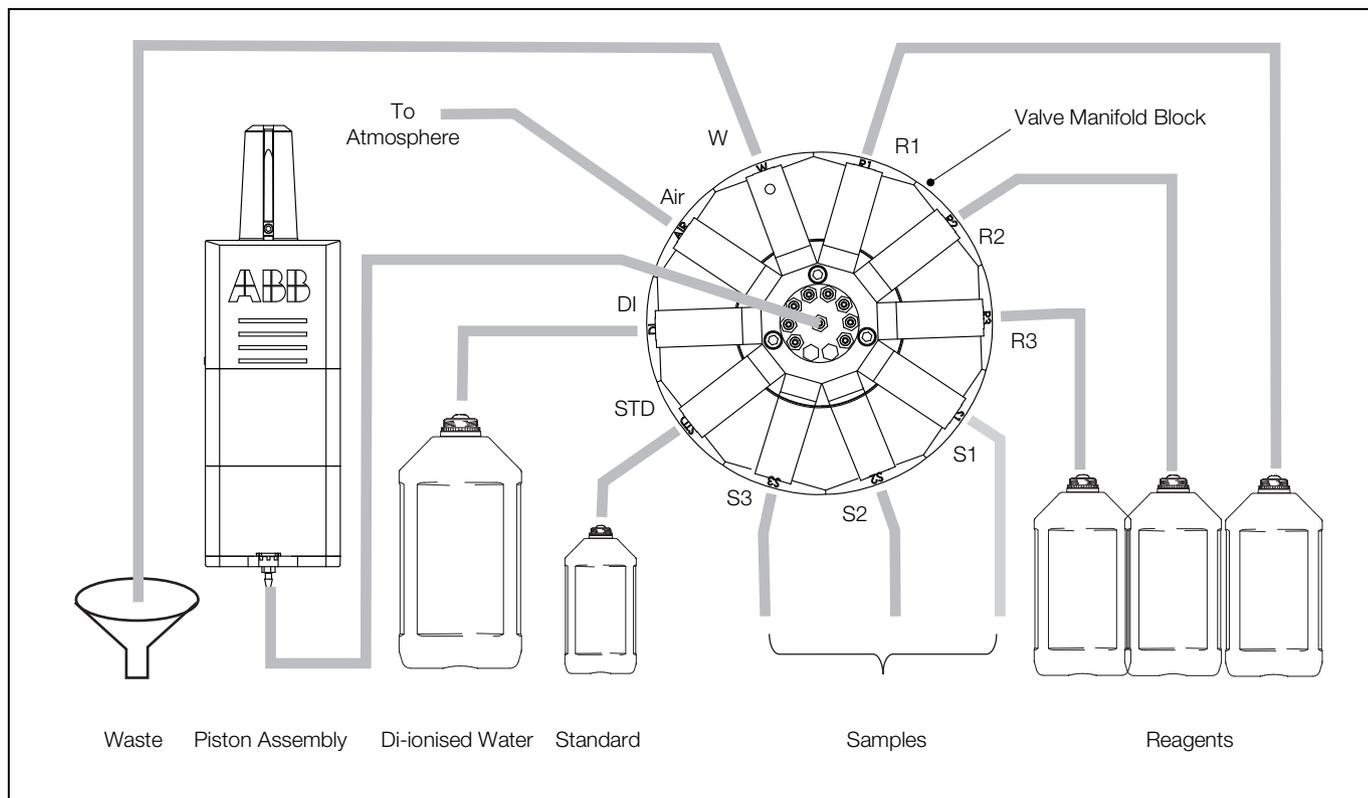
Fig. C.1 Flow Schematic
