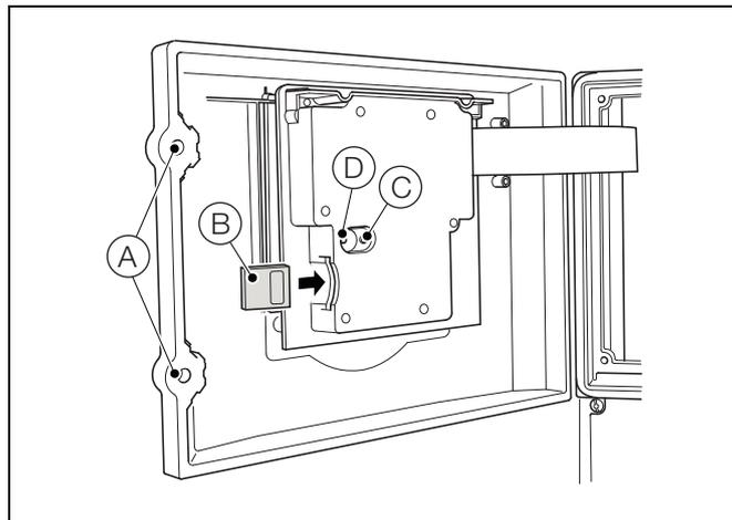
Fig. 7.2 SD Card Removal
