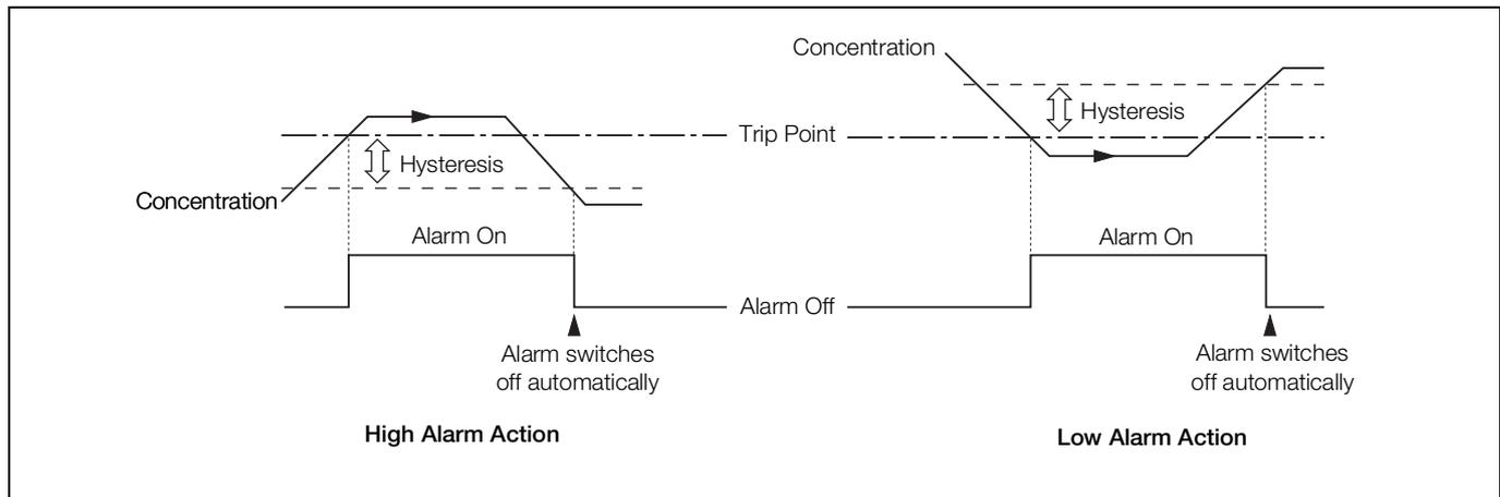
Fig. 6.3 High/Low Process Alarms
