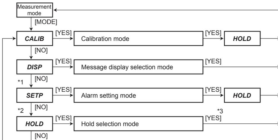
\*1: Skipped if alarm setting function is set to "0: Disabled" in Code 51 at service level, or unless either of functions of contact output S1 or S2 is set to "1: Alarm" in Code 40 or 41 at service level.
