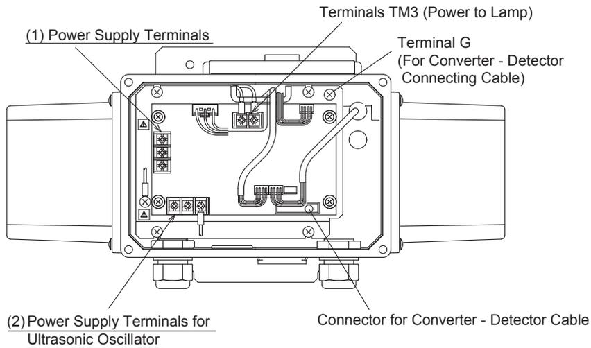
**Figure 2.4 Internal View of Detector**
