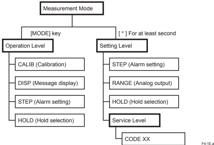
Figure 4.1 Transition between Measurement Mode and Three Levels
