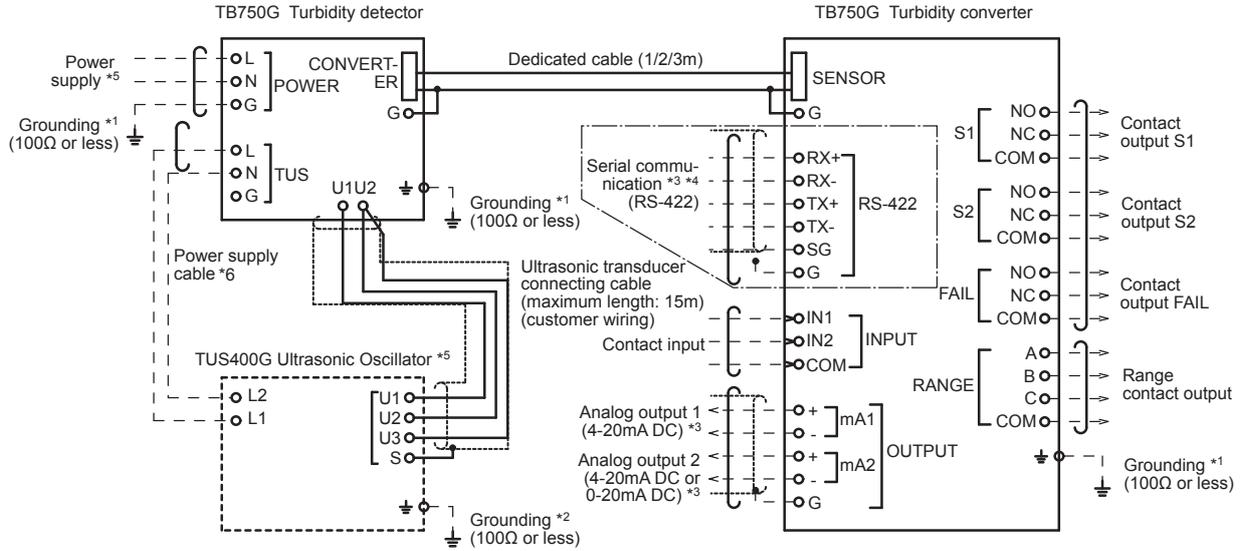
(Note) Dotted wiring is external wiring. Use cable with 6 to 12 mm OD for wiring.
