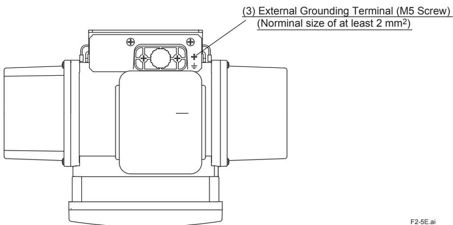
**Figure 2.5 Grounding Terminal of Detector**
