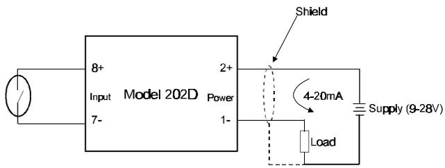
**Connection to a Sensor requiring External Power**
