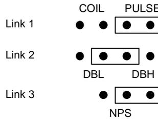
Note: For a switch or reed input with contact bounce link DBH can be switched "on". This will eliminate the effect of switch bounce while limiting the input frequency to 200Hz.
