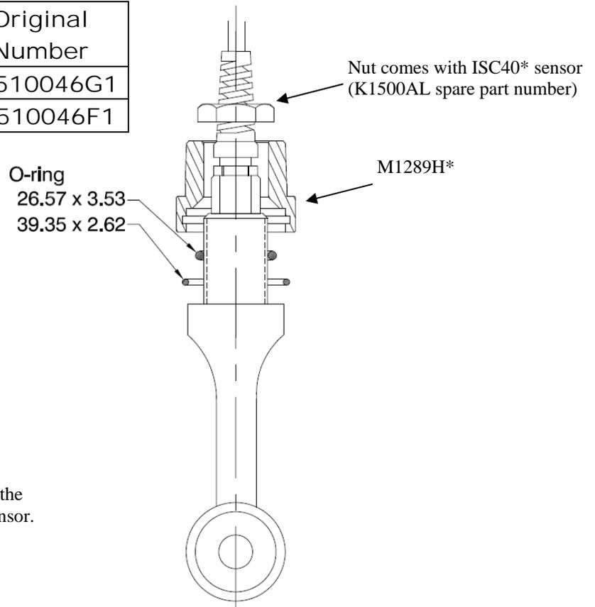
**NOTE:** O-ring Seal is used instead of the Flat Seal provided with the ISC40\* sensor.
