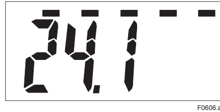
Figure 6.6 Display showing Confirm Connecting Status State
