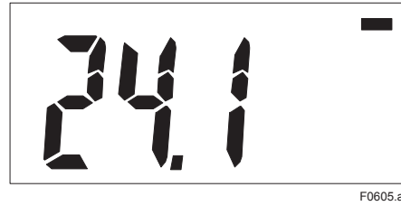
Figure 6.5 Display showing Ready and Pause State
