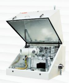
The Liquid Injection System if fully compliant with GPA 2177, as the liquid sample valve is outside the heated zone(GC). The Liquid Injection System comes as a fully integrated package, including the Liquid Inject panel, pilot valves and controller, in an environmental enclosure. Designed for NGL's with dew point below 100°C/212°F.
