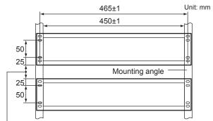
Supplied spacer(50) or Wiring space(30 to 60)
