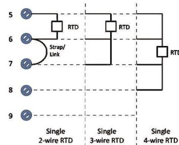
Figure 10: RTD connections
