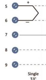
Figure 9: Thermocouple connections
