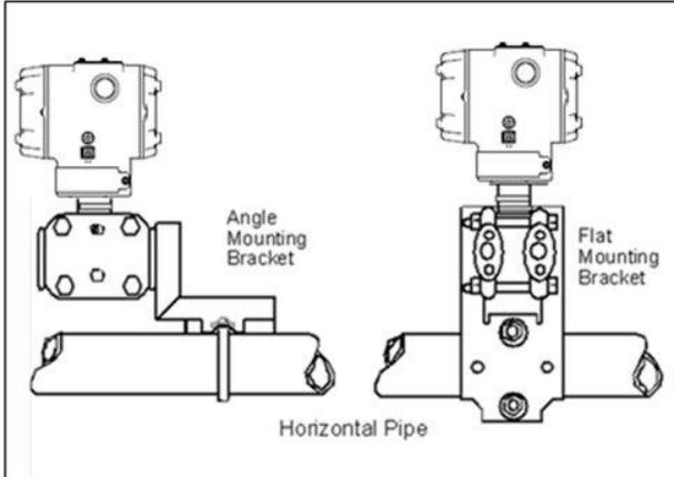
Figure 2: Mounting brackets
