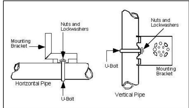
Figure 3: Angle mounting bracket
