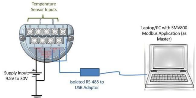
**Figure 12: Transmitter configuration via Modbus (RS-485) network port**
