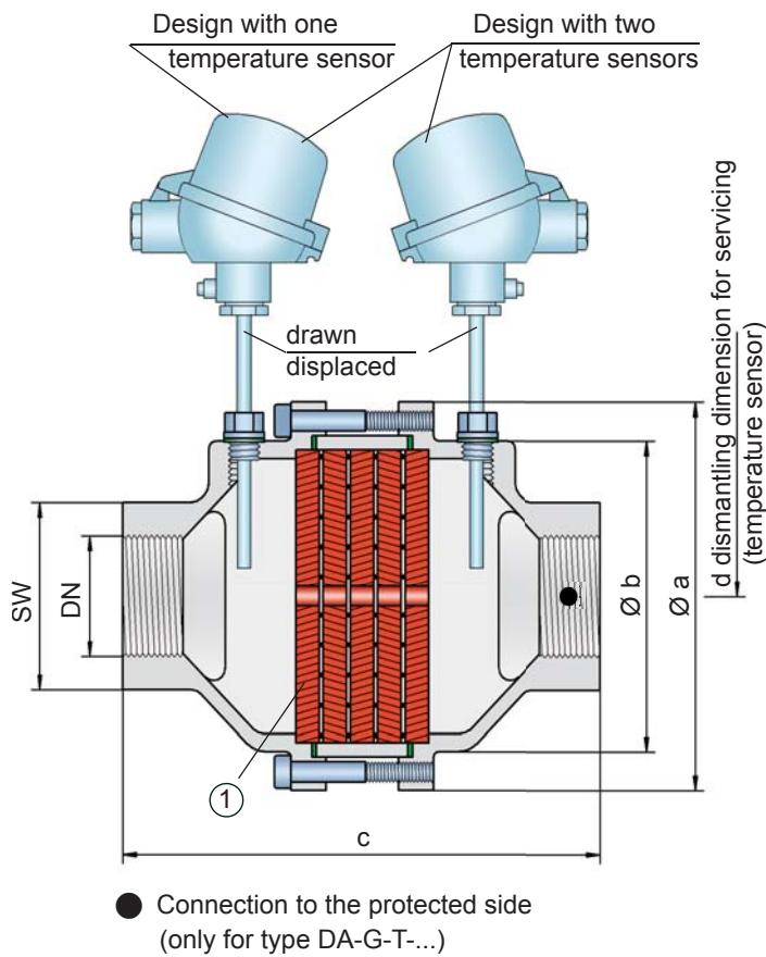
that can be used for all explosion groups, IIA, IIB3 and IIC (NEC Group D, C MESG  $\geq 0.65$  mm and B). The standard design can be used up to an operating temperature of +60°C / 140°F and an absolute operating pressure up to 1.1 bar / 15.9 psi. Devices with special approvals can be obtained for higher pressures (see table 4) and higher temperatures upon request.
